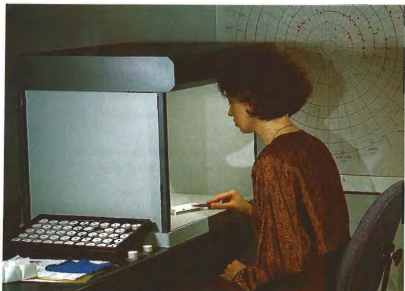
Figure 9. The Judge II box provides a standardized viewing environment, with a neutral gray interior color, controlled lighting, and sufficient working distance for making consistent color comparisons of colored diamonds. Photo by R. Weldon.
