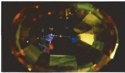
Figure 10. Purple iridescence on the pavilion of this medium-dark 0.98-ct yellowish orange sapphire suggests that it has been coated.
