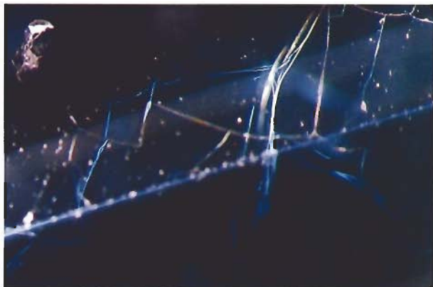
Figure 18. Violetish blue dispersive flashes, as shown here in an amethyst, are believed to be the most characteristic feature of Opticon-filled fractures in quartz gems. Photomicrograph by John I. Koivula.
