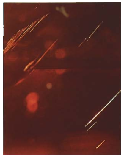
Figure 14. The presence of what appeared to be boehmite needles together with repeated twinning also created problems in the client's identification of this 26.00 × 13.12 × 9.20 mm reddish orange sapphire. Magnified 23×.
