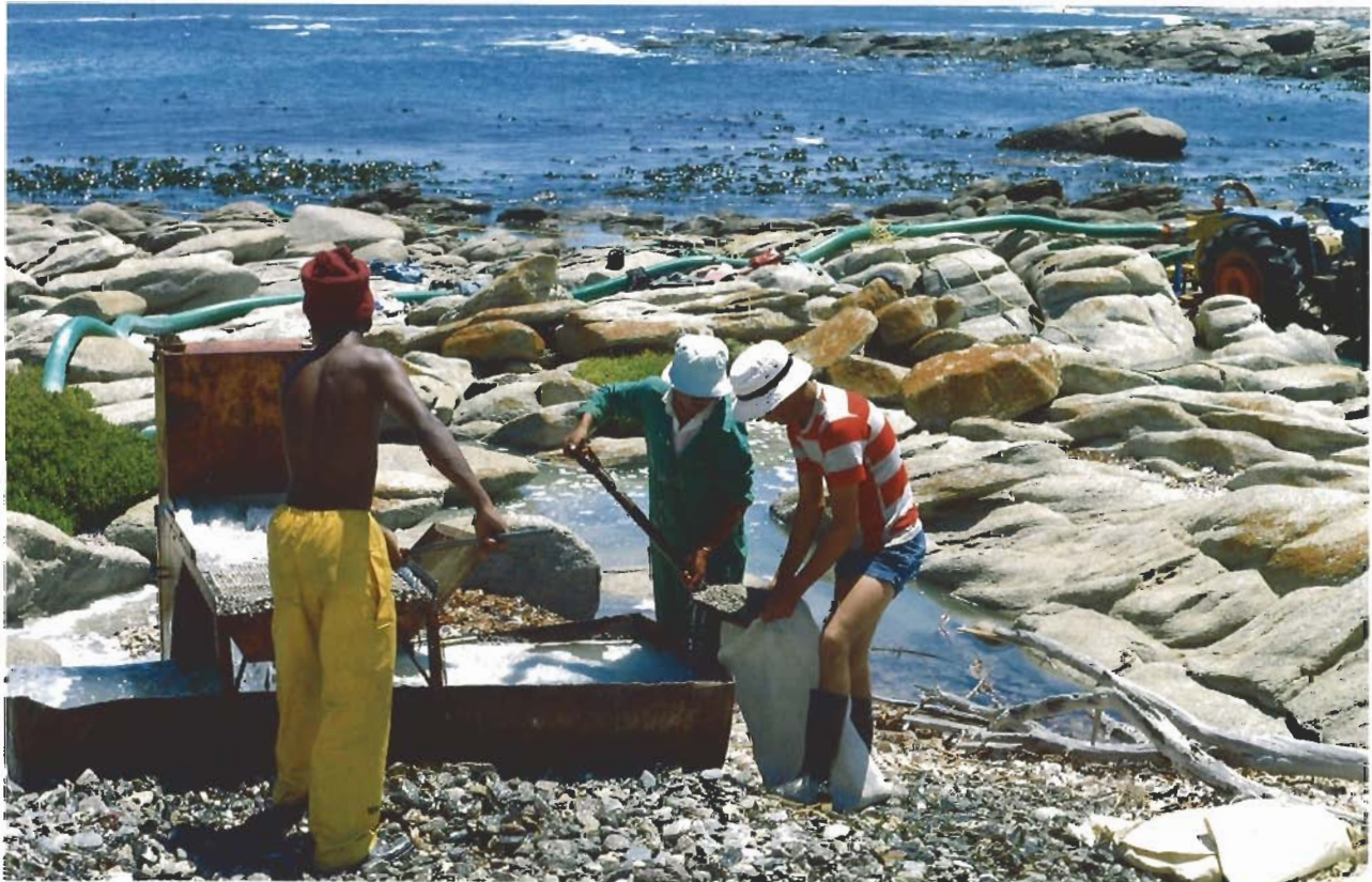
Figure 14. The other end of the suction apparatus illustrated in figure 13 is frequently mounted on a tractor (which supplies the power) that is located nearby (here, far upper right) together with a sieving operation. The sack in the foreground contains diamond-bearing material that has been screened to eliminate the coarse gravel. This "sieved material" will be taken to a diamond-recovery plant for further processing.
