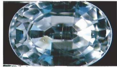
Figure 12. With additional soaking in HCl heated to a low temperature, the "yellowish orange" sapphire became completely colorless.
