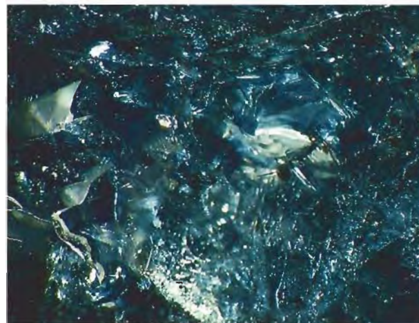
Figure 6. Numerous minute black inclusions lining cleavages and fractures were responsible for the almost opaque nature of the black diamonds. Photomicrograph by Robert E. Kane; oblique illumination, magnified 20 \times .
