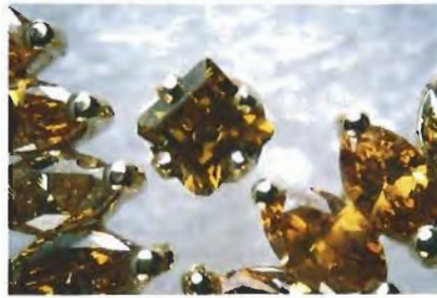
Figure 4. The similarity in appearance between a Sumitomo synthetic yellow diamond (here, the 0.19-ct stone in the center) and the natural fancy yellow diamonds in the brooch shown in figure 3 is striking. The stone at the lower left is one of the two that fluoresced to short-wave U.V. radiation.
