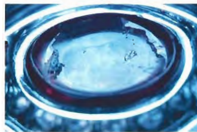
Figure 13. The synthetic ruby in the pin shown in figure 12 has a glass-filled cavity. Magnified 15 \times .
