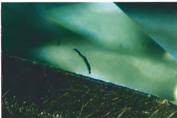
Figure 12. At first glance, this appears to be a normal radiation "stain" (evidence of radiation damage) on the surface of an upper girdle facet of the Dresden Green diamond. Photomicrograph by Robert E. Kane; magnified 25 \times .
