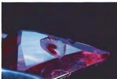
Figure 11. A glass-filled cavity is readily apparent in this 1.12-ct faceted ruby, which showed no other evidence of heat treatment. Magnified 15 \times .
