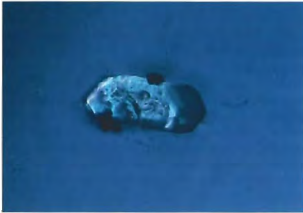
Figure 14. The Kashmir samples examined commonly contained small, slightly corroded crystals with indentations that match earlier descriptions of zircon. The smaller, black, cube-like crystals shown here on a zircon-like crystal in a Kashmir sapphire appear to be uraninite. Photomicrograph © Rolf Schwieger; magnified 200×.
