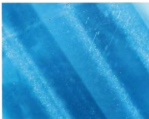
Figure 6. Even at 40× magnification, with the strong illumination provided by a powerful fiber-optic light source, the tiny particles that contribute to the haziness of the milky layers can be seen in some Kashmir sapphires. Photomicrograph © Rolf Schwieger.
