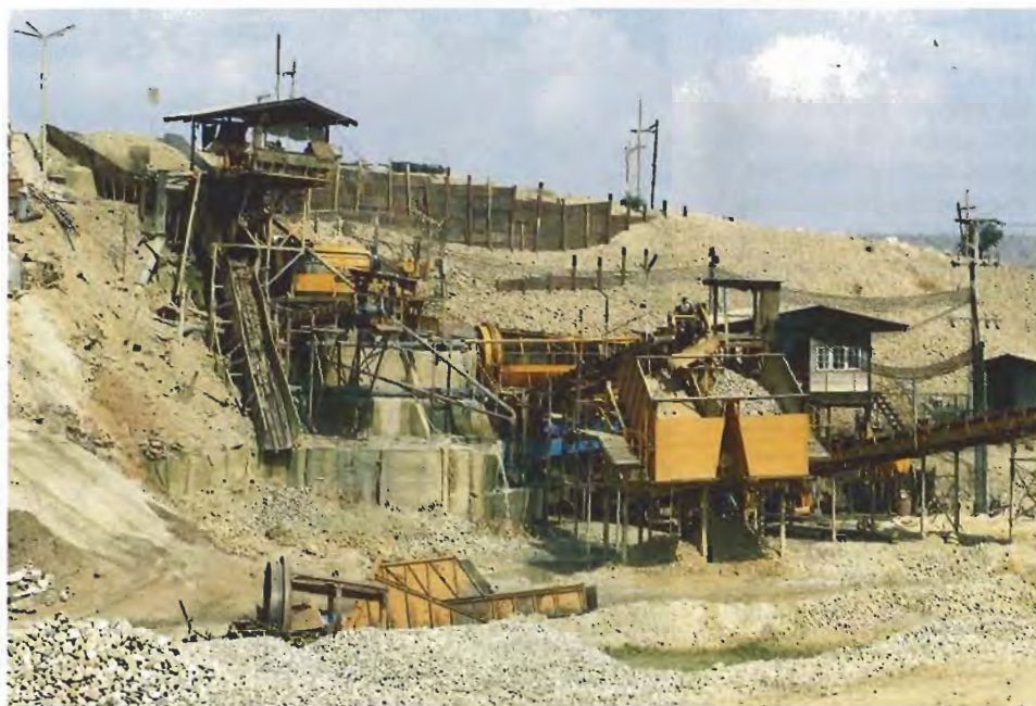
Figure 4. Modern, large-capacity equipment is used by S.A.P. Mining Co. to process the gemiferous gravels it mines near Bo Phloi in the Kanchanaburi district. Photo by Robert C. Kammerling.
