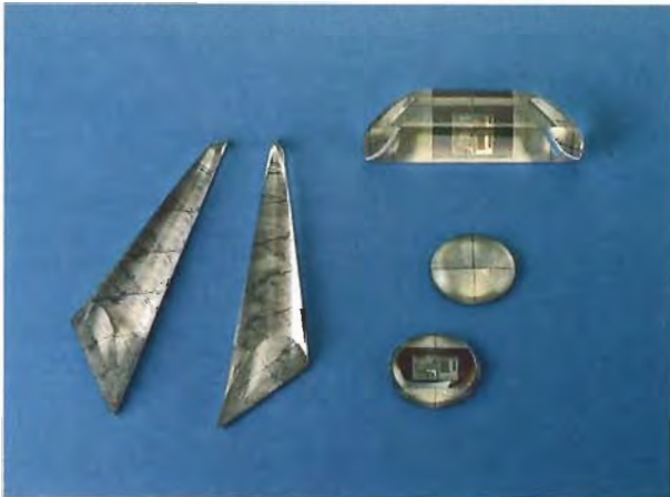
Figure 2. These novel assembled stones have been constructed from silicon chips and quartz. Photo by Robert Weldon.
