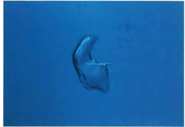
Figure 15. More than half of the Kashmir sapphires studied were found to contain strongly corroded crystals of what appear to be plagioclase. Photomicrograph © Rolf Schwieger; magnified 63×.
