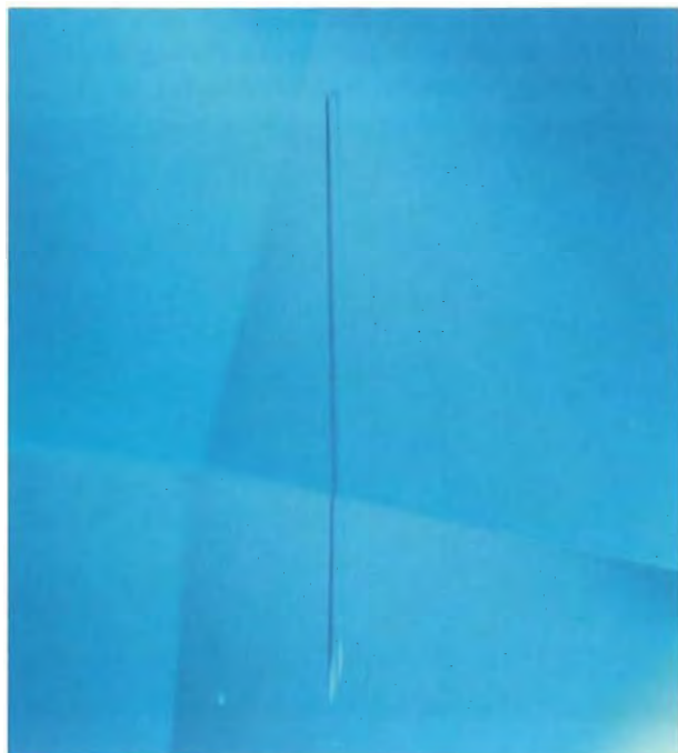
Figure 11. Long, thin, needle-like crystals of pargasite were observed in about 10% of the stones examined for this study. Pargasite has not been reported in sapphires from other localities. Photomicrograph © Rolf Schwieger; magnified 40×.
