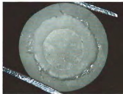
Figure 5. There appears to be a "melted" indentation on the crown of this 0.88-ct burned diamond. Magnified 20\times .
