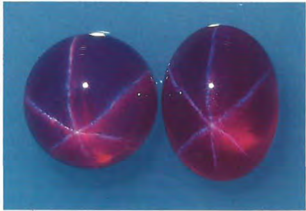
Figure 1. Shown here are the largest round (1.99 ct) and oval (1.60 ct) cabochons of Kyocera synthetic star ruby studied for this report. Note the near-transparency and slightly imperfect stars.
