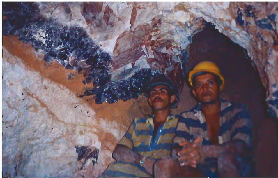
Figure 4. Veins of amethyst line the walls of this tunnel at Alto Bonito. Because the air is so thin, the miners operate in groups of three, with one man working while the other two rest.
