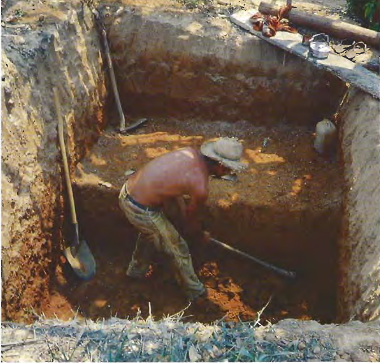
Figure 8. Picks and shovels are used at Pau d'Arco to remove the various layers of dirt and gravel that cover the amethyst-producing layer. The pits average 4 m wide \times 7 m long, and usually reach 2–3 m deep.
