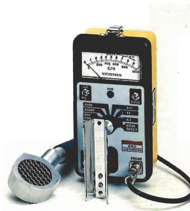
Figure 11. The most common, and least expensive, radiation detector is a Geiger counter such as this Victoreen Model 290 Survey Meter with a Model 489 pancake probe. Photo courtesy of Victoreen, Inc., Cleveland, OH.
