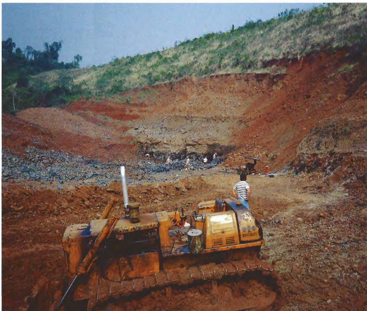
Figure 14. At Iraí in Rio Grande do Sul, a tractor is used to remove much of the hill in which the amethyst-bearing basalt layer is found, 30 m below the original surface.
