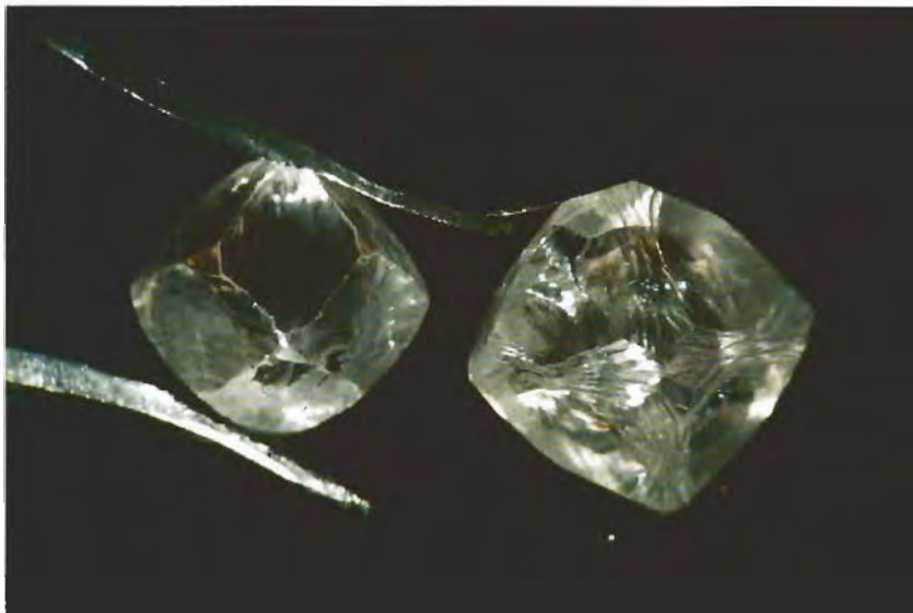
Figure 2. Cubic zirconia has been very cleverly fashioned to imitate rough diamond crystals. These two samples measure 10.21 \times 7.88 \times 7.38 mm and 8.50 \times 7.30 \times 6.96 mm, respectively, with a total weight of 15.19 ct. Magnified 10\times .
