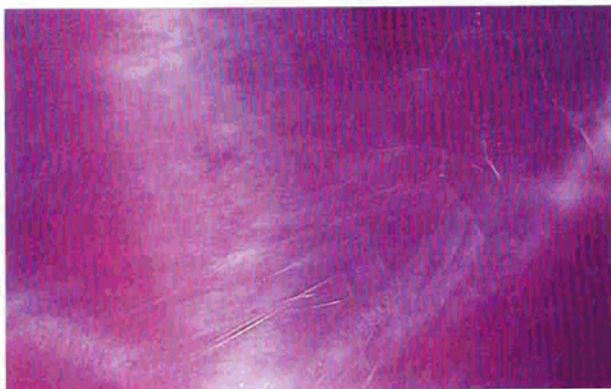
Figure 4. Present in all five specimens examined, these white smoke-like patterns, together with the fineness of the asterism-causing needles, provide proof of synthesis. Darkfield and oblique fiber-optic illumination; magnified 50 \times .
