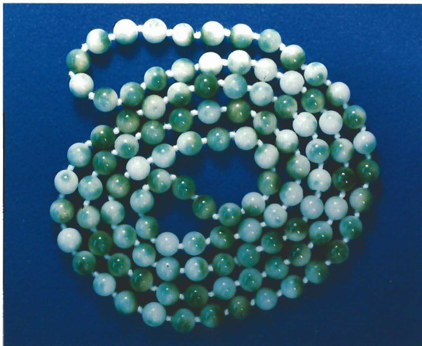
Figure 6. These 8-mm quartzite beads were selectively dyed to simulate the appearance of "moss-in-snow" jadeite.
