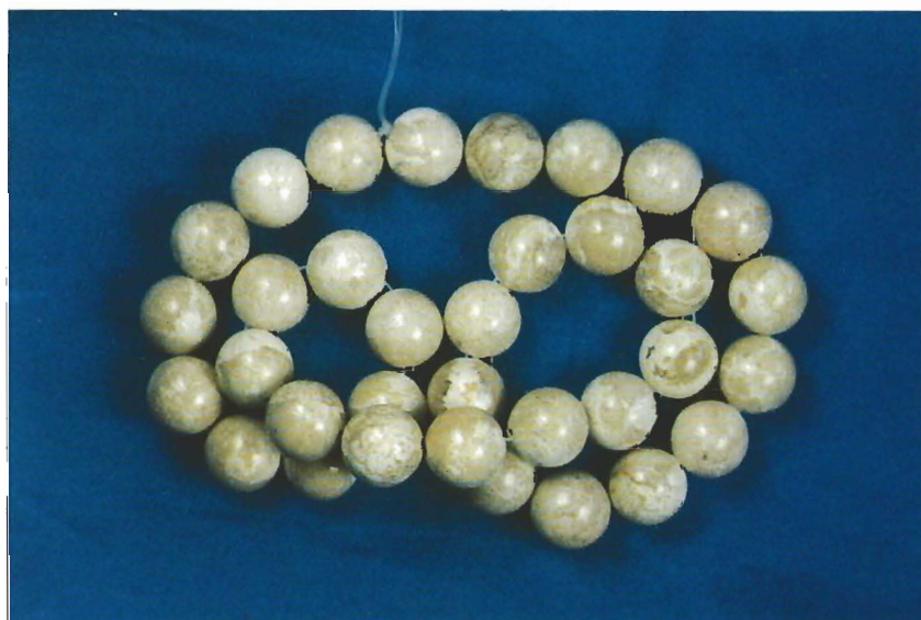
Figure 3. These 12–12 1/2-mm beads, sold as "Riverstone," are actually a type of calcium carbonate.
