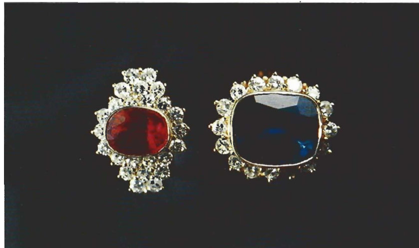
Figure 4. These attractive cocktail rings contain corundum doublets that consist of synthetic ruby and synthetic sapphire pavilions with natural sapphire crowns.
