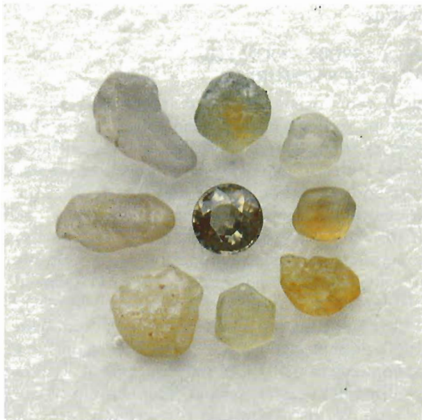
Figure 3. Examples of the range of colors of types 1, 2, and 3 pale tan and brown sapphires studied; the largest piece is 6 mm long.
