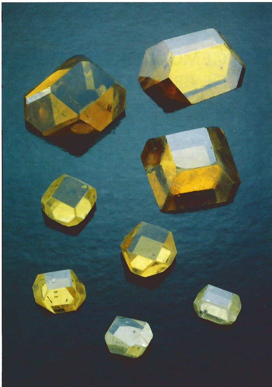
Figure 1. These eight gem-quality synthetic diamond crystals (0.40–5.23 ct) were manufactured on an experimental basis at the De Beers Diamond Research Laboratory and loaned to GIA for study. They fall into three distinct color groups: dark brownish yellow, yellow, and light greenish yellow. Photo © Tino Hammid.
