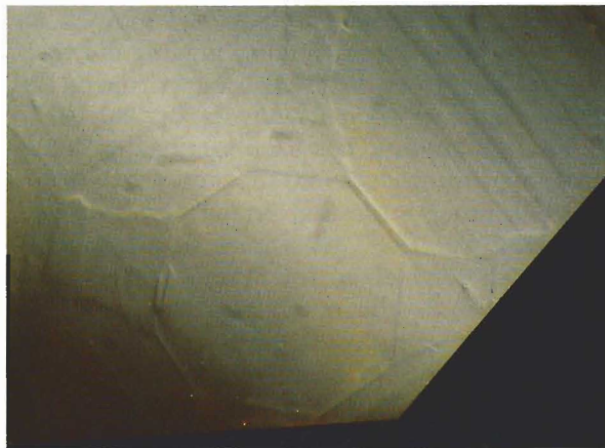
Figure 22. An octagonal “stop sign” pattern of surface graining is also visible on the polished table of the synthetic diamond shown in figure 21. Near the lower right-hand edge of the table, the central cubic-sector core of the crystal is recognizable from its octagon-shaped outline. Four narrow octahedral growth sectors extend outward from the core at right angles to one another. Also visible are the four cubic growth sectors with their parallel surface grain lines. Oblique illumination; magnified 30×.
