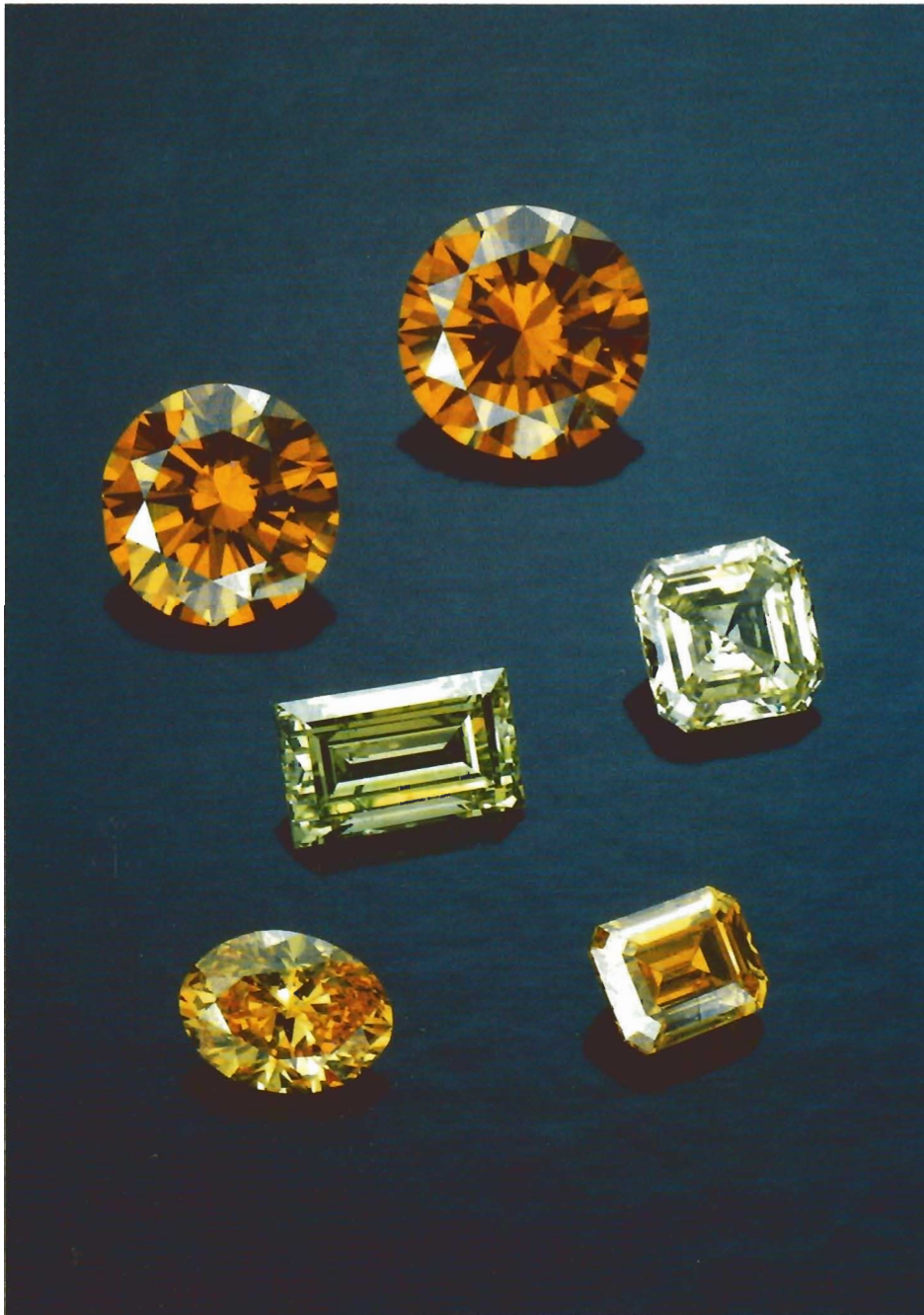
Figure 2. These six faceted De Beers synthetic diamonds (0.27–0.90 ct) were also examined for this study. They include the largest faceted synthetic diamonds that have ever been examined at GIA. Photo © Tino Hammid.
