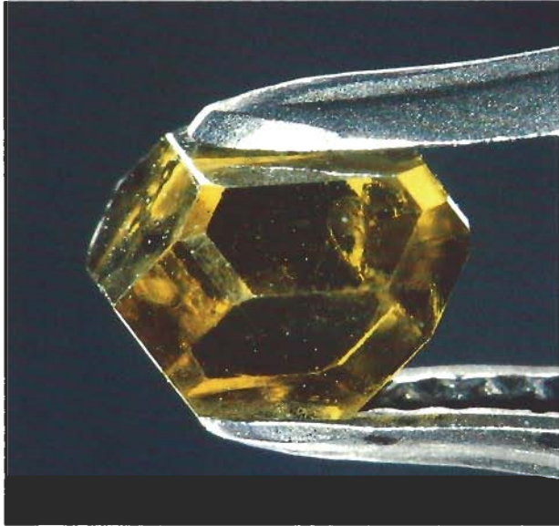
Figure 2. This close-up view of a Sumitomo synthetic diamond crystal illustrates the appearance of the crystal, the arrangement of the crystal faces, and the nature of the outer surface of the crystal. The crystal weighs 1.07 ct. Photo by John Koivula.
