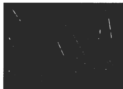
Figure 4. These spicules are the closest counterparts to the nailhead spicules typical of hydrothermal synthetic emerald that the lab has seen thus far in a synthetic amethyst. Magnified 20x.
