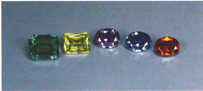
Figure 8. This 11.66-ct imitation emerald and the other variously colored stones are synthetic spinel triplets that use sintered colored glass instead of cement. The drawing shows the construction of these triplets.
