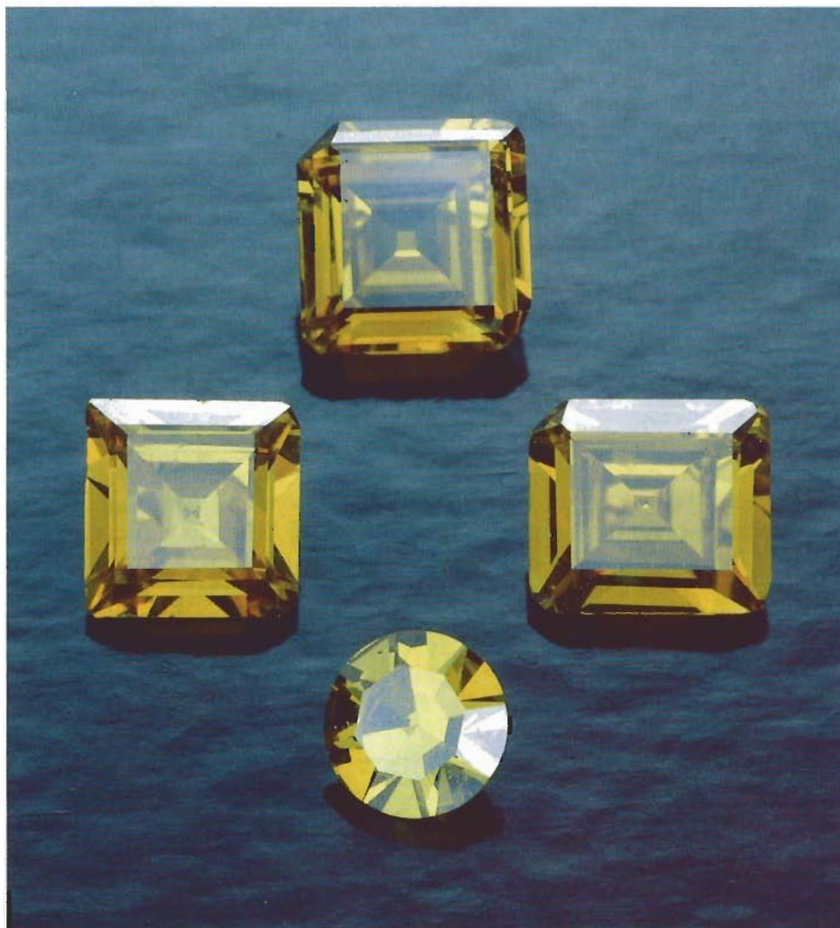
Figure 19. Four of the synthetic diamonds that we had faceted from the rectangular pieces of the material. The round single cut weighs 0.08 ct and measures 2.80 \times 2.80 \times 1.69 mm. The step-cut faceted pieces weigh between 0.16 and 0.24 ct and measure between 3.48 and 3.84 mm in maximum dimension. Photo © Tino Hammid.
