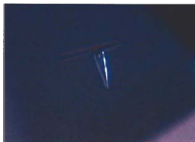
Figure 3. This spicule with quartz crystal cap seen in a synthetic amethyst closely resembles an inclusion seen in the hydrothermally grown Biron synthetic emerald, which appears on page 164 of the Fall 1985 issue of Gems & Gemology . Magnified 45x.
