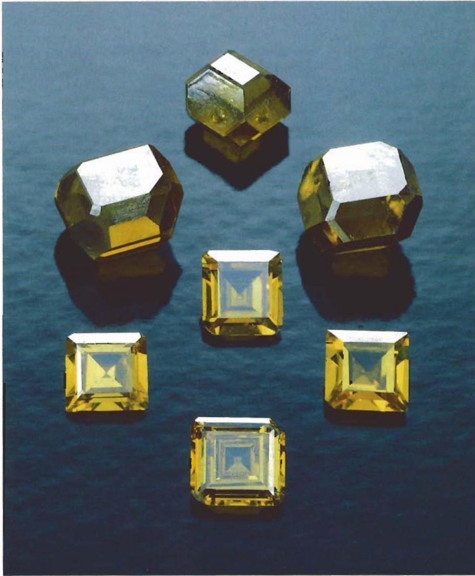
Figure 1. Three synthetic yellow diamond crystals manufactured by Sumitomo Electric Industries along with four of the synthetic yellow diamonds that we had faceted. The crystals (left to right) weigh 1.05, 0.63, and 1.07 ct, and measure 5.5, 4.7, and 5.3 mm in maximum dimension. The crystals can be described as distorted octahedral shapes that are modified by large cube crystal faces on the top and bottom and by smaller dodecahedral crystal faces around the edges. The four faceted stones were cut from the rectangular pieces of synthetic diamond (the form in which it is currently sold for use as heat sinks) in such a fashion as to retain maximum weight. The faceted stones weigh between 0.16 and 0.24 ct, and measure between 3.48 to 3.84 mm in maximum dimension. Photo © Tino Hammid.
