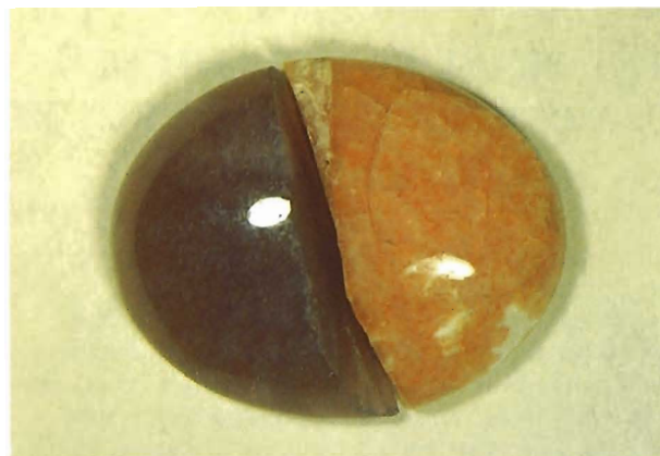
Figure 7. Deep purple amethystine chalcedony cabochon before (left) and after (right) heat treatment to 550°C. Photo by John Koivula.
