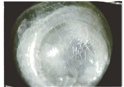
Figure 14. The surface of the imitation pearl shown in figures 12 and 13 was crazed when the bead was immersed in safety film cleaner. Magnified 10x.
