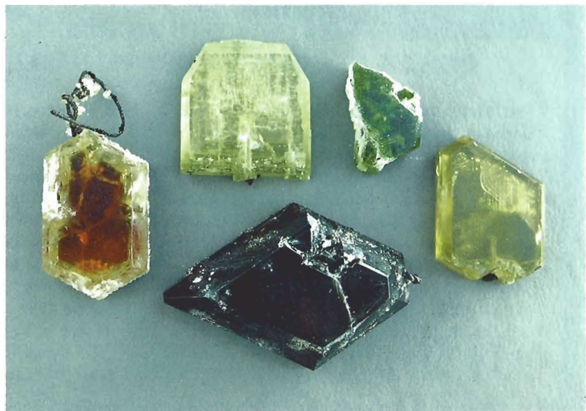
Figure 16. The various colors of this hydrothermally grown synthetic zincite are caused by the use of different impurities. The large black specimen is 43 mm long and weighs 52.1 grams.
