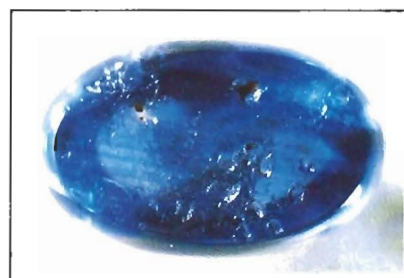
Figure 2. The craters in the base of the sapphire shown in figure 1 prove that this stone was heat treated rather than diffusion treated. Magnified 12x.
