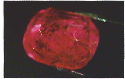
Figure 18. Note the dark inclusions in the "Geneva (synthetic) Ruby" illustrated in figure 17. Magnified 18x.
