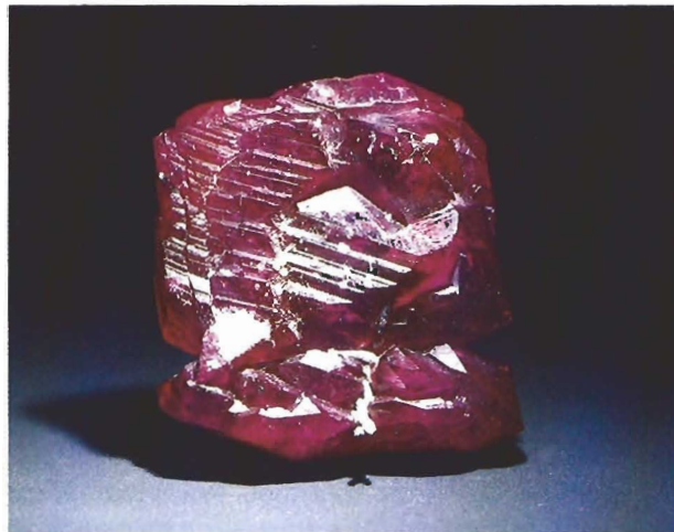
Figure 6. Verneuil synthetic ruby slab after flux regrowth for 42 days ( 20.7 \times 16.8 \times 7.6 mm). Note the platinum wire at the base. Photo by Mike Havstad.
