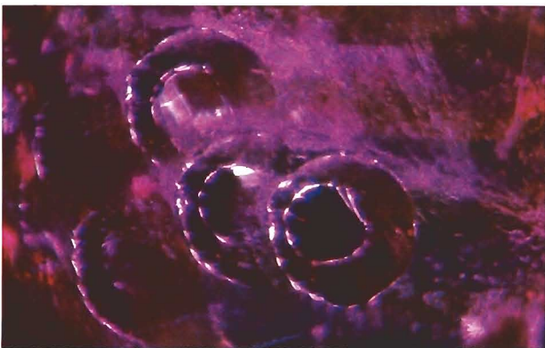
Figure 9. Typical inclusions in Thai ruby are these circular features surrounding pyrrhotite. Magnified 60×. Photo by John Koivula.
