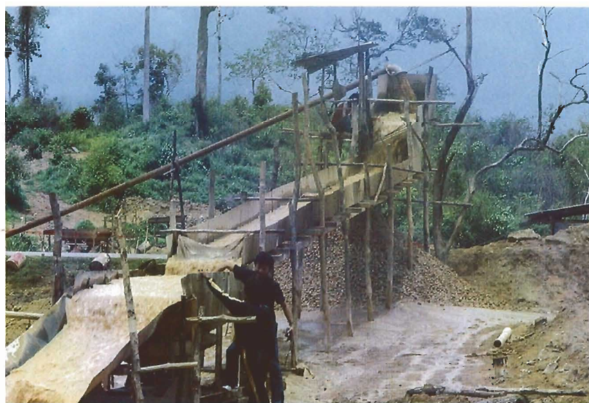
Figure 5. After the gem gravels exit the pipe, they are run over a long sluice. The heavier corundum concentrate collects in a jig at the end.
