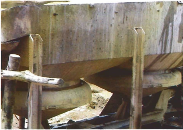
Figure 6. A jig or "willoughby" table washer, a device borrowed from the Phuket tin mines on the southern extension of Thailand, is very effective at concentrating ruby.
