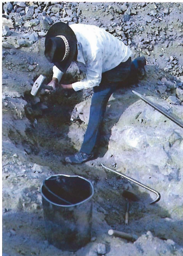
Figure 3. An Apache miner uses a chisel and sledge hammer to work a hand-dug peridot pit in the hard basalt.
