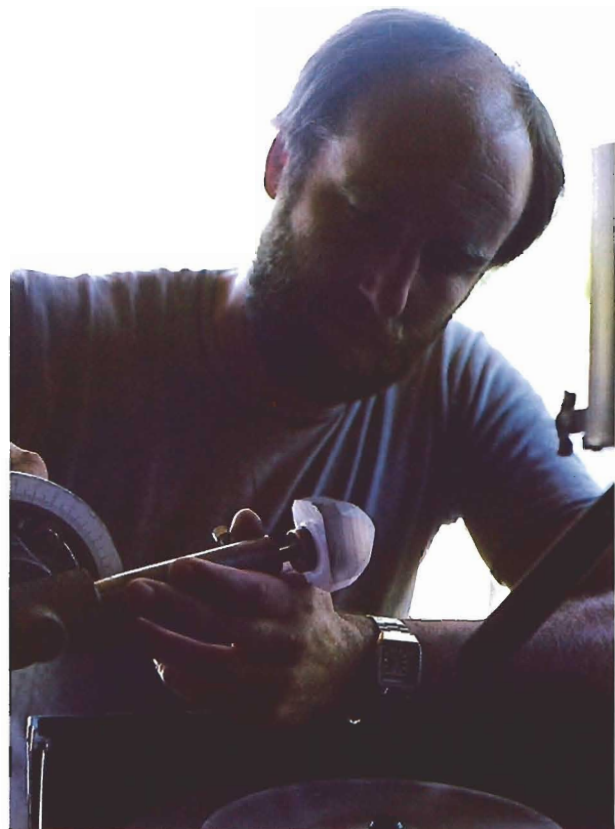
Figure 4. Carleton faceting the kunzite. This custom-made faceting machine, a second-generation design by Bryant Harris of Fallbrook, California, is big enough to cut the world's largest faceted stone.
