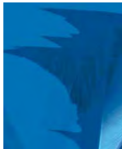
Figure 3. This DiamondView image of the pavilion of the pear shape clearly shows the different type zones: moderate blue fluorescence for the type IIa region, and weak blue for the IIb zone.
