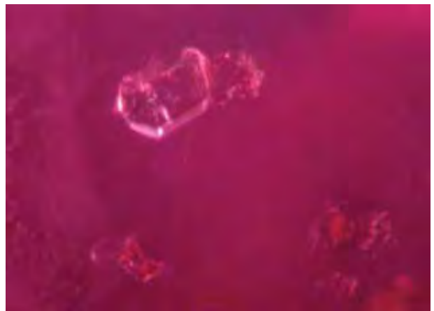
Figure 29. Colorless transparent apatite crystals were seen in only two Winza rubies. Photomicrograph by V. Pardieu/GGL; magnified 40×.
