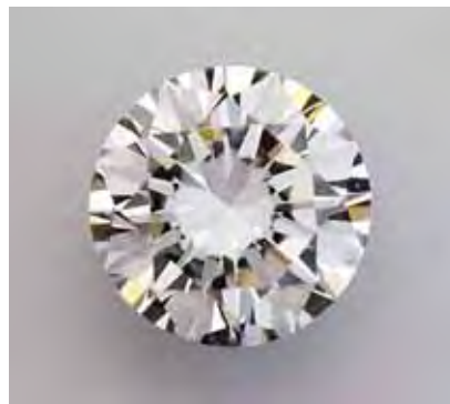
Figure 5. This 0.21 ct CVD synthetic diamond was found to be HPHT treated.
