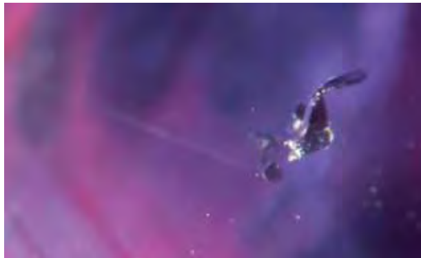
Figure 31. A group of mineral inclusions (probably amphibole) is accompanied by a weakly developed "comet tail" in this Winza sapphire. Note also the pink-blue color zoning and (slightly diffuse) fine light blue growth bands. Photomicrograph by V. Pardieu/GGL; magnified 40 \times , fiber-optic illumination.
