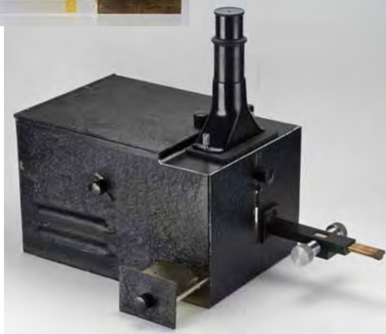
Figure 3. The GIA Colorimeter, introduced in 1941, was developed to select master stones by visually comparing a diamond to a repeatable standard called the “color yardstick” (inset, top)—a graduated wedge of glass that transitioned from colorless to yellow. When a diamond being graded matched a section of the wedge in the colorimeter, the corresponding Roman numeral expressed the grade. Lighting, viewing geometry, and the comparison standards were all controlled with this box. Although modified over time, these three factors continue to be at the heart of consistent color grading. Photos by Robert Weldon.
