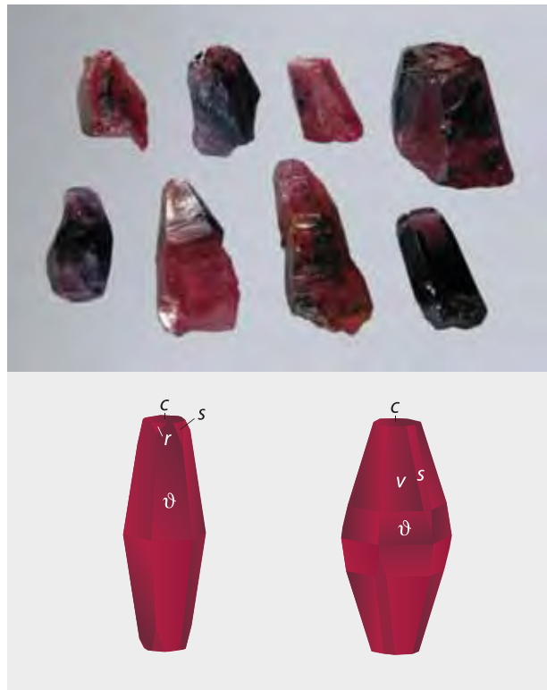
Figure 13. The dipyramidal Winza ruby and sapphire crystals, such as those shown here (lower right is 7 \times 13 mm), are dominated by \vartheta faces, which are accompanied by various combinations of c , r , s , \nu , and n faces. Photo by K. Schmetzer.
