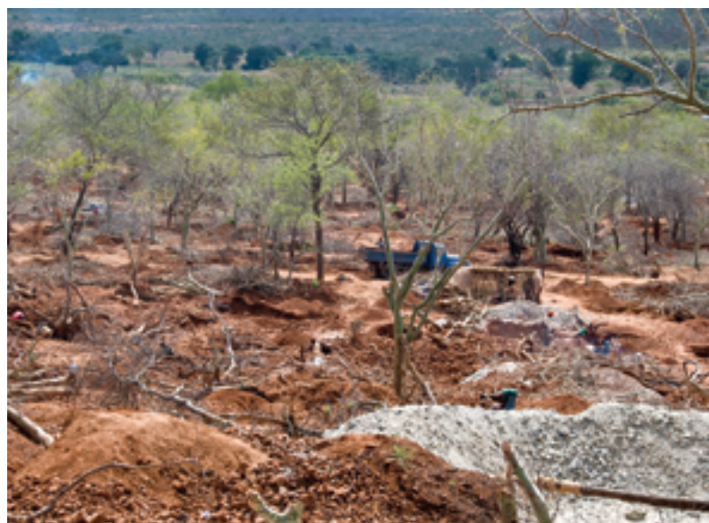
Figure 4. The eluvial and primary deposits at Winza (both shown here) have been mined by hand methods, and the gem-bearing material is then carried to the Mtindiri River for washing. This is typically done by hand, but a truck was also in use at the time this photo was taken in May 2008. Photo by B. M. Laurs.
