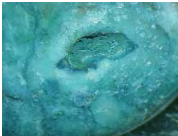
Figure 28. Microscopic examination of the dyed chalcedony shows a greenish blue dye concentrated in fractures and cavities. Photomicrograph by N. Ahmed, © Dubai Gemstone Laboratory; magnified 20x.
