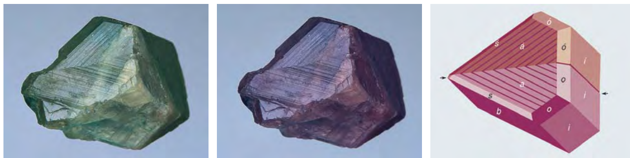
Figure 2. Alexandrite from the Mananjary area shows a distinct color change, from bluish green in day or fluorescent light (left) to reddish or grayish purple in incandescent light (right), as seen in this 70.74 ct specimen. The crystal is twinned by reflection across the prism {031} and reveals the striations characteristic of chrysoberyl on the a and a' {100} faces of the twin. Photo by Maha Tannous; color corrected to show appearance in fluorescent light. The crystal drawing indicates the faces present on this thick columnar twin; the location of the twin boundary is shown by arrows.
