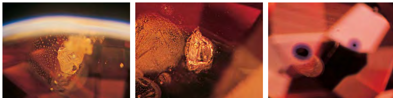
Figure 3. The new Be-diffusion process exposes corundum to such high temperatures that extreme changes occur in the inclusions, such as: (left) partial recrystallization of melted inclusions, (center) completely melted inclusions that contain gas bubbles, and (right) large spherical blue halos around rutile crystals. Photomicrographs by Shane F. McClure (left and center, magnified 40 \times ) and John I. Koivula (right, magnified 25 \times ).
