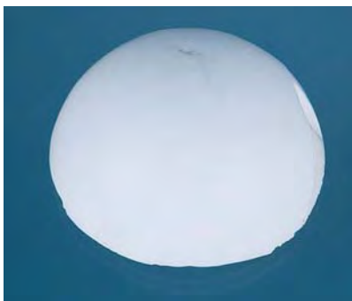
Figure 4. Represented as a pearl, this 20 mm opaque white "cabochon" was identified as a molded form of ceramic.
