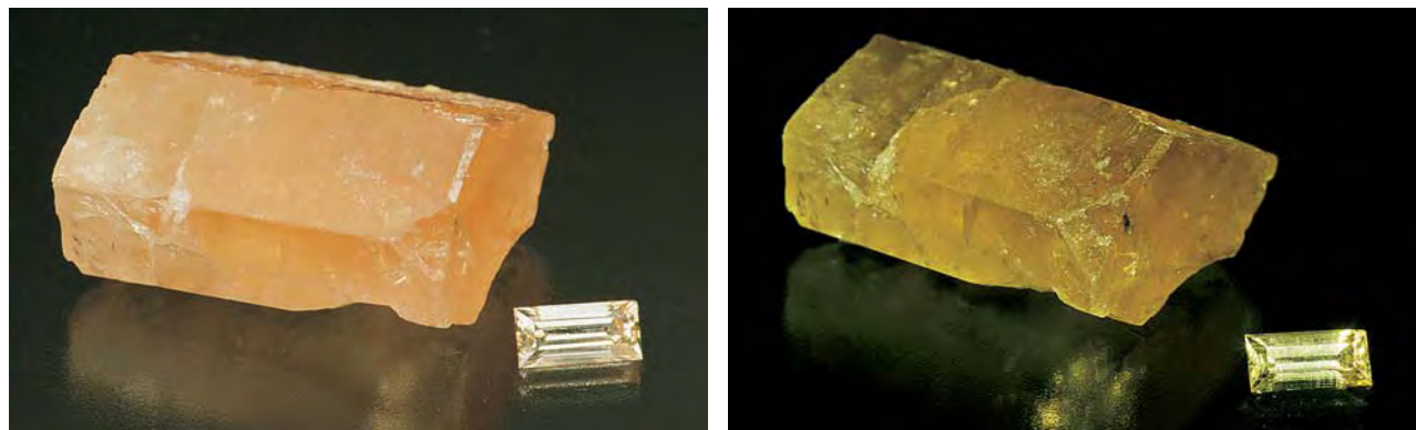
Figure 3. Gem-quality color-change apatite was recently produced from a pegmatite in Kazakhstan. The 3.5-cm-long crystal and 2.37 ct faceted stone shown here are pinkish orange in incandescent light (left) and greenish yellow in fluorescent light (right). Photos by Jaroslav Hyrsl.
