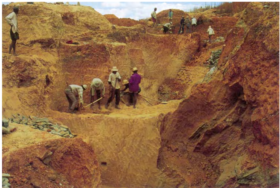
Figure 5. At Antsongombato, gem-quality rhodizite-londonite was mined from a rather narrow (up to 60 cm thick) pegmatite dike by simple hand-digging. A portion of the pegmatite is visible as the steeply dipping dike in the right foreground. Photo by Federico Pezzotta, April 1999.
