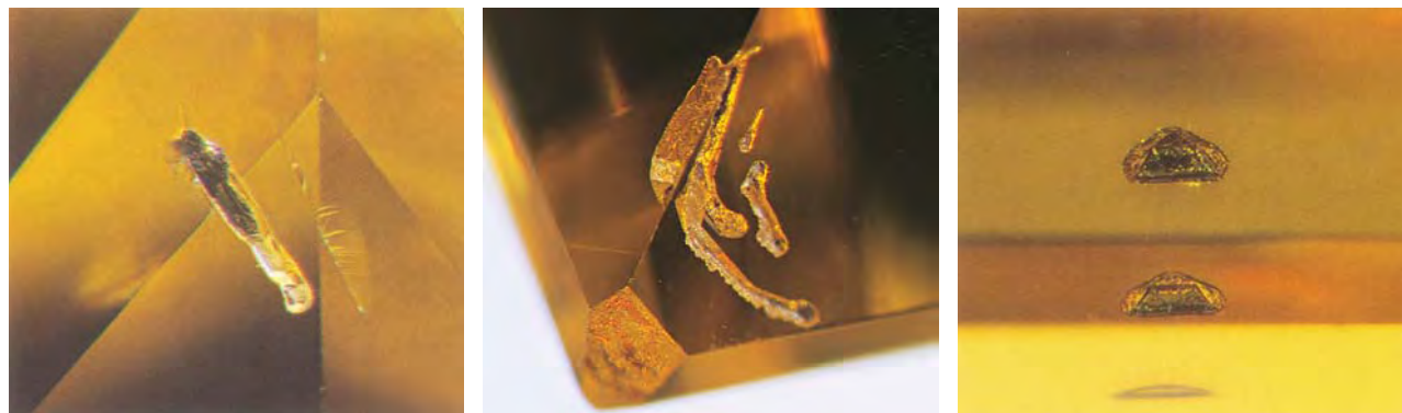
Figure 5. Small metallic inclusions were observed in 10 of the 30 Gemesis laboratory-grown diamonds, three of which are illustrated here. Note in the center image that a small area also shows part of the original crystal surface. The metallic inclusion on the right, seen in direct view and by reflection in two facets, has an equant shape with flat surfaces. Photomicrographs by James Shigley; magnified 75 \times .
