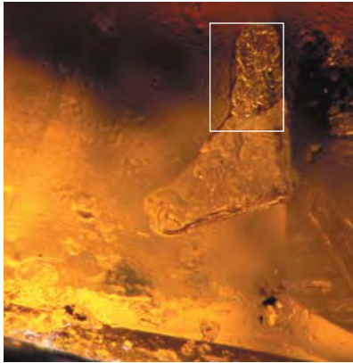
Figure 9. Microscopic examination (at 45×) of the sapphire in figure 8 revealed tabular crystal regrowth after extreme heating.
