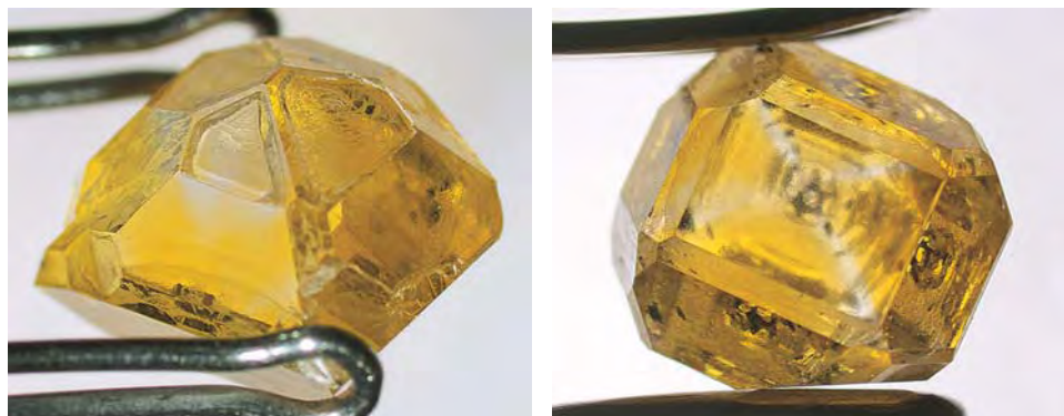
Figure 3. The 2.17 ct crystal on the left shows the cuboctahedral form typical of most synthetic diamonds grown by the temperature gradient technique. On the right, the four-fold arrangement of colorless growth sectors (and several dark metallic inclusions) can be seen in this 1.81 ct crystal. Photomicrographs by James Shigley; magnified 15× (left) and 25× (right).
