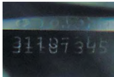
Figure 13. A mirror reflection is proof that this inscription in a 1.01 ct diamond is totally internal. Ion implantation is thought to be responsible for the inscription. Magnified 63x.
