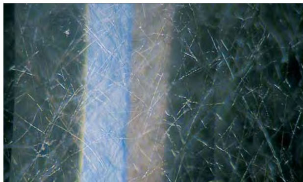
Figure 13. The milarite shown in figure 12 is filled with unusual very thin, elongate inclusions, which locally appear interrupted. Photomicrograph by Emmanuel Fritsch; magnified 7x.
