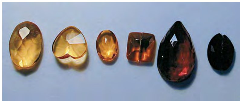
Figure 30. With increasing temperature and heating time, the color of these amber samples (left to right, samples 1 to 6 in table 1) changed from yellow to orange to dark brown. The reference sample on the far left has not been heat treated. Samples 4 and 6 were cut in half for testing purposes. The samples range from 3.2 to 13.8 ct. Photo by Morley Chang.
