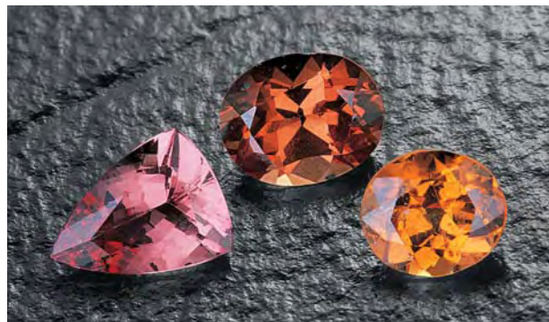
Figure 17. The pink malaya garnet on the left has a lower manganese content (sample M7; 13.04 wt. % MnO) than the orange malaya garnet in the center (sample M3; 26.63 wt. % MnO). A spessartine (sample S; 38.32 wt. % MnO) is shown on the right for comparison. The samples weigh 1.16–1.47 ct. Photo by Maha Tannous; incandescent light.
