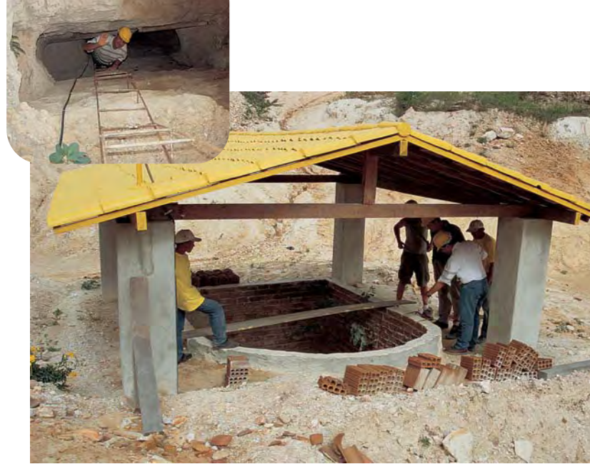
Figure 9. This shaft at the Mina da Batalha follows one of the pegmatites to a depth of approximately 20 m, and provides access to an extensive part of the underground workings. When looking down the shaft, the narrow width (typically about 1 m) and steep dip are clearly evident (see inset). The shafts were dug using hand tools, and the pegmatite material was removed by winch. Photos by Brendan M. Laurs.
