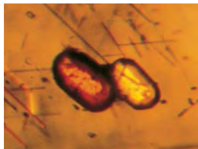
Figure 12. Apatite crystals, some with rounded edges, were identified by Raman analysis. Immersion, crossed polarizers, magnified 80 \times .
