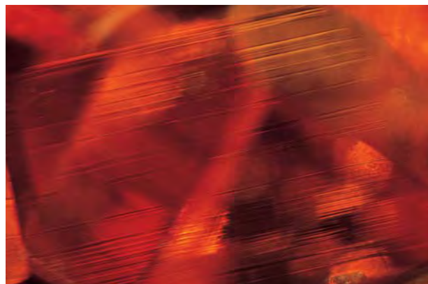
Figure 21. Parallel planar growth zoning was conspicuous in a few of the spessartines, with angular and irregular growth patterns also noted. Photomicrograph by John I. Koivula; magnified 10 \times .
