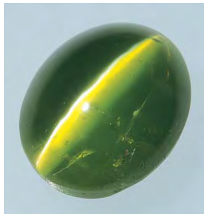
Figure 2. This 4.58 ct cat's-eye chrysoberyl cabochon had extremely high R.I. and S.G. values.
