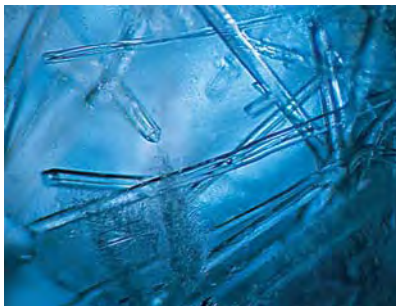
Figure 9. All of the glass beads contained numerous inclusions identified as synthetic wollastonite. Note the tiny gas bubble trapped along a groove in one of the crystals (centered in the photo). Magnified 40 \times .
