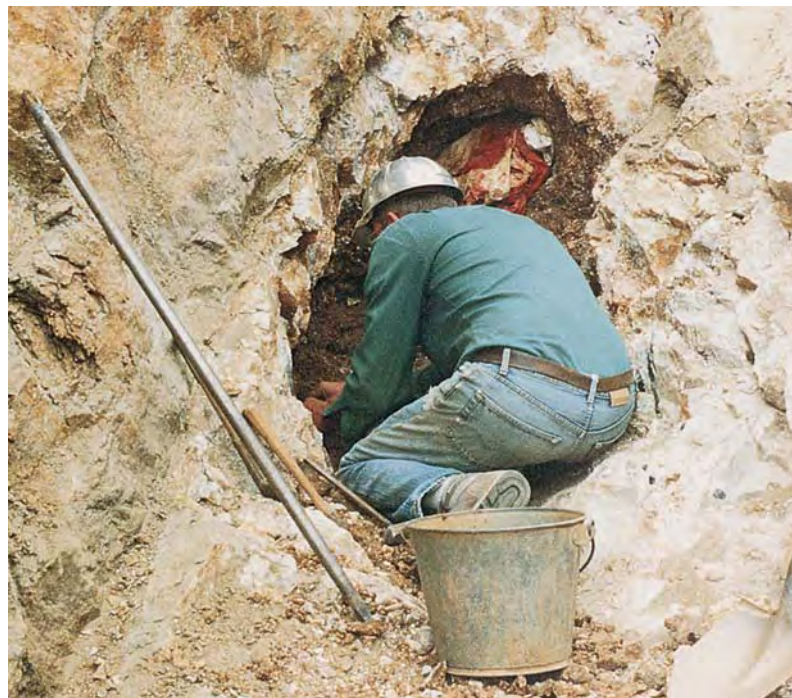
Figure 11. Spessartine-bearing pockets are carefully excavated by hand, as shown here at the Spessartite mine. Courtesy of Louis Spaulding Jr.
