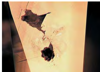
Figure 4. In reflected light, the lower cavity in the pavilion of this 3.30 ct diamond breaks the surface in a flower-like shape. Feathers can be seen extending from both cavities. A “spatter ring,” a remnant of laser drilling, is also visible around the lower cavity. Magnified 160×.
