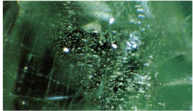
Figure 24. Partially healed fractures containing minute inclusions were often present in the Sandawana emeralds examined. Darkfield illumination, magnified 60 \times ; photomicrograph by J. C. Zwaan.
