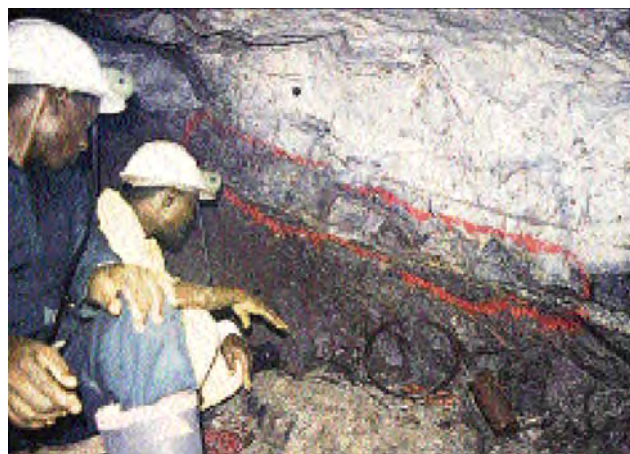
Figure 4. At Sandawana, emeralds are typically found in the zone (outlined in red here) at the contact of small pegmatite bodies and greenstone (left, in the Zeus mine, 25/28 stope, 200 foot [61 m] level). Schlieren (streaks) of actinolite and phlogopite in pegmatite are commonly seen in the "ideal" emerald-bearing pegmatite bodies (right, in the Zeus mine, 17/16 stope, 250 foot [76 m] level). Photos by J. C. Zwaan.
