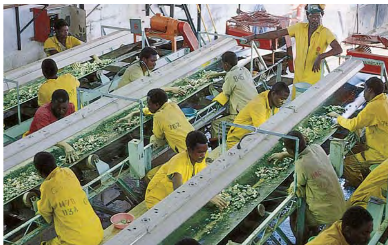
Figure 8. Ore fractions on the slow-moving conveyor belts are carefully checked for emeralds by hand-pickers. Gem-quality pieces are deposited in safety boxes by each sorter. Photo by E. J. Petsch.
