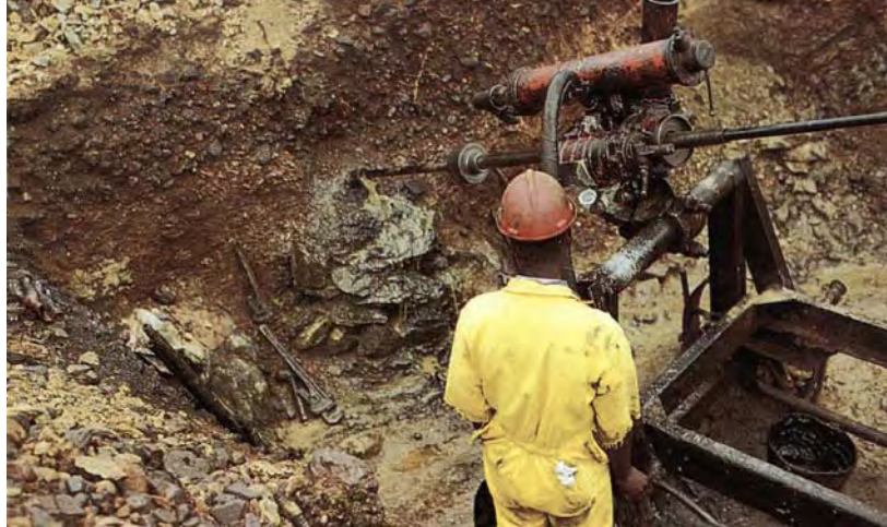
Figure 7. Exploration activities at Sandawana include (left) cross-trenching at the Aeres-3 section to find new pegmatite bodies, and (top) surface drilling at Orpheus to locate new ore zones. Photos by J. C. Zwaan (left) and E. J. Petsch (top).
