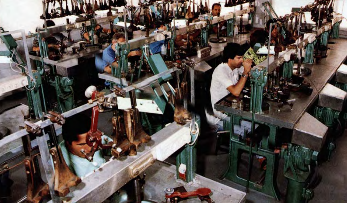
Figure 20. Polishers use a wide variety of tangs (shown here in the foreground and hanging on the central bars), depending on the facets being polished, the shape of the stone, and the like.
