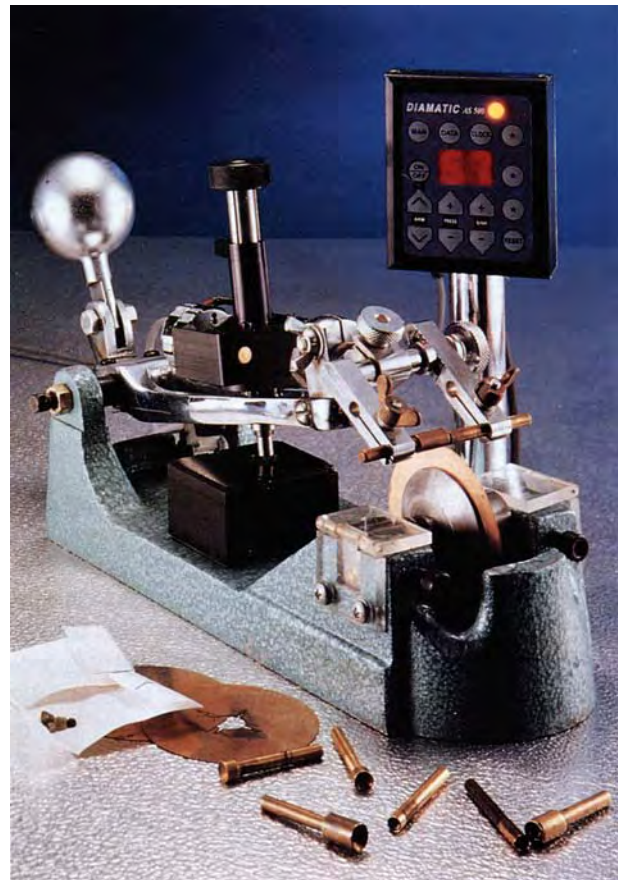
Figure 11. Modern sawing machines, like this Dialit AS500, have a pressure controller. After setting the diamond in the machine, the operator sets the required pressure of the diamond on the blade and the maximum velocity in which the diamond will be sawn. The control system continuously checks and adjusts the pressure.
