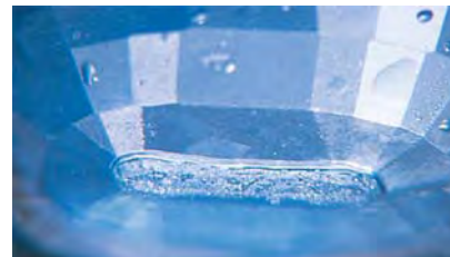
Figure 17. The melted surface at the culet of the stone in figure 16 is higher than the surface of the facets, suggesting that the culet was not repolished after treatment. Note also the rounded features that have been etched on some pavilion facets. Magnified 13×.
