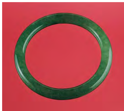
Figure 12. Although testing proved that this jadeite bangle had been dyed and polymer impregnated, examination with a handheld spectroscope did not reveal the broad absorption band centered at 640 nm that is typical for dye.
