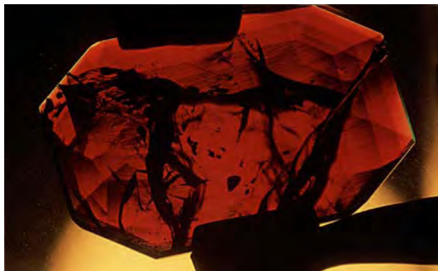
Figure 21. When the sample shown in figure 20 was immersed and viewed between crossed polarizers, two sets of rhombohedral twinning lamellae became visible (seen here on the left side of the photo to the left). Further examination revealed fine Verneuil color banding (seen here in the upper right corner of the photo to the right), which proved that the ruby is synthetic. Photomicrographs by H. A. Hänni.
