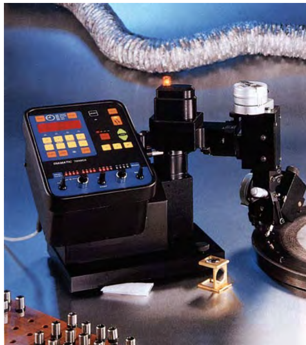
Figure 21. The Dialit GS7000 automated polishing machine (left) can polish the crown (excluding the stars) and pavilion facets on a stone. The control panel is on the left. The holder is set in the machine, with a few additional holders in the wooden cassette. The Dialit GSB800 automated blocking machine (right) can block eight facets on the crown or the pavilion. Photos courtesy of Dialit Ltd.
