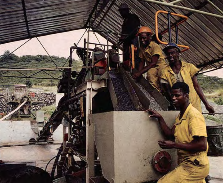
Figure 9. The high-efficiency DMS (dense media separation) module is used at Sandawana to separate emeralds in the 1.6–6 mm fraction of run-of-mine material from the other minerals that are present in the ore zone. This computer-controlled module can process about one ton of ore per hour. Photo by J. C. Zwaan.
