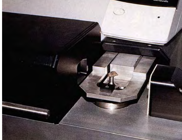
Figure 18. The Sarin automatic centering system (Dia-Center) consists of a sample chamber, light source, camera, computer, and monitor. On the right of the sample chamber (shown above) is the light source, and on the left is the camera. In front of the holder is the mechanical apparatus that moves the holder and centers the diamond. The camera measures the dimensions of the rough diamond, which is glued to a special dop, from a number of orientations. After the computer decides where the optimal center of the future cut stone will be, it moves the upper part of the dop so that the center of the diamond and the center of the bruting machine are co-axial. Photo by James E. Shigley.
