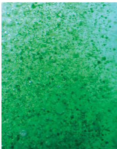
Figure 11. The green spherules in this polymer-filled cavity in a jadeite bangle make the filler much less conspicuous. Note also the many gas bubbles in the polymer. Magnified 25 \times .
