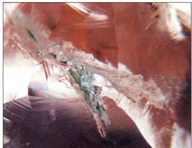
Figure 5. With 30 \times magnification, we saw that fractures in the diamond shown in figure 4 have the streaked and spotted appearance typical of natural radiation stains. The green color is largely confined to fracture surfaces.
