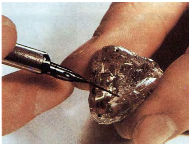
Figure 4. The most critical stage in diamond manufacturing, marking the diamond for sawing or cleaving, requires a complex decision-making process to optimize the value of the finished stones.
