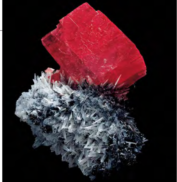
Figure 12. Cleaned of silica and mud by a combination of acids and air abrasion, the specimen in figure 11 emerges as a fine, 16-cm-high, rhodochrosite crystal on snowy white quartz and dark sphalerite crystals. Courtesy of the Collector's Edge; photo © Jeff Scovil.
