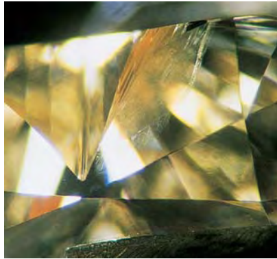
Figure 3. Stains in fractures, such as this orange limonitic stain in the stone shown in figure 2, can impart an additional aspect to the color appearance of a diamond. Magnified 32 \times .
