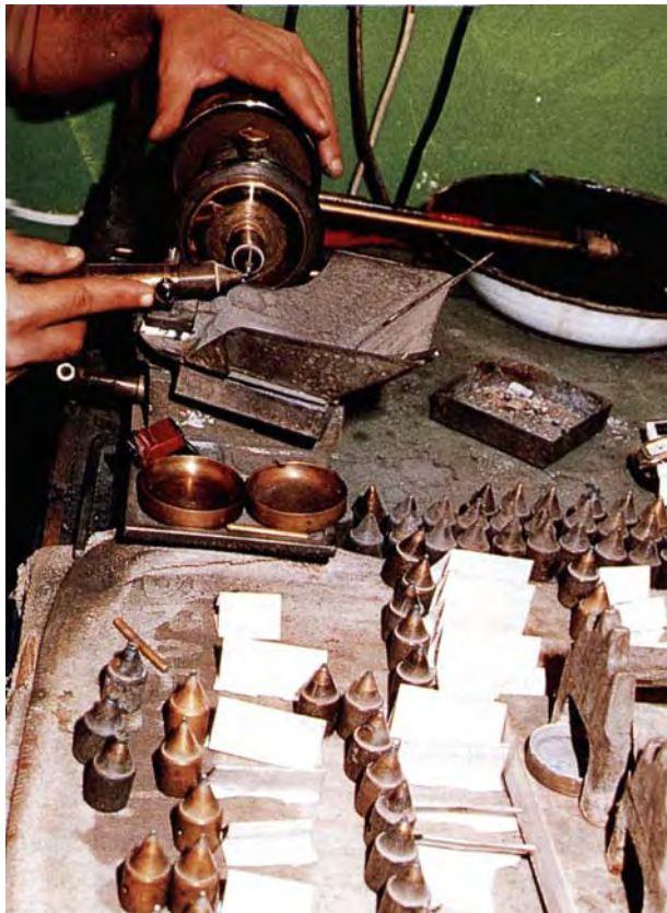
Figure 15. With a manual bruting machine, the diamond is glued to a dop that is set in the machine. In his hand, the bruter holds a stick with another dop to which a diamond has been glued. As the diamond in the machine is rotated, the other diamond is bruting it.
