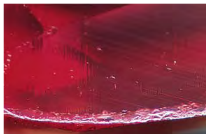
Figure 15. Characteristic thready gas bubbles in the synthetic spinel crown and curved striae in the synthetic ruby pavilion are visible in the doublet shown in figure 14 at 40× magnification.
