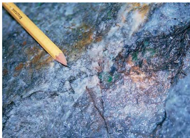
Figure 4. At Sandawana, emeralds are typically found in the zone (outlined in red here) at the contact of small pegmatite bodies and greenstone (left, in the Zeus mine, 25/28 stope, 200 foot [61 m] level). Schlieren (streaks) of actinolite and phlogopite in pegmatite are commonly seen in the "ideal" emerald-bearing pegmatite bodies (right, in the Zeus mine, 17/16 stope, 250 foot [76 m] level). Photos by J. C. Zwaan.
