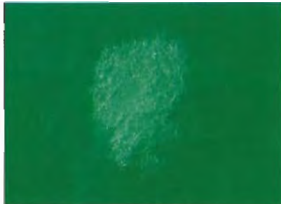
Figure 11. When we examined one of the jadeite cabochon’s dark green inclusions in reflected light at higher (40×) magnification, we found that a less reflective substance was coating the boundaries between jadeite grains in the “inclusion” regions. (Because of the light scattering, this substance appears white in the microscope.)
