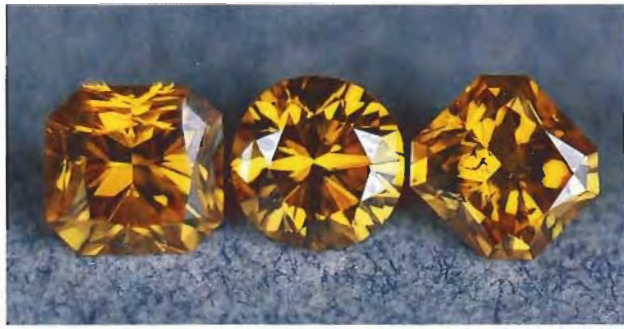
Figure 6. All three of these diamonds (from left, 0.41, 0.30, and 0.30 ct), which were submitted to the laboratory for origin-of-color reports, proved to be synthetic.
