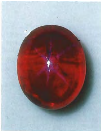
Figure 15. Although this 21.28-ct "star ruby" was somewhat included, had a good color, and appeared to be native cut, gemological testing proved that it was a synthetic ruby with a diffusion-induced star and "fingerprint" inclusions.
