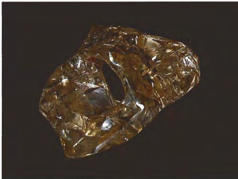
Figure 5. Although this unusual 13.34-ct rough diamond appears to be some sort of intergrowth, it is actually a single crystal with what appears to be an etched hole through the center.
