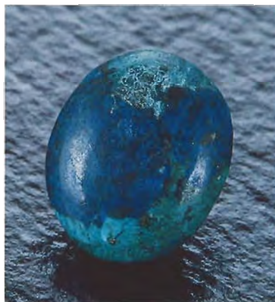
Figure 1. Testing revealed that this 3.33-ct oval cabochon is a rock consisting primarily of blue azurite, green antlerite, and quartz. The foreign material seen in surface cavities is probably a colored polymer.
