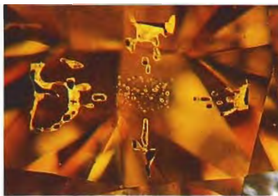
Figure 8. EDXRF analysis of one of these surface-reaching droplets—which were observed in one of the stones shown in figures 6 and 7—indicated that it contains iron and nickel, elements found in the fluxes used to synthesize diamond. Magnified 30 \times .
