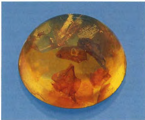
Figure 8. This 8.32-ct cabochon (19.13 × 19.23 × 7.03 mm) consists of plastic with embedded fragments of natural resin. Photo by Maha DeMaggio.
