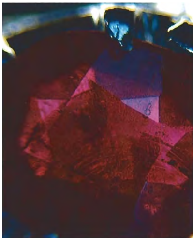
Figure 17. Sharply curved striae and dark inclusions, seen here at 19 \times , prove that the synthetic rubies shown in figure 16 are of early manufacture.
