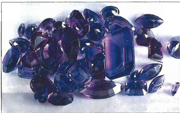
Figure 11. Note the fine color match of the natural amethysts and glass imitations in this parcel. The R.I.s are also closely matched, at 1.55.
