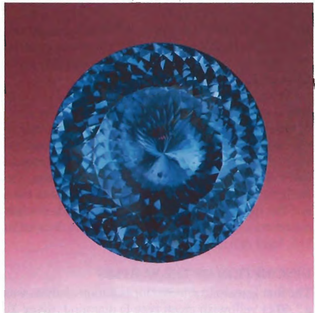
Figure 3. This unusually large, 140.5-ct, "London blue" topaz was neutron irradiated in June 1990. More than a year later, in August 1991, it still showed some radioactivity. Stone courtesy of Danny Duke, Gem Marketing International; photo by Shane F. McClure.
