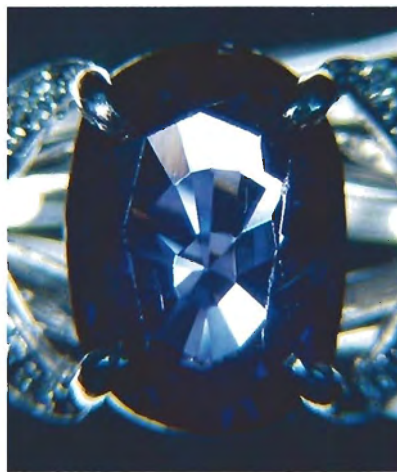
Figure 18. The abraded facet junctions on this approximately 3-ct diffusion-treated sapphire probably could not be repolished without removing part of the shallow color layer.
