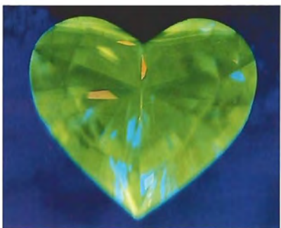
Figure 5. The strong fluorescence to long-wave U.V. radiation (and persistent phosphorescence) of the stone in figure 4 is typical of chameleon-type diamonds.
