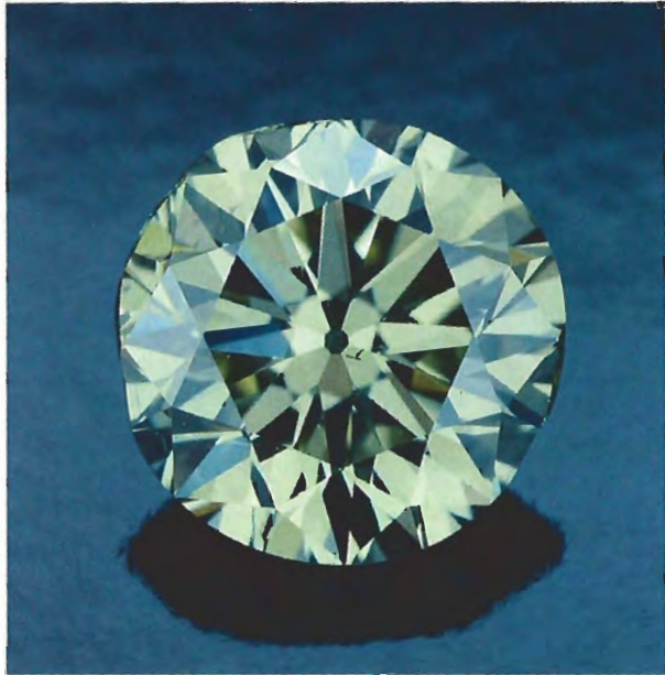
Figure 2. Gamma-ray spectroscopy determined that this 2.60-ct yellowish green diamond, believed to have been radium treated when purchased in 1983, was actually color enhanced by americium-241. GIA Gemstone Reference Collection no. 14052; photo © GIA and Tino Hammid.
