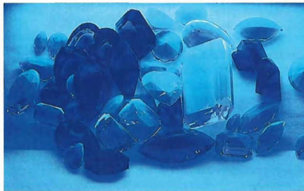
Figure 12. In this parcel, the glass imitations fluoresce chalky blue—while the amethysts are inert—to short-wave U.V. radiation.
