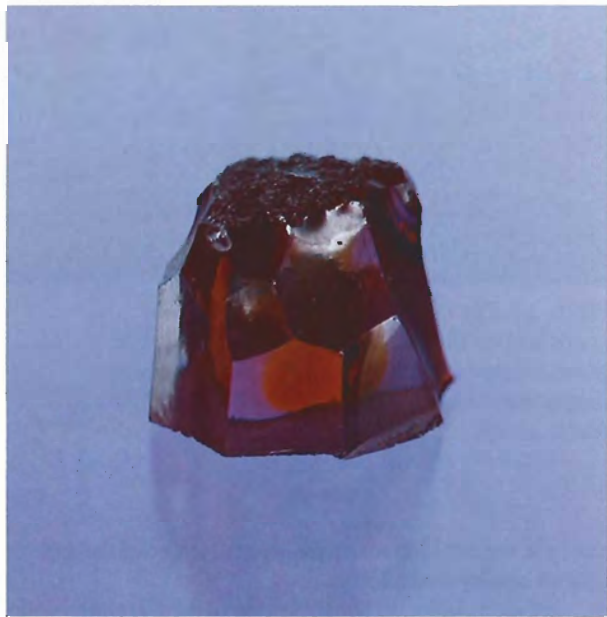
Figure 15. This 230.10-ct CZ displays interesting color zoning due to a combination of the dopants and growth conditions used. Photo by Maha Smith.
