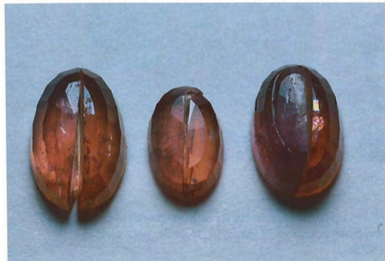
Figure 15. The Umba Valley sapphires reportedly do not respond to heat treatment as well as sapphires from some other localities. These three sapphires from the Umba Valley were cut and the left half of each heat treated to provide some idea of the extent of the change produced. Stones and experiment courtesy of the GIA Research Department; photo © GIA and Tino Hammid.
