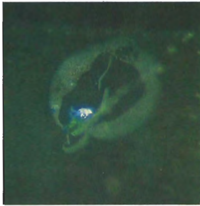
Figure 7. High magnification (126x) revealed that what was believed to be "jardin" in an emerald is actually a combination of bubbles and flux in a green YAG.
