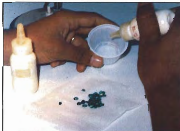
Figure 4. After Opticon treatment at Stone World, the emeralds are coated with a mixture of Opticon and hardener—here, being prepared—to seal the surface-reaching breaks. Photo courtesy of Stone World.
