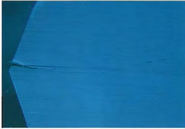
Figure 6. The use of surface-reflected light with the microscope enables the location of surface-reaching fractures in treated emeralds. Photomicrograph by John I. Koivula; magnified 25 \times .
