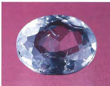
Figure 10. Before ultrasonic cleaning, no fractures were visible in this 1.78-ct cedarwood oil-treated aquamarine (left). Within 10 minutes in the ultrasonic, some of the oil had been removed; after 25 minutes, a multitude of fractures had become visible (right). Photos by Maha Smith.
