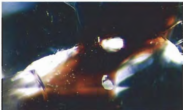
Figure 12. When this Opticon-treated beryl was exposed to the heat of a jeweler's torch during a procedure approximating the retipping of prongs, Opticon boiled out of some of the fractures and darkened, leaving a brown residue on the surface. Photomicrograph by John I. Koivula; magnified 30 \times .
