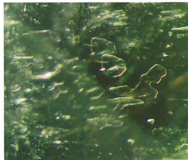
Figure 9. Careful examination of the areas surrounding trapped air bubbles will sometimes reveal subtle flow structures within the filling agent, which in this case is Opticon. Photomicrograph by John I. Koivula; magnified 20 \times .
