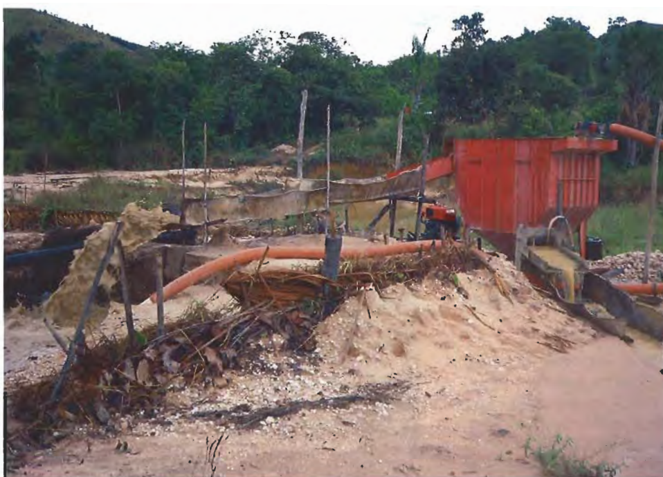
Figure 4. The separator jig shown here is used to recover both gold and diamonds in this Brazilian alluvial mining operation. Photo by Patricia Maddison.
