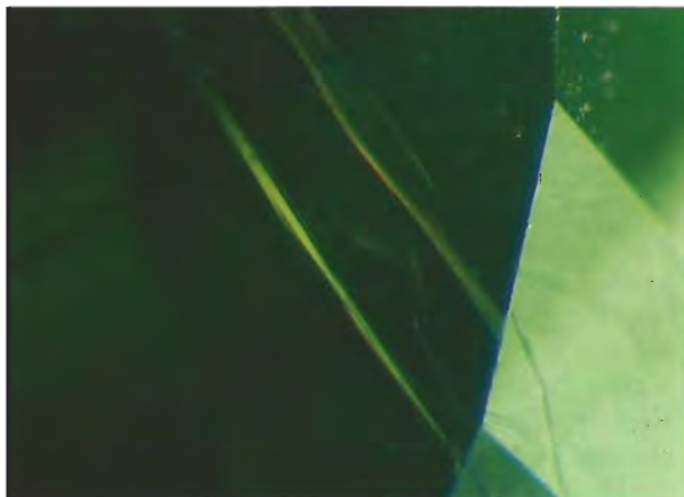
Figure 7. A slightly orangy yellow flash (left) was observed in the filled fractures of this Opticon-treated emerald. When the stone was tilted slightly and the background became lighter, the flash turned blue (right). In some stones, only one color is seen. Photomicrograph by John I. Koivula; magnified 20 \times .
