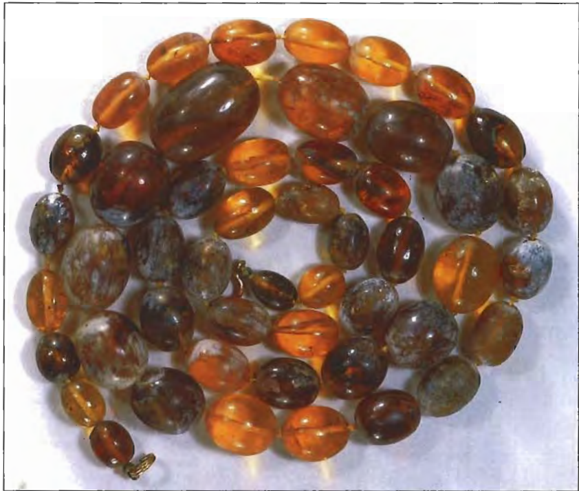
Figure 1. When these amber beads (10.25 × 7.34 mm to 25.30 × 16.75 mm) were "washed" by immersion in alcohol, many of them acquired a white film that could only be removed by repolishing.
