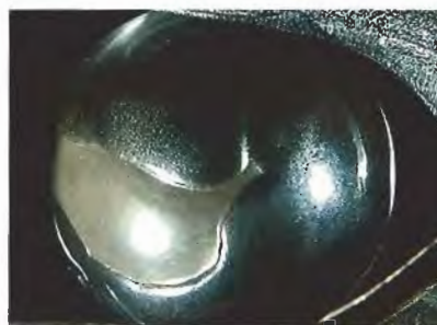
Figure 2. The light-colored nucleus visible under the dark surface of this calcareous concretion has no apparent structure and thus cannot be a shell bead. Magnified 5 \times .
