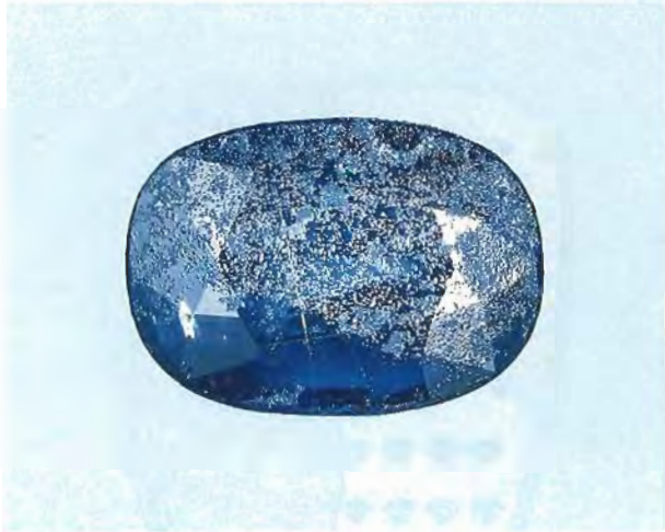
Figure 6. Partially reflected light reveals the rough, sintered surface on this unrepolished 3.37-ct diffusion-treated sapphire. Courtesy of Gem Source; photo by Shane F. McClure.
