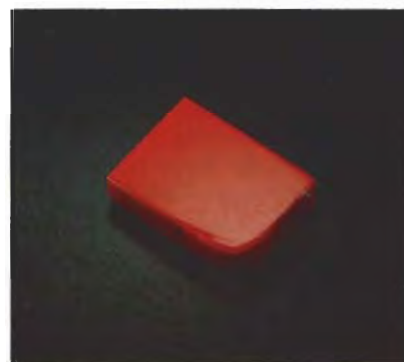
Figure 3. This 21.26-ct slab of imitation coral is comprised of barium sulfate, a plastic binder, and a coloring agent.
