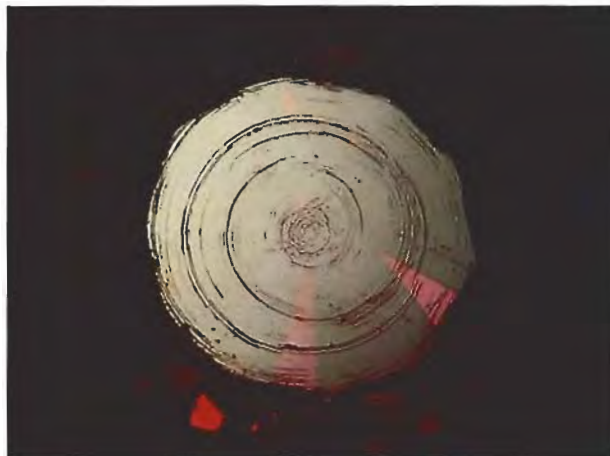
Figure 5. After only one 360 ^\circ rotation in the jaws of the diamond-impregnated tweezers, considerable damage was done to the table facet of the synthetic ruby seen in figure 3. Photomicrograph by John I. Koivula; magnified 5 \times .
