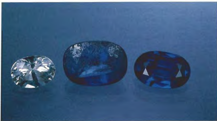
Figure 8. These three stones (1.10–3.37 ct) represent the various stages involved in producing diffusion-treated blue sapphires: Left, the starting material is a faceted colorless (or light-colored) sapphire; center, the use of chemicals and extreme heat produces a dark blue stone with rough, corroded, and “pock-marked” surfaces; right, repolishing produces a finished blue diffusion-treated sapphire. Courtesy of Gem Source; photo by Shane F. McClure.
