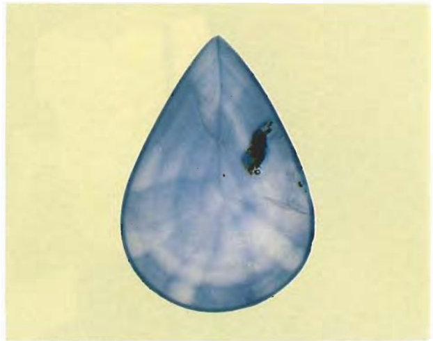
Figure 14. In addition to high relief and color concentrations at facet junctions, immersion may also reveal a blotchiness of the diffused color layer caused by a combination of uneven diffusion and light repolishing. Photo by Shane F. McClure.
