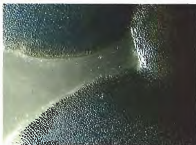
Figure 1. The cellular structure characteristic of calcareous concretions is readily apparent in these dark surface areas. Magnified 20 \times .
