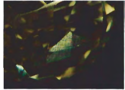
Figure 15. Plato lines characteristic of synthetic yellow sapphire were visible in this 6.93-ct stone even without magnification (shown here at 10x for clarity).
