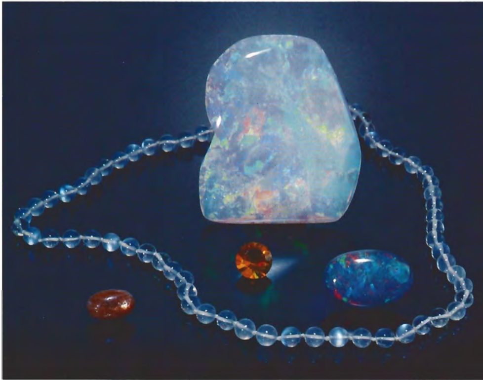
Figure 1. Colors in gem materials can be caused by a wide variety of processes. This article explains color-producing mechanisms related to band theory and physical phenomena. Examples of the latter include diffraction in opal (in the center top and bottom right), scattering of light in “moonstone” feldspar (the necklace), and coloration by inclusions in fire opal (center bottom) and “sunstone” feldspar (bottom left). The necklace is courtesy of Elise Misiorowski; photo by Robert Weldon.
