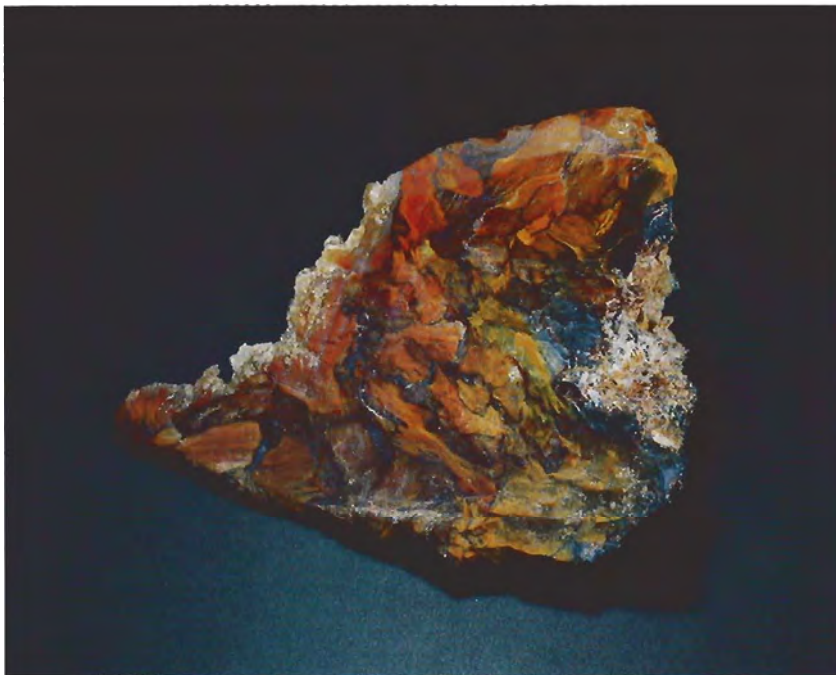
Figure 18. In this rough piece (5.4 cm at its largest dimension), the components of this material are evident in a 1-cm-deep cavity lined with drusy quartz on the left, brecciated tiger's-eye quartz in the center, and unaltered blue crocidolite on the right.
