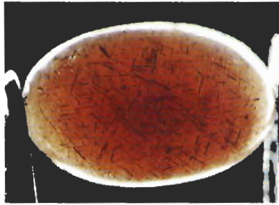
Figure 14. When the stone shown in figure 13 is viewed with transmitted light and at 10x magnification, both the actual brown color and the ilmenite inclusions that make the stone look black in reflected light are evident.
