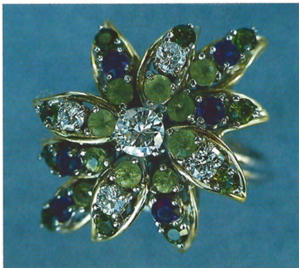
Figure 11. Use of the torch during a retipping procedure on the center diamond resulted in the permanent clouding of the surrounding peridots, which are very heat sensitive.
