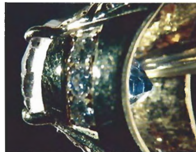
Figure 12. The concentration of color in the culet area of the synthetic sapphire shown in figure 11 lends the color to the entire stone when seen face up. Note also the unusual depth-to-width ratio of this stone.
