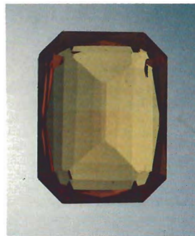
Figure 13. The curved striae in this 15.54-ct yellow flame-fusion synthetic sapphire are unusually apparent.
