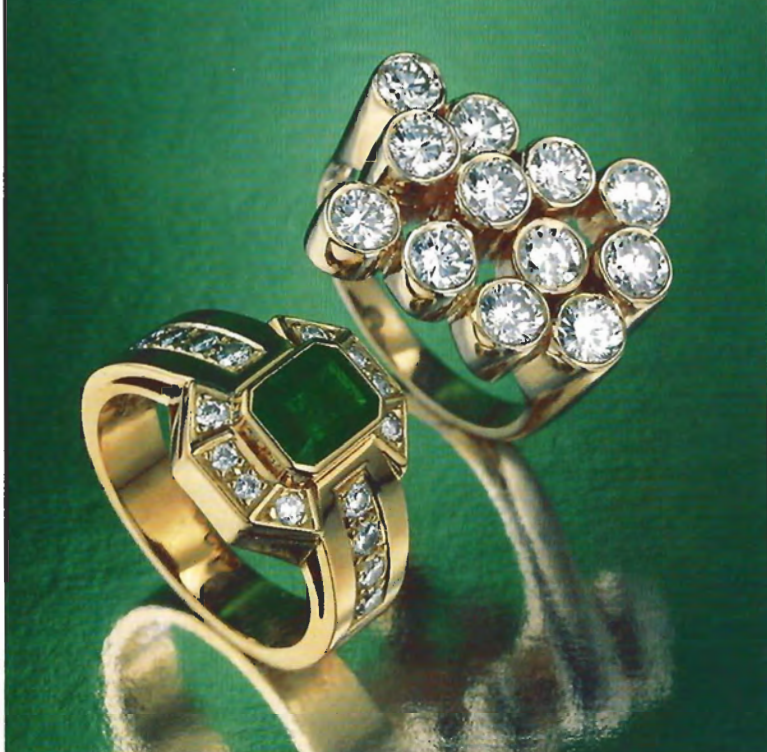
Figure 3. Bezel settings help protect the girdle and pavilion areas of any gemstone, but are particularly useful for stones that are less durable or, like the bezel-set emerald shown here, have a tendency to chip or crack. Tube setting requires more pressure in burnishing than a regular bezel setting and so is recommended only for more durable stones, such as the diamonds shown here. Emerald ring by Silverhorn, Montecito, CA; diamond ring by The Altobelli Jewelers, North Hollywood, CA. Photo © Tino Hammid.
