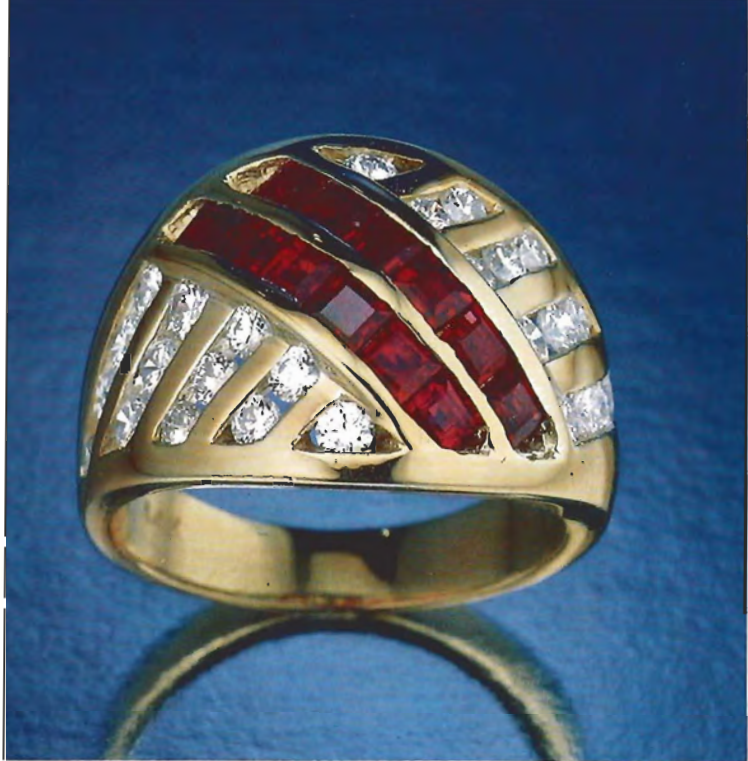
Figure 5. Diamonds and rubies (or any other variety of corundum) are best suited for channel setting because of their durability. Ring courtesy of the Altobelli Jewelers, North Hollywood, CA; photo © Tino Hammid.
