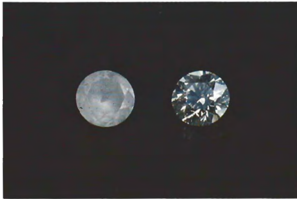
Figure 12. Improper use of the jeweler's torch caused permanent clouding and cracking of the diamond on the left, shown here with an undamaged diamond. Photo by Robert Weldon.
