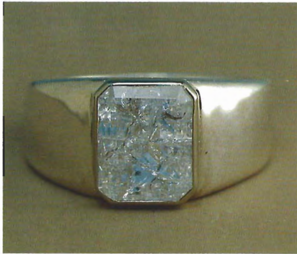
Figure 16. Even the most durable of gemstones, diamond, can be severely damaged by thermal shock.
