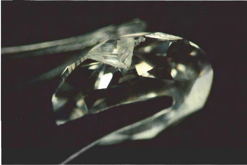
Figure 4. Blocked out 2.5-ct diamond that broke on the wheel. Magnified 10 \times .
