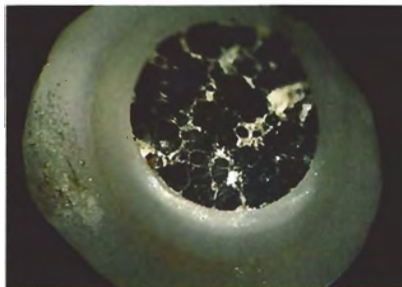
Figure 13. An 8-mm imitation pearl showing a metallic core and iridescent ring. Magnified 15×.
