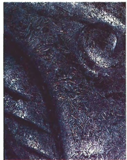
Figure 7. Extensive etching caused by immersion of the fluorite carving shown in figure 6 in a sulfuric acid solution. Magnified 30 \times .
