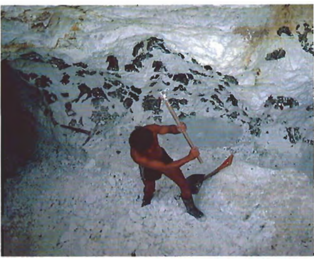
Figure 10. Many gem pockets have been found in the soft kaolin of Golconda II. The black tourmaline lining the walls is an indication that gem crystals may be nearby.
