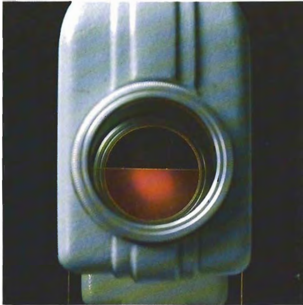
Figure 3. View through a polariscope with the first-order red compensator inserted halfway through the polarized light field.
