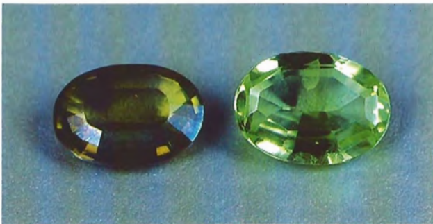
Figure 4. The stone on the left is Arizona peridot GIA #12430A after heat treatment. Its original color was the same as that of the peridot shown on the right in this photo.
