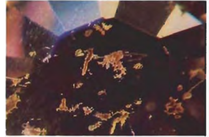
Figure 17. Unusual root-like inclusions in natural spinel. Dark-field illumination, magnified 20x.
