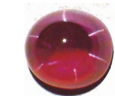
Figure 13. Synthetic star ruby (4.22 ct) cut from a piece near the bottom of the boule from which the stone in figure 12 was cut. Note that the rays of the star do not meet in the center of the stone.
