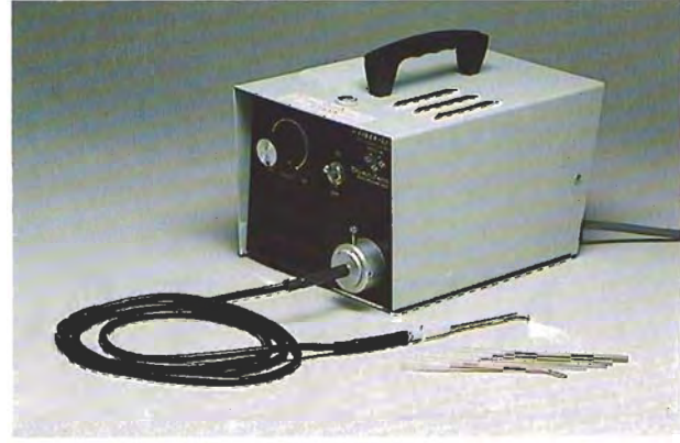
Figure 2. The quartz-halogen illuminator adapted for pinpoint illumination.
