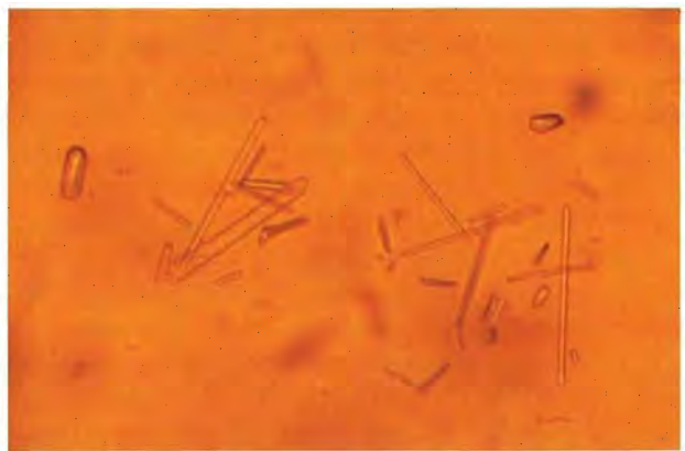
Figure 13. Apatite and diopside crystals in hessonite garnet. Magnified 30×.
