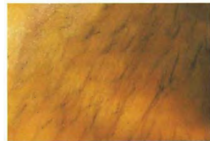
Figure 8. Dark streamers in opal. Transmitted light, magnified 50\times .
