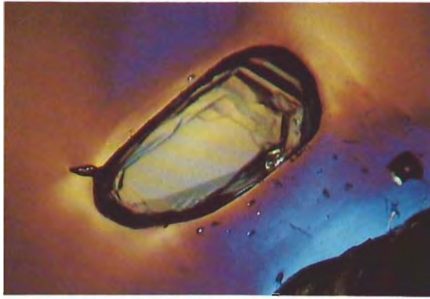
Figure 6. An included crystal in a natural Burmese pink spinel is lit by polarized pinpoint illumination. The clarity of this photograph is startling considering the difficult angle of illumination and the degree of magnification, 100 \times .
