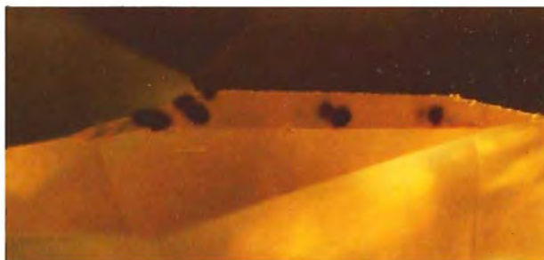
Figure 9. Natural radiation "staining" on an unpolished portion of the girdle of the stone referred to in figure 8. Magnified approx. 70×.
