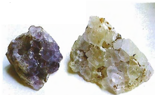
Figure 18. Fluorite before (colorless) and after irradiation.
