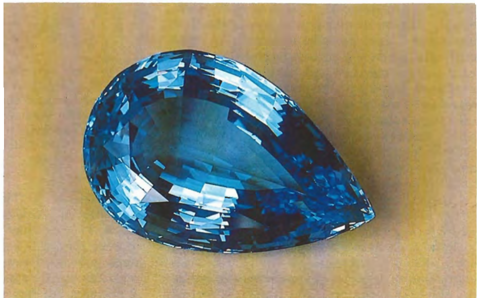
Figure 15. Blue topaz in which color has been produced by irradiation followed by heat treatment.
