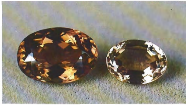
Figure 14. Comparison of a light natural brown and a dark irradiated brown topaz. Some natural brown topazes can be as dark as the irradiated stone pictured here.
