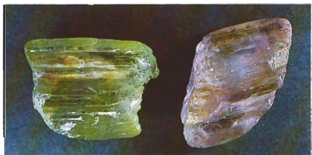
Figure 13. Kunzite before (pink) and after (green) irradiation with cobalt-60 gamma rays.
