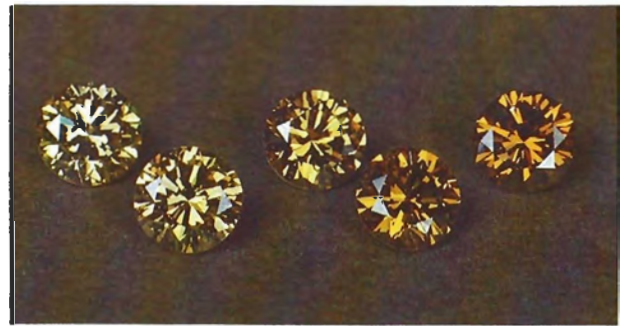
Figure 24. Heat treatment of irradiated diamonds produces orange and yellow colors.
