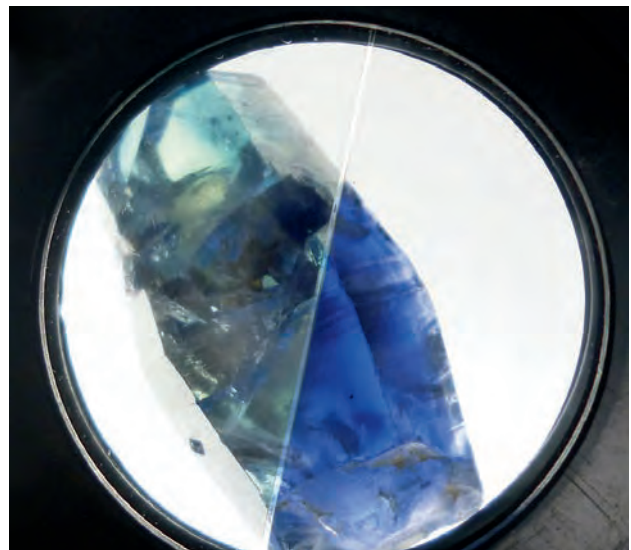
Figure 13. Strong dichroism is observed with the London dichroscope in this 5.7 g sapphire. Photo by D. Dillimuni.
