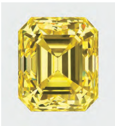
Figure 1. Spectroscopic analysis showed that this 50.86 ct Fancy Vivid yellow emerald-cut diamond had been artificially irradiated.
