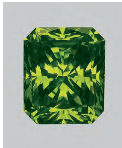
Figure 2. This 0.99 ct diamond’s saturated yellowish green color resulted from a multistep process involving HPHT treatment and irradiation.
