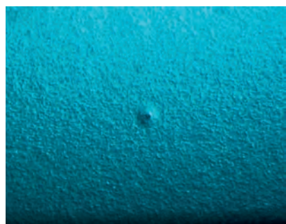
Figure 14. Microscopic examination of the imitation opal with shadowed illumination showed a granular pattern and small pinpoint inclusions surrounded by an optical halo. Image width 0.80 mm.
