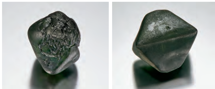
Figure 6. These rough diamond crystals (15.77 and 14.42 ct) were coated to mimic the appearance of naturally irradiated green diamonds.
