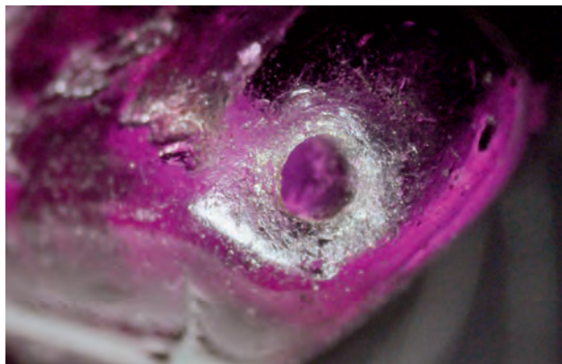
Figure 28. No chipping of the coloration was seen around the drill holes of the bead, making it quite difficult to detect the coating. Photomicrograph by G. Choudhary; magnified 20x.
