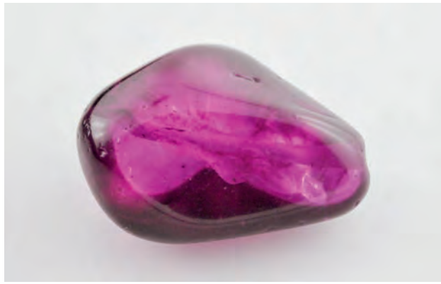
Figure 27. This 22.99 ct purplish pink bead resembled rubellite tourmaline but was identified as coated quartz. Photo by G. Choudhary.
