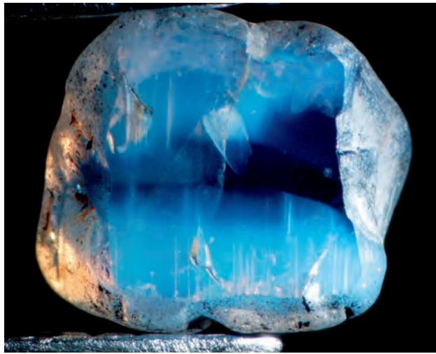
Figure 20. This 0.25 g untreated sapphire from Ilakaka, Madagascar, has cloudy areas containing traces of Be, Nb, and Ta. Photo by Shane F. McClure.
