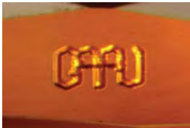
Figure 4. During the laser ablation process, our research showed that inscribing the GAAJ logo on the girdle of a gemstone provided sufficient material for analysis of one area; this inscription also proves that a sample has been analyzed by LA-ICP-MS. The tiny mark measures 80 \times 230 \mu\text{m} and penetrates the stone to a depth of ~5–10 \mu\text{m} . Photomicrograph by A. Abduriyim; magnified 80 \times .
