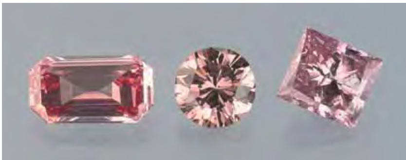
Figure 10. The intense pink color of these three diamonds (0.70–1.05 ct) proved to be the result of a surface coating.
