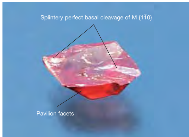
Figure 5. The first rhodonite crystal (2.50 ct) cleaved along the M plane during faceting. Note the outline of the pavilion facets, which were almost completed. The crown was unrecoverable. Photo by P. Millsted.
