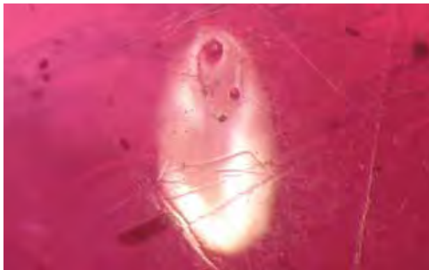
Figure 42. This ruby bead contains filled fractures and twin planes, as well as cavities with multiple gas bubbles. Photomicrograph by H. A. Hänni, © SSEF Swiss Gemmological Institute; magnified 30x.
