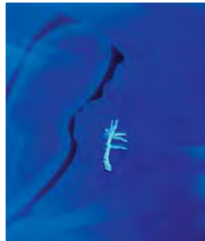
Figure 14. DiamondView fluorescence imaging revealed that the etch channel formed within a specific growth zone, indicating that its development was probably controlled by localized lattice defects.
