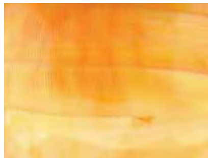
Figure 18. A close-up image of the sphere in figure 17 reveals a coarse flame structure oriented perpendicular to the banded shell structure, and the presence of dye concentrations in fractures and cavities.
