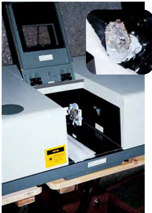
Figure 9. The Cullinan II diamond, still in its basket setting, is positioned with Blu Tack in the beam of the Nicolet 510 FTIR to measure its infrared spectrum. The inset provides a closer view of Cullinan II in the sample chamber. Photos by K. Scarratt.
