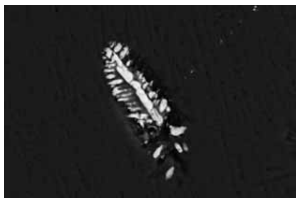
Figure 16. When heated above 1680°C, nearly all the zircon inclusions showed some degree of melting, in addition to subsolidus reactions. In this inclusion, the quenched baddeleyite had a dendritic structure. BSE image width 85 μm.
