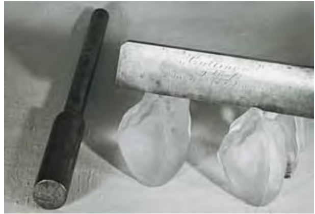
Figure 5. The hammer and knife used to cleave the Cullinan diamond. The knife is seen here spanning two models of the rough Cullinan. Photo by Alan Jobbins.
