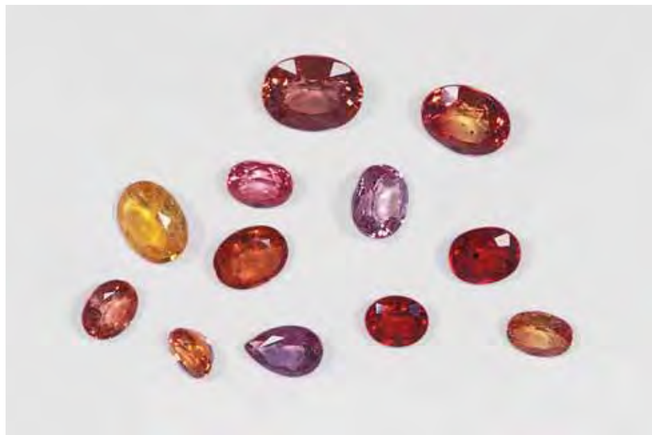
Figure 6. These Be-diffused sapphires and rubies (0.45–3.98 ct) are typical of the material that was analyzed by LA-ICP-MS for this study. Photo by Masaaki Kobayashi.
