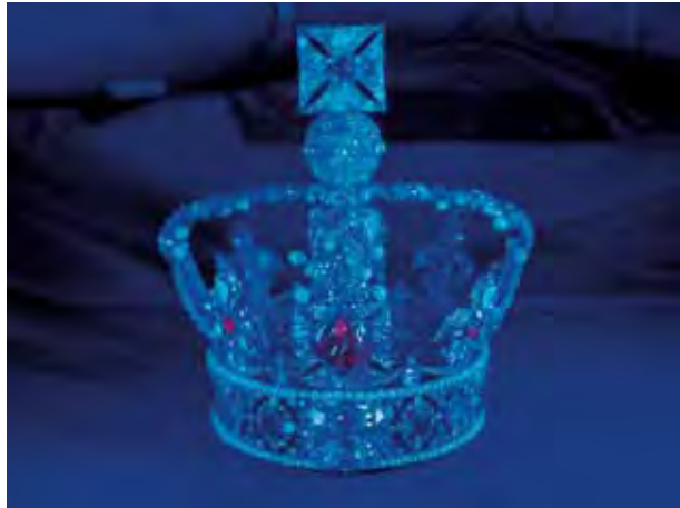
Figure 17. The Imperial State Crown with Cullinan II in place is shown during exposure to long-wave UV radiation. Note that the Cullinan II is inert under these conditions. A ruby inset in the red spinel (the Black Prince's "Ruby," which had been pierced during medieval times to be worn as a pendant) located above the Cullinan II and two rubies set in fleurs-de-lis show red fluorescence; several other diamonds show blue fluorescence. Photo by Alan Jobbins.
