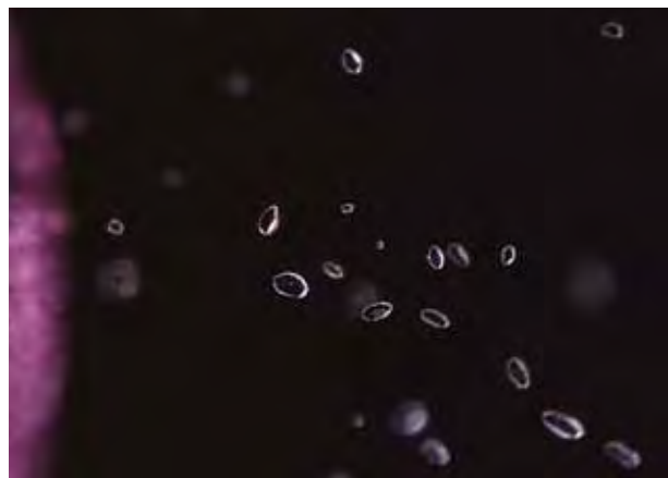
Figure 2. Discrete zircon inclusions were common in the Madagascar sapphires. With magnification, the interfaces between the zircon inclusions and their host sapphire were almost always clear and transparent, showing no frostiness or turbidity. The crystal faces were flat or somewhat rounded and shiny. Photomicrograph by W. Wang; magnified 90 \times .
