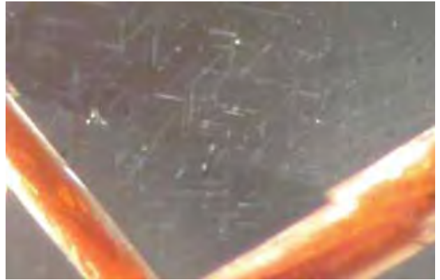
Figure 28. Higher magnification reveals fine needles and platelets in the sapphire, which are oriented in three directions at approximately 60° to one another. They show that the sapphire has not undergone high-temperature heat treatment. Also visible is a portion of the “hockey stick” inclusion in figure 27. Photomicrograph by G. Choudhary; magnified 70 \times .
