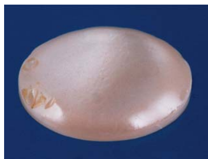
Figure 5. Magnification revealed that this 0.55 ct cabochon was assembled from a mother-of-pearl base and a plastic top.
