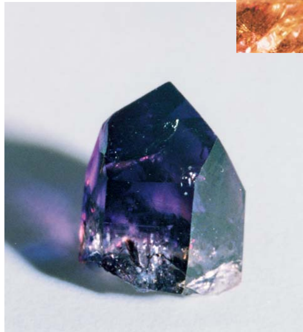
Figure 11. The shape of this approximately 1 cm wide synthetic amethyst crystal, one of several examined recently in China, resembles that of a natural crystal. Because these crystals are grown on dome-shaped seeds, there was no obvious seed plane. Inset: These “nail-head” inclusions extend from the curved seed into the synthetic amethyst. Macro photo by Zhang Tao, NGTC; photomicrograph by Shen Meidong, magnified 25x.
