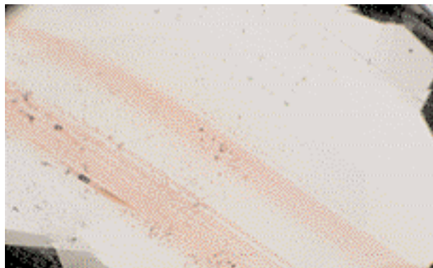
Figure 13. Curved planes of liquid and two-phase inclusions crossed the pink color bands at random angles in this natural pink quartz from Brazil. Photomicrograph by Shane F. McClure; magnified 10x.
