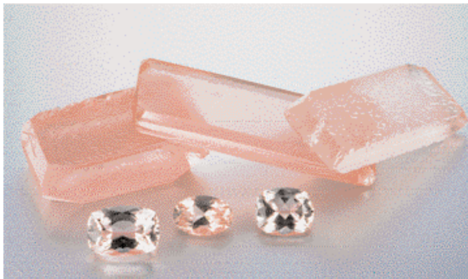
Figure 1. Transparent synthetic pink quartz is now being manufactured commercially in Russia. These crystals (132.25–193.76 ct) and faceted samples (7.30–15.97 ct) of synthetic pink quartz are some of the samples used in this study. Photo by Maha DeMaggio.
