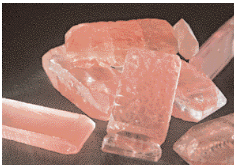
Figure 4. These synthetic pink quartz crystals (70–80 mm long and 10–18 mm thick) are representative of the samples studied in Russia and at GIA. Photo by Mikhail A. Bogomolov.
