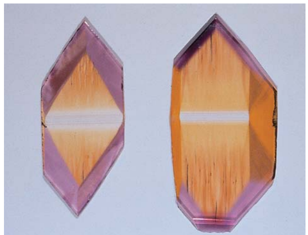
Figure 21. Synthetic ametrine grown in Russia is now commercially available. The smaller crystal measures 51 x 21 x 5 mm. Photo by Maha DeMaggio
