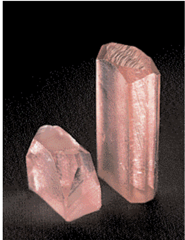
Figure 16. These two samples of synthetic pink quartz are shown here three years after they were irradiated, at which time they were both the same color. However, the crystal on the right (52 mm long x 10 mm thick) was kept in the dark for the three years, whereas the crystal segment on the left (23 mm long and 12 mm thick) was one of several that were exposed to sunlight throughout this period. The fact that there is very little difference in color between the two samples indicates that the color appears to be stable over time. Photo by Mikhail A. Bogomolov.
