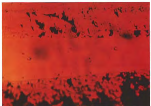
Figure 6. On the surface of this faceted Lechleitner synthetic ruby, the boundaries between the Verneuil-grown "seed" (center) and the partially removed flux-grown skin are readily apparent. Photomicrograph by K. Schmetzer; immersion, magnified 50×.
