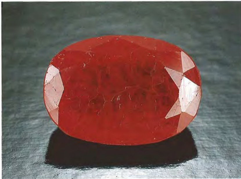
Figure 4. Flux-induced inclusions like those shown in figure 3 were seen throughout this 9.93-ct sample (approximately 10.3 × 14.8 mm) of a new type of treated synthetic ruby. Photo © GIA and Tino Hammid.
