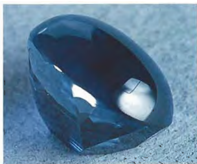
Figure 19. A side view of the star sapphire shown in figure 18 reveals the cabochon top and faceted pavilion characteristic of the cutting style known as a buff top.
