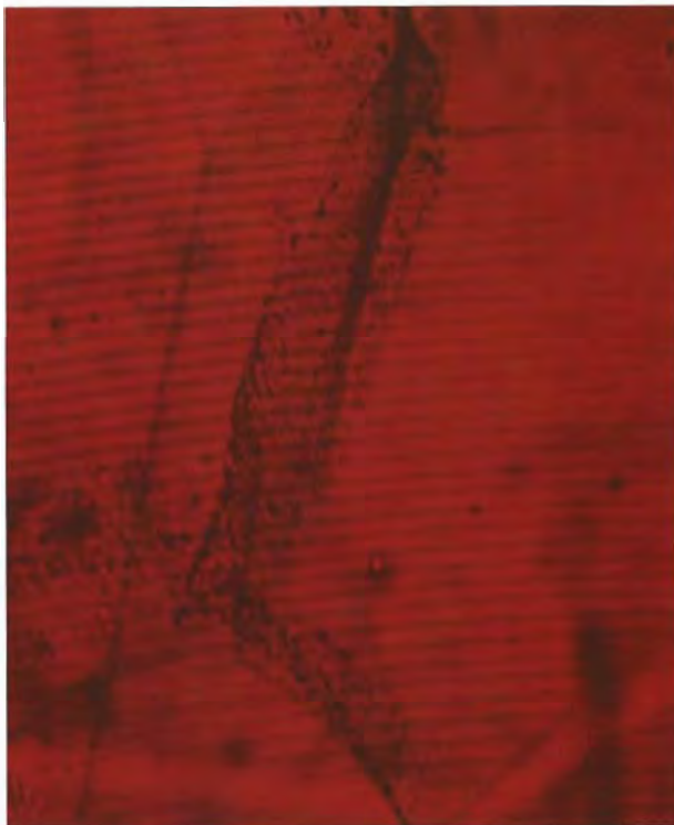
Figure 8. In this Lechleitner flame-fusion synthetic ruby, both curved striae and the "fingerprint" patterns of residual flux are readily visible. Photomicrograph by K. Schmetzer; immersion, magnified 85 \times .
