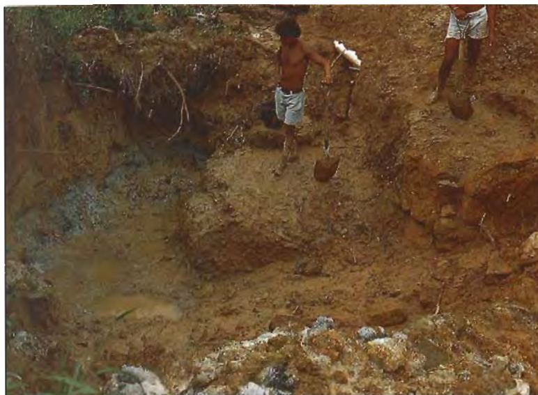
Figure 4. Nearly 2 m of clay-like material was removed with simple shovels to reach the sapphire-bearing gravels.
