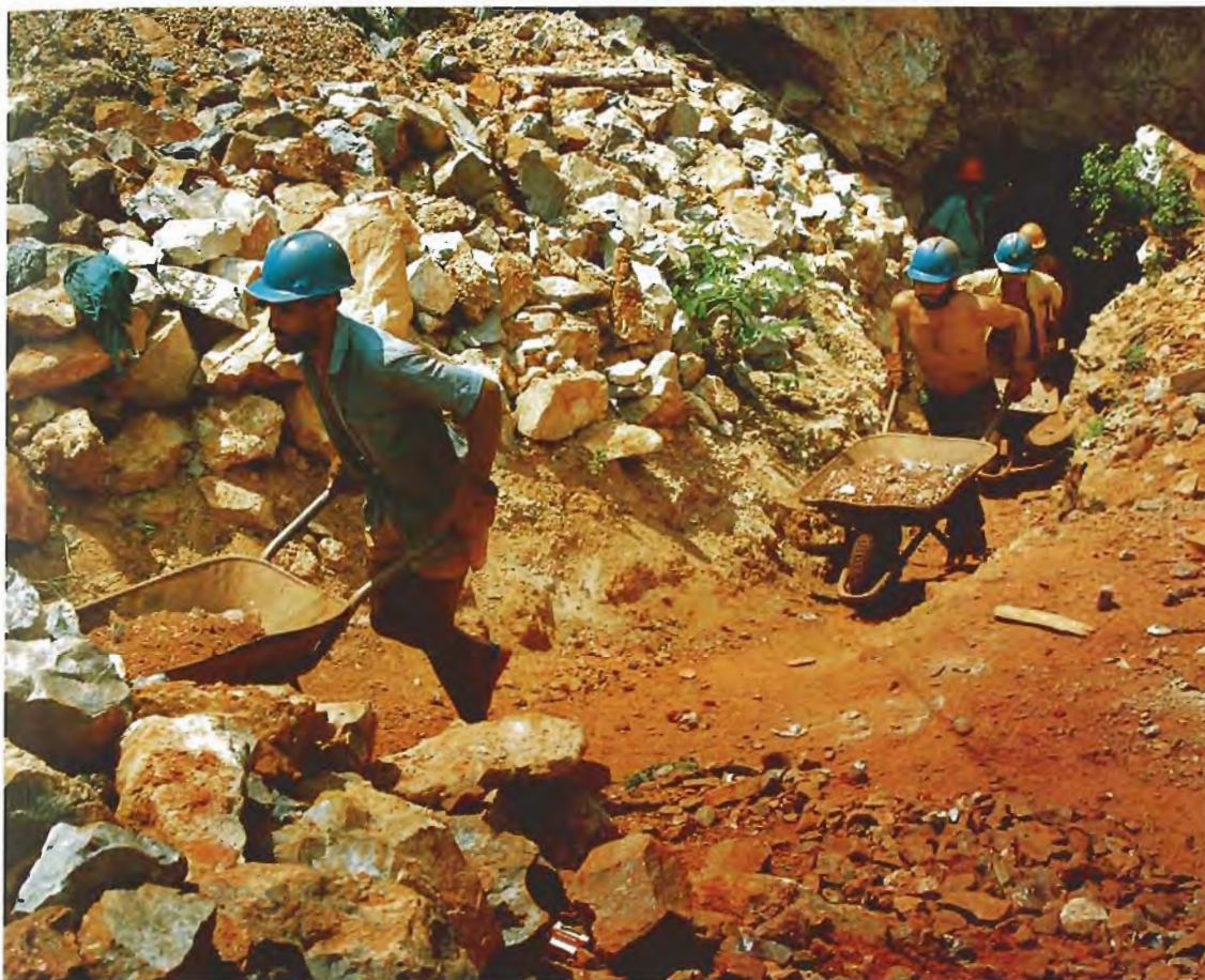
Figure 8. Miners transport barren host rock and clay to the dump sites in wheelbarrows. Note the large, brecciated limestone blocks. Photo courtesy of Minerales y Metales del Oriente S.R.L.
