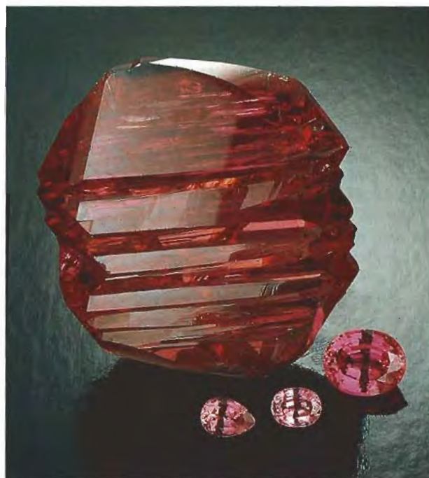
Figure 17. This 884-ct crystal and three faceted stones (the largest weighs 13.35 ct) are representative of the new flux-grown pink synthetic sapphires being produced by Chatham Created Gems, San Francisco. Photo by Robert Weldon.
