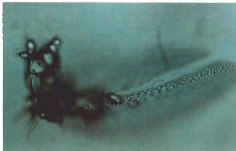
Figure 9. This brown-stained inclusion looks like zircon. Note the tension halo associated with a healed fracture. Photomicrograph by J. C. Mendes; magnified 200x.
