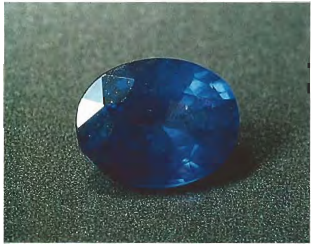
Figure 3. This approximately 1-ct sapphire, represented as diffusion treated, was found to be surface coated. Photo by Tony Laughter.
