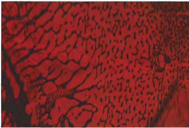
Figure 1. Induced fingerprint-like patterns of residual flux are seen here in a Verneuil-grown synthetic ruby treated by Chatham Created Gems. Photomicrograph by K. Schmetzer; immersion, magnified 40 \times .
