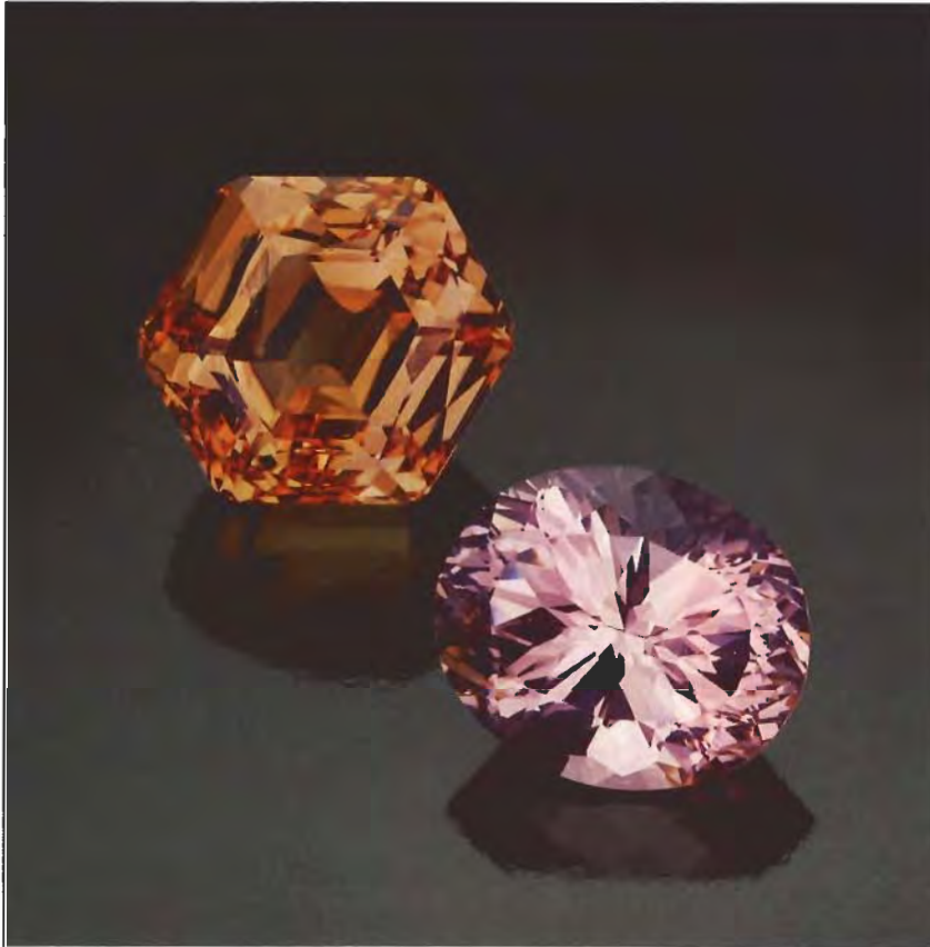
Figure 5. Both of these gems are from the 1986 discovery at the Bananal mine. The 131-ct pink morganite was the same color as the 235-ct pinkish orange stone before exposure to strong Southern California sunlight for approximately one month. Courtesy of Ramsey Gem Imports, Inc.; photo © Tino Hammid.
