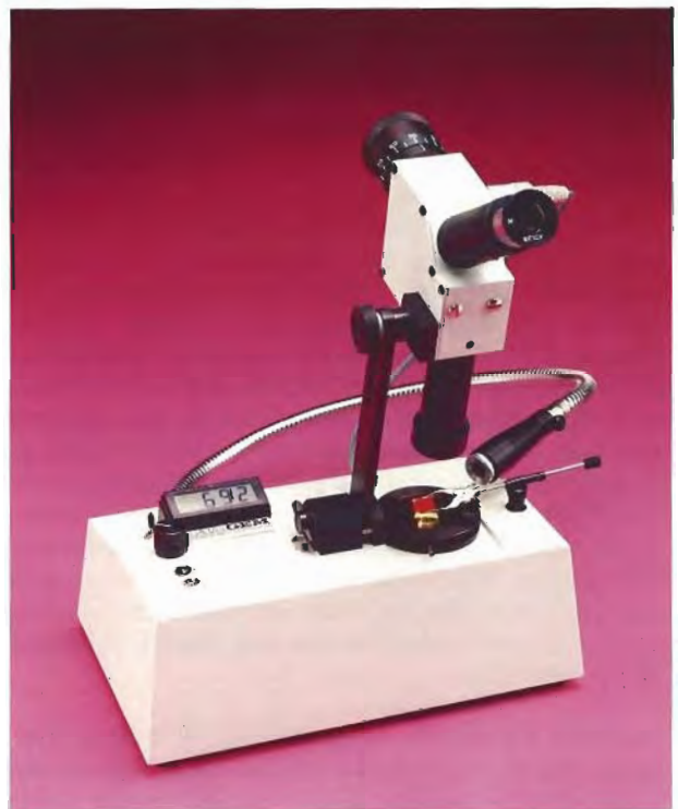
Figure 12. The new DISCAN spectroscope has a crosshair scanner coupled with a liquid crystal display so that an absorption feature can be lined up precisely and its exact numeric position (in nm) read in the digital display window.
