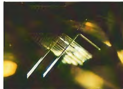
Figure 4. These sets of parallel "needles," which intersect at 90°, are unusual in diamond. Magnified 45 \times .
