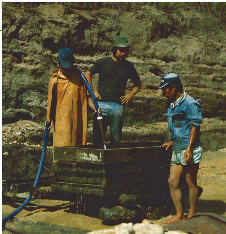
Figure 8. To sort the gem gravels quickly and efficiently at Barro Preto, the miner uses a water cannon to force them through four screens of different mesh. Photo by Henry Kennedy.
