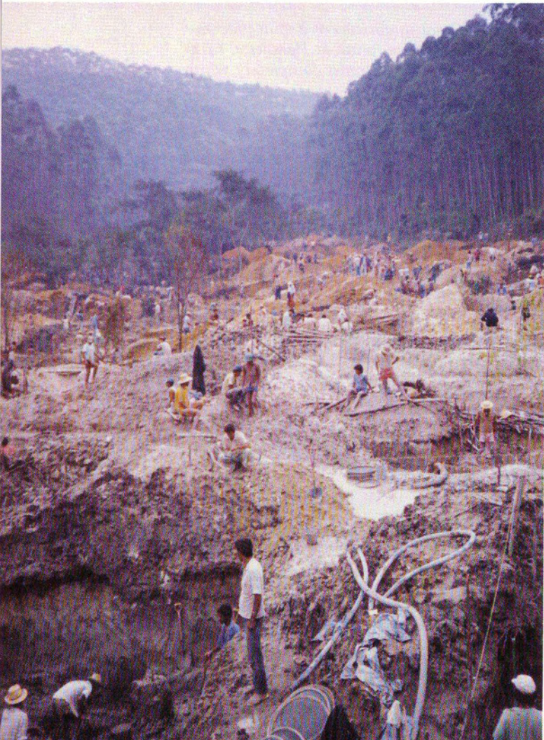
Figure 15. Pumps were required to rid most of the pits of water at Hematita. Note also the many circular screens, which the miners use to wash the gravels in their search for the gem alexandrites. Photo by Agenor Tavares.
