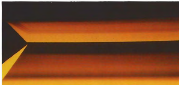
Figure 5. The "umbrella effect" characteristic of cyclotron-treated diamonds is evident as a line of darker color parallel to the culet (here, at the top of photo) in this emerald-cut diamond. Magnified 30 \times .
