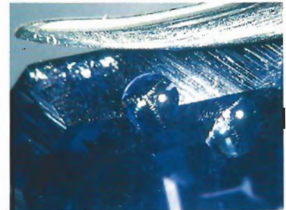
Figure 16. Drops of methylene iodide on a faceted needle-filled natural sapphire can produce a star effect. Magnified 10x.
