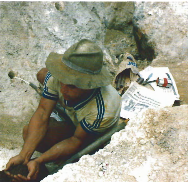
Figure 7. Large granite boulders often block access to the top gem-bearing layer at Barro Preto and must be blasted into smaller pieces for removal. Here the hole has already been drilled and the dynamite (note the sticks in back) with fuse has been put in place. The miner puts newspaper on top of the dynamite to protect the charge and then packs it with soil so that the rock will break uniformly. Photo by Henry Kennedy.
