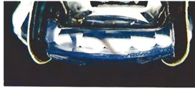
Figure 19. Brown color zoning is a rare occurrence in heat-treated sapphire. Magnified 10X.
