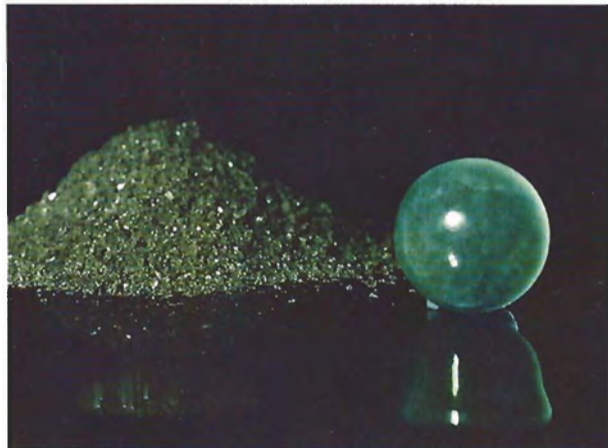
Figure 5. The crushed glass on the left was used as starting material in some of the synthesis experiments, and is shown here with one of the synthetic jadeite disks that resulted. Photo courtesy of the General Electric Company.
