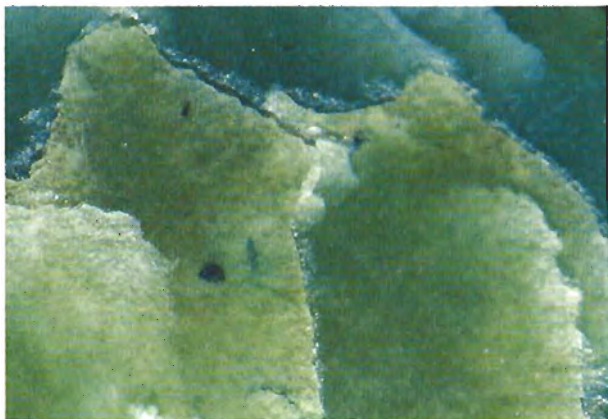
Figure 10. This view of the upper surface of one of the synthetic jadeite cabochons (no. 4) shows the broken edges of several of the thin layers that make up the material. Reflected light, magnified 20×. Photomicrograph by John Koivula.
