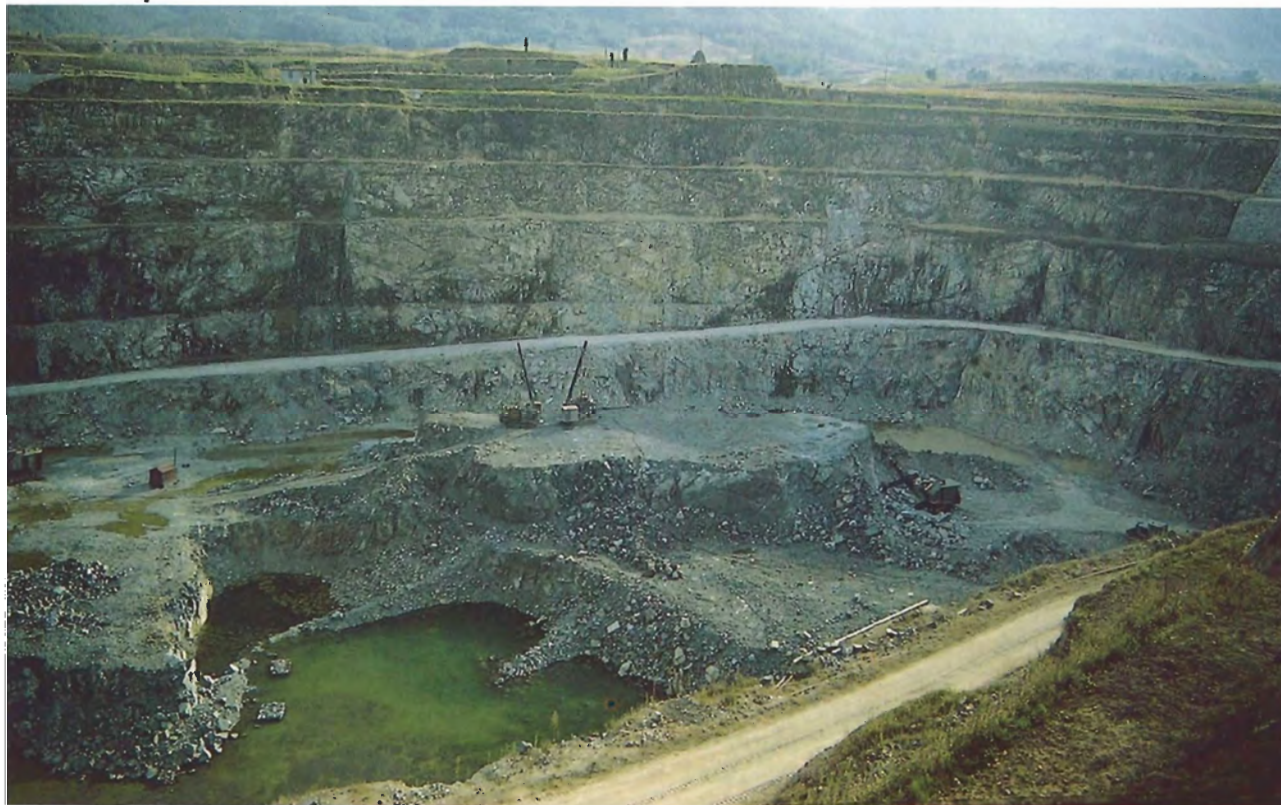
Figure 3. A view looking east in the bottom of the Victory No. 1 open-pit mine. The smaller of two kimberlite pipes is apparent and is being mined using power shovels.
