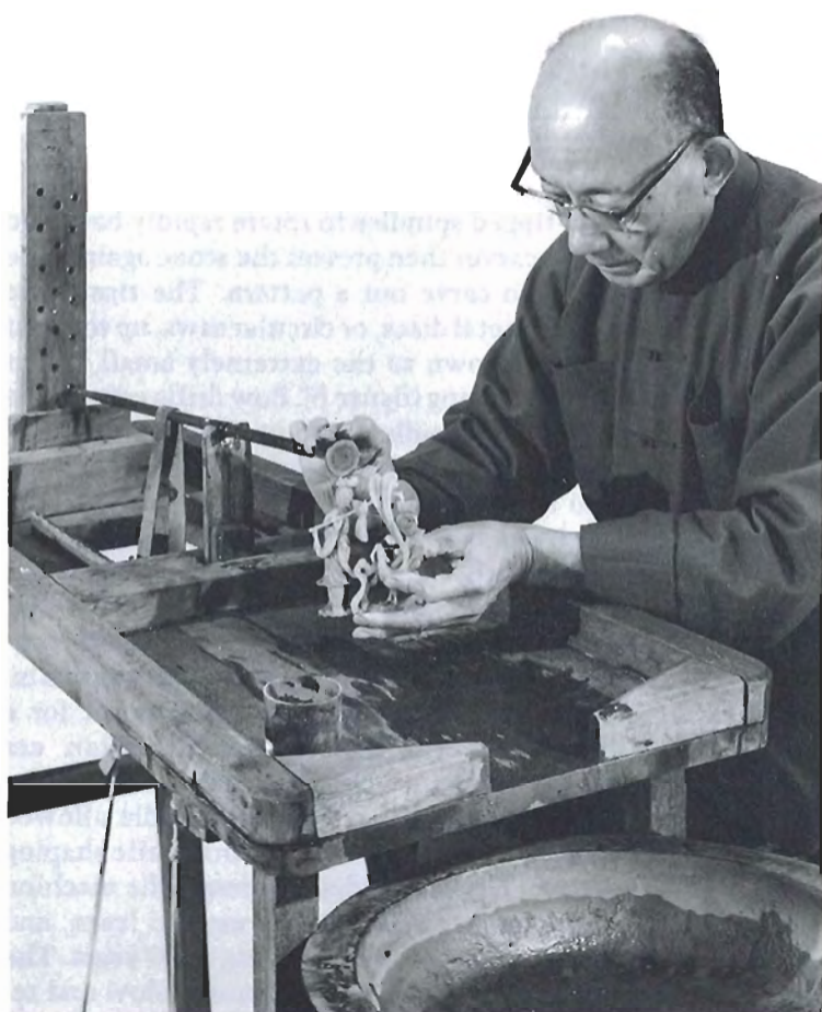
Figure 6. Through feedback from the pedals and his hands, the carver can exercise the control necessary to produce delicate carvings. Photo © Harold & Erica Van Pelt.
