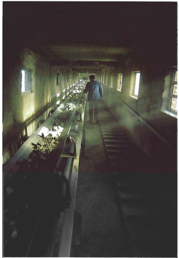
Figure 9. After initial crushing, the kimberlite ore is taken by conveyor belt through another series of crushing and screening, to break the ore further for treatment in the rotary washing pans.
