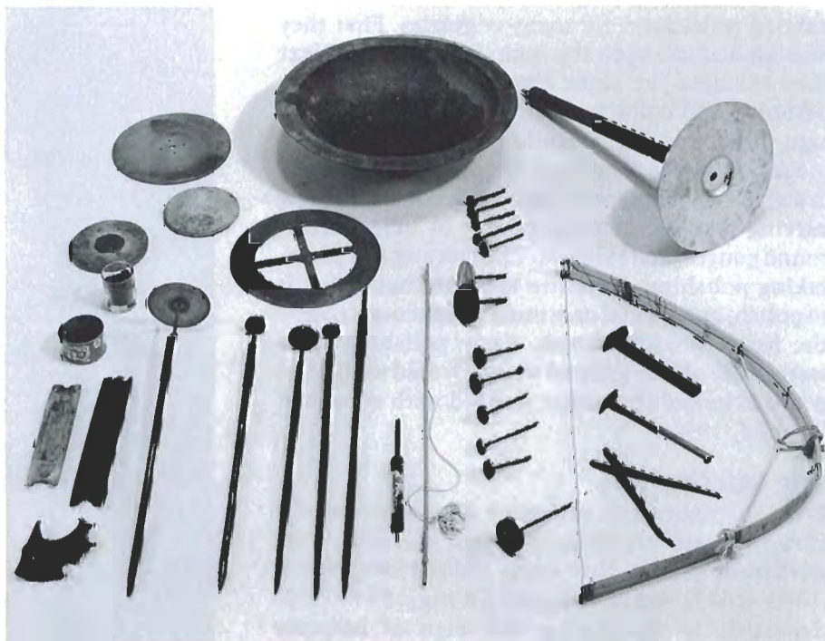
Figure 5. These tools of the Chinese master carver are used in conjunction with the treadle machine shown in figure 4. Photo © Harold & Erica Van Pelt.
