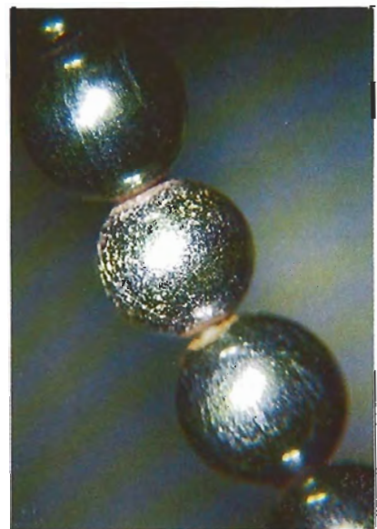
Figure 10. Pitted surface and banded structure on 4-mm magnetic hematite beads.
