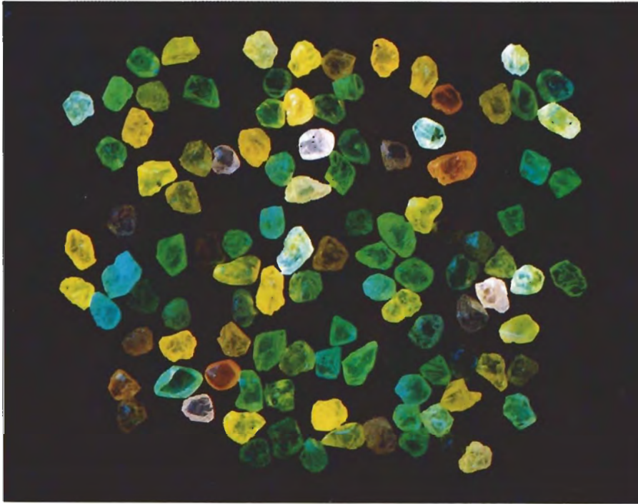
Figure 6. Luminescence produced in rough stones selected from a batch of gem-quality brown diamonds. Long-wave ultraviolet radiation (365 nm) was used to excite the luminescence.
