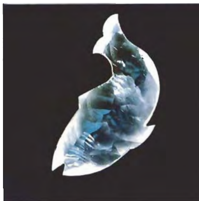
Figure 2. Carved fish-shaped diamond. The stone weighs 2.87 ct and measures 18.38 mm × 8.95 mm × 2.26 mm thick.
