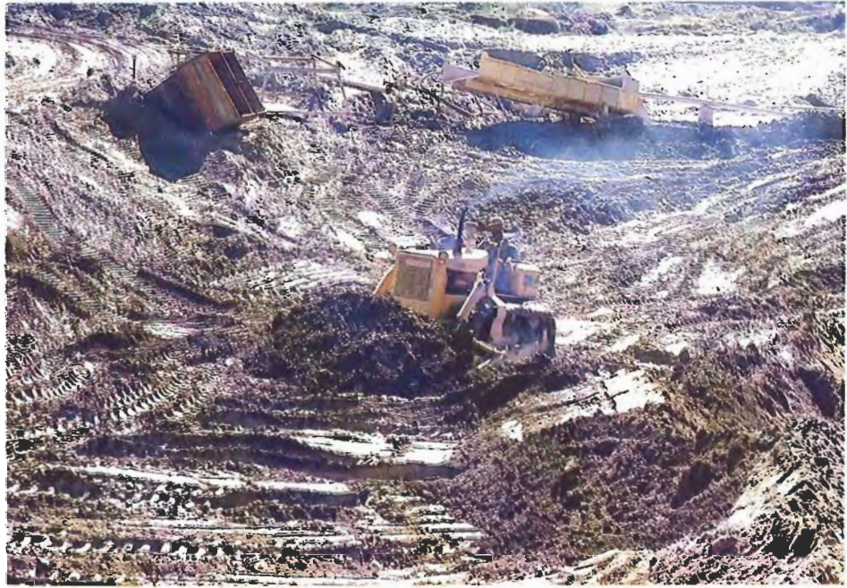
Figure 4. Large earth-moving equipment initially strips away the deeply weathered country rock, which is now essentially a lateritic clay that contains remnant pockets of kaolinite and topaz.
