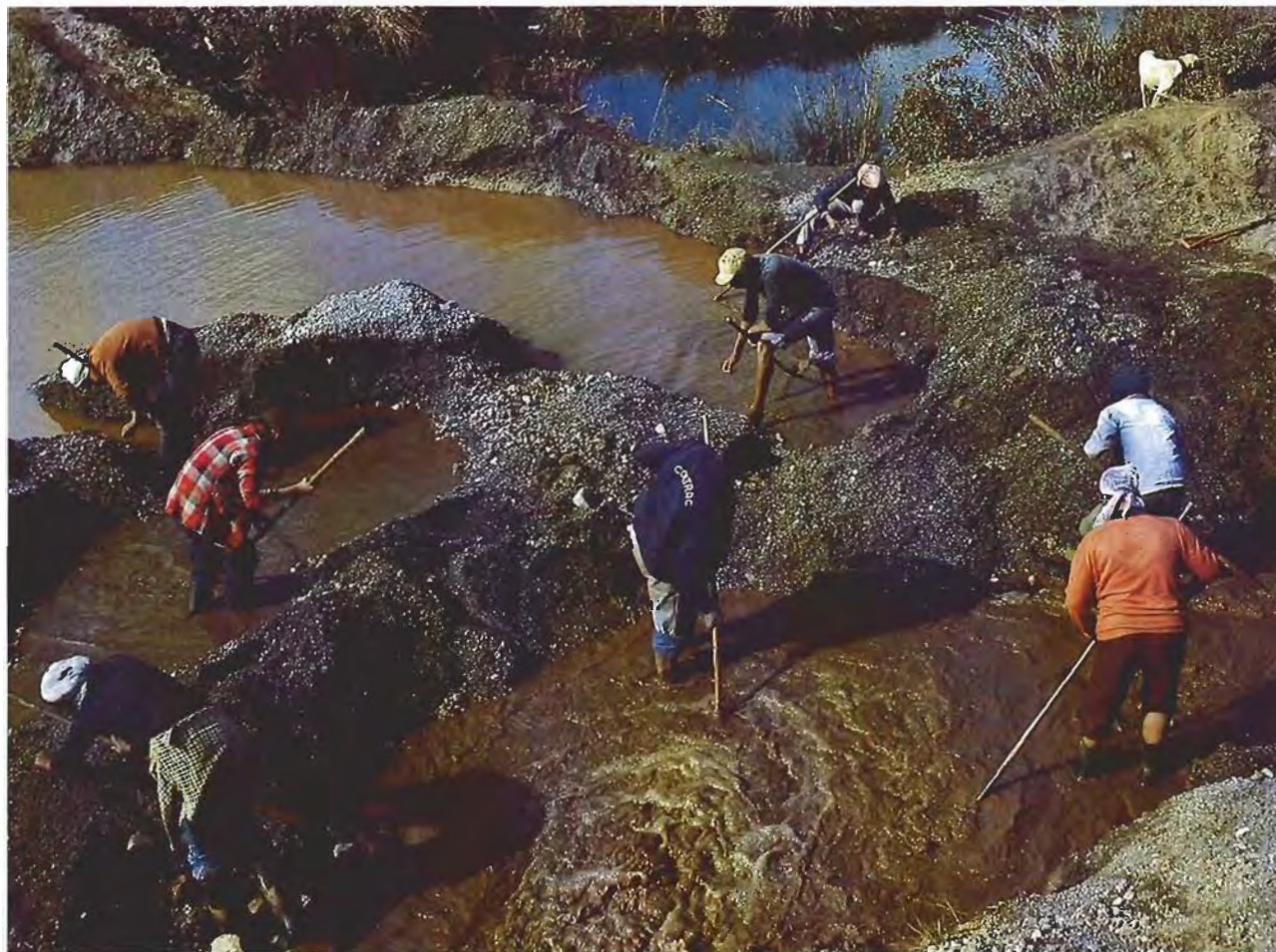
Figure 8. Garimpeiros work with simple sieves below the main mining operation at Capão in hopes of recovering an overlooked topaz. Photo by D. Vincent Manson.
