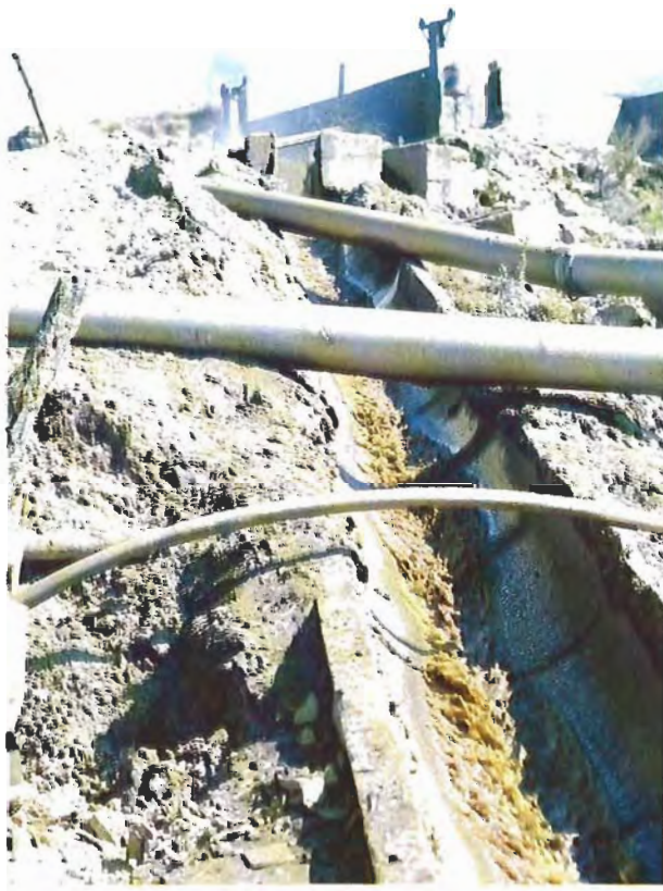
Figure 5. High-pressure water cannons put the topaz-bearing clay into solution so that the "heavies" can be separated from the lighter clays. The slurry is then washed down a concrete sluice to a concrete apron below.
