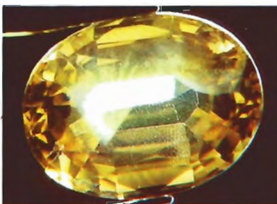
Figure 15. Light yellow natural sapphire after heat treatment. It was reported to be subject to fading. Magnified 12x.
