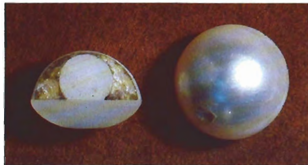
Figure 7. This section of an assembled cultured blister pearl (called a Mabe) clearly shows the four parts of which this product is composed.
