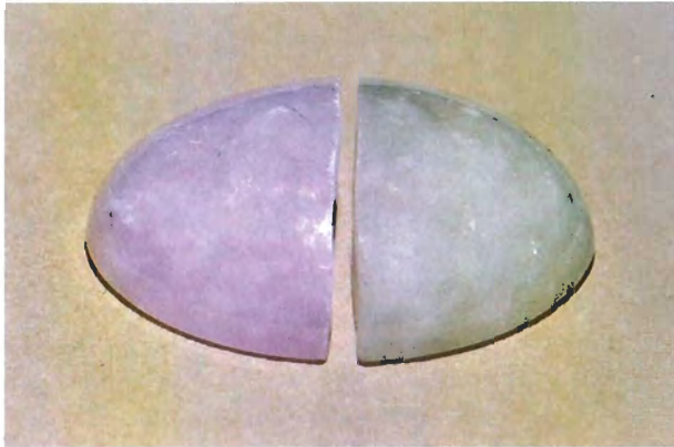
Figure 3. An example of heat bleaching. The unheated control half is on the left, and the heat-bleached half of the same stone is on the right (GIA collection no. 3661).
