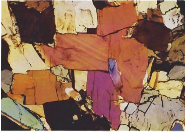
Figure 2. A thin section of jadeite shows many interlocking granular crystals. Magnified 100 \times . Photograph courtesy of the Smithsonian Institution, NMNH 94303.
