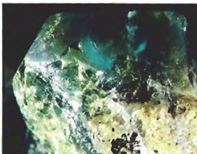
Figure 5. Mica flakes mixed into epoxy give a more natural appearance to the fake emerald crystal pictured in figures 3 and 4. Magnified 6x.
