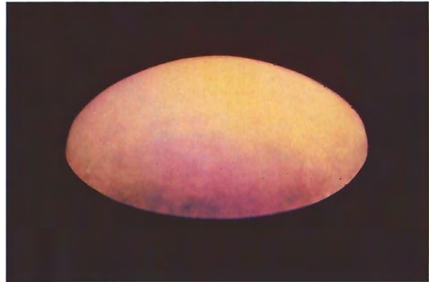
Figure 4. The strong orange long-wave fluorescence of a color-treated lavender jadeite (GIA collection no. 3654).
