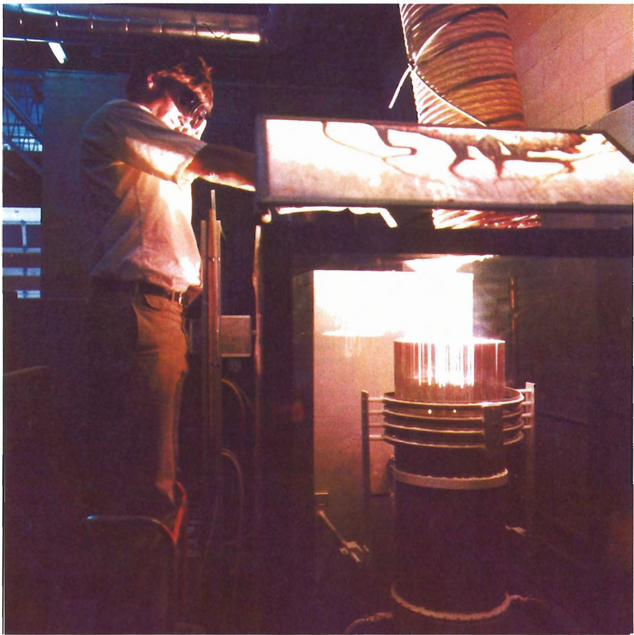
Figure 1. A large skull-melting apparatus being operated by George Bramhall. Courtesy of the Ceres Corp., Waltham, MA.
