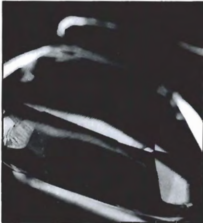
Figure 21. Curved striae and "fingerprint" inclusions in synthetic ruby. Magnified 30x.
