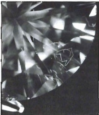
Figure 8. Irregular tube-like inclusions in a diamond. Magnified 18×.
