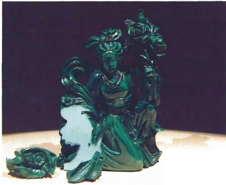
Figure 17. Damaged malachite carving showing separation between bedding planes; 2.5 cm × 7.5 cm × 10.5 cm high.
