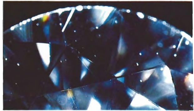
Figure 9. GGG often has rounded facet junctions because it has a hardness of only 6½. Magnified 40×.
