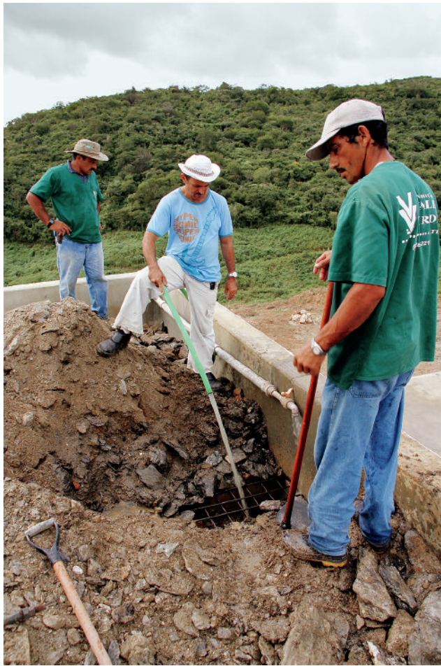
Figure 7. A basic processing plant has been used onsite to wash and sort the mined material in search of emeralds. Photos by J. C. Zwaan.
