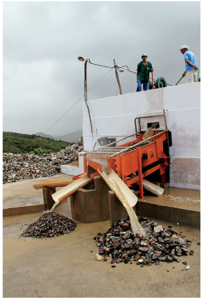
Figure 7. A basic processing plant has been used onsite to wash and sort the mined material in search of emeralds. Photos by J. C. Zwaan.
