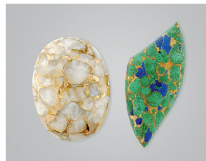
Figure 10. These 76.63 ct oval and 34.53 ct freeform cabochons proved to be manufactured composites that contain artificial metallic veining.
