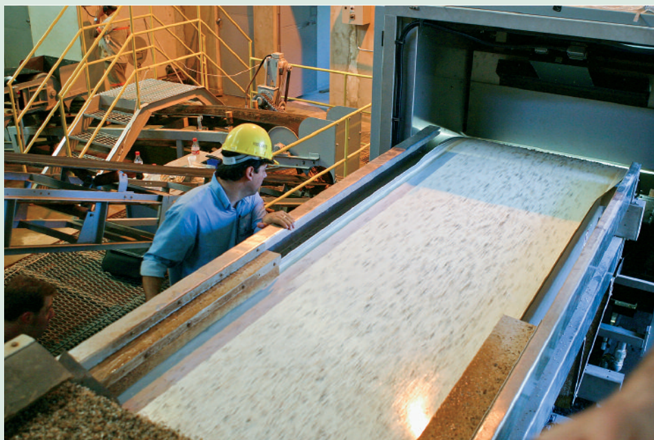
Figure 2. A conveyor belt brings ore into the optical sorter at Belmont for the CCD cameras to scan. Photo by Eric Welch.
