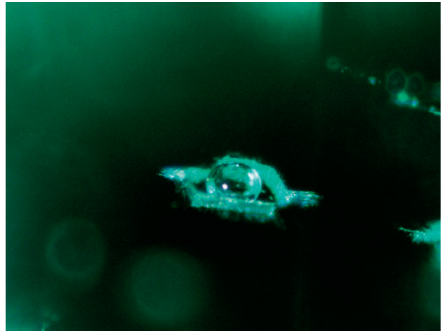
Figure 12. Raman microspectroscopy showed the presence of CO 2 within large gas bubbles in hexagonal-shaped negative crystals. Photomicrograph by J. C. Zwaan; image width 0.8 mm.
