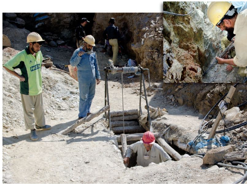
Figure 28. The mine manager at the Mingora emerald deposit climbs down the shaft to inspect production. The hand-powered windlass behind him is used for moving equipment and mined material in and out of the shaft. A pneumatic jackhammer is used to break up the emerald-bearing schist (see inset). Photos by A. Lucas.
