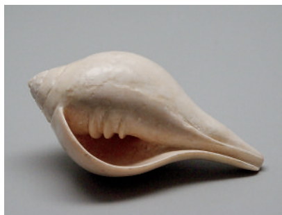
Figure 16. This specimen (13.2 cm long) proved to consist of a natural shell that contained a filler material and was covered by an unidentified artificial coating.
