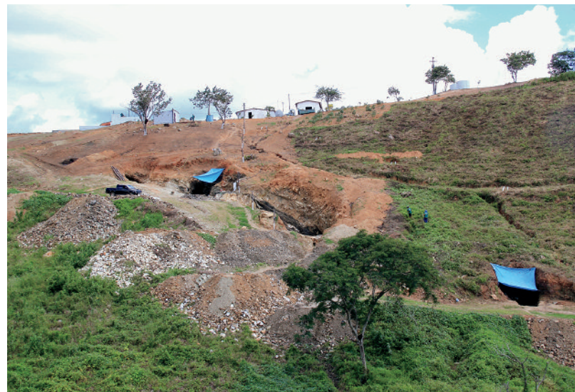
Figure 6. This overview of the emerald mining area shows small pits and adits along the ultramafic/granitic gneiss contact. Photo by J. C. Zwaan.
