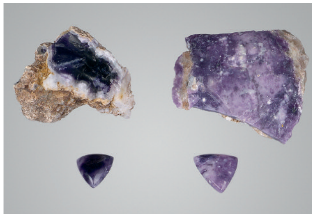
Figure 8. These samples of purple common opal are colored by fluorite inclusions. The rough pieces, which weigh 116 and 130 g, are shown with 13.98 and 15.24 ct cabochons. Photo by C. D. Mengason.
