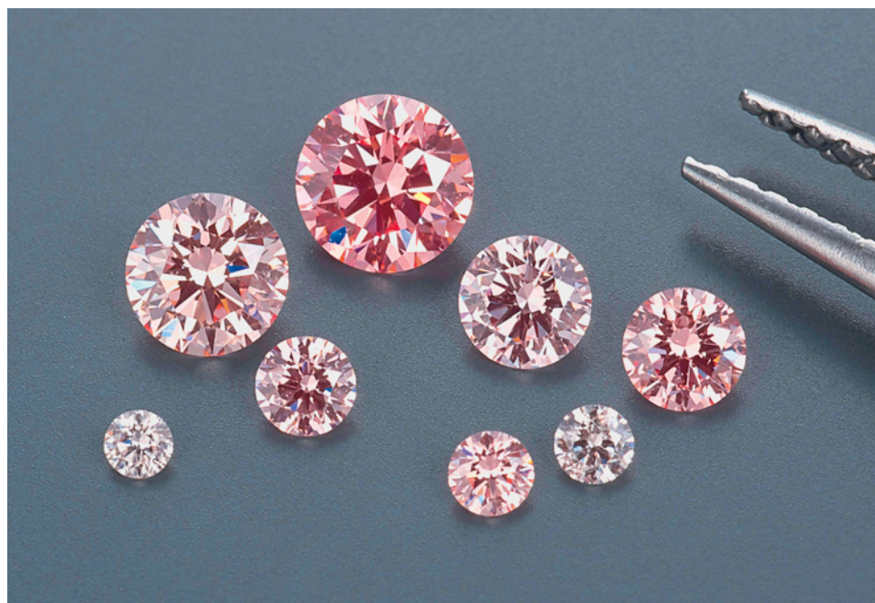
Figure 22. These eight representative samples of treated-color pink CVD synthetic diamonds range from 0.01 to 0.25 ct. Photo by M. Sasahara.
