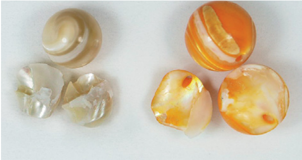
Figure 29. When some of the shell beads were broken open, the pale-colored ones (left, 7 mm in diameter) did not show any features indicative of dyeing. However, the orange beads on the right had color concentrations in fractures, along the drill holes, and in some areas near their rims. Photo by Jun Su.
