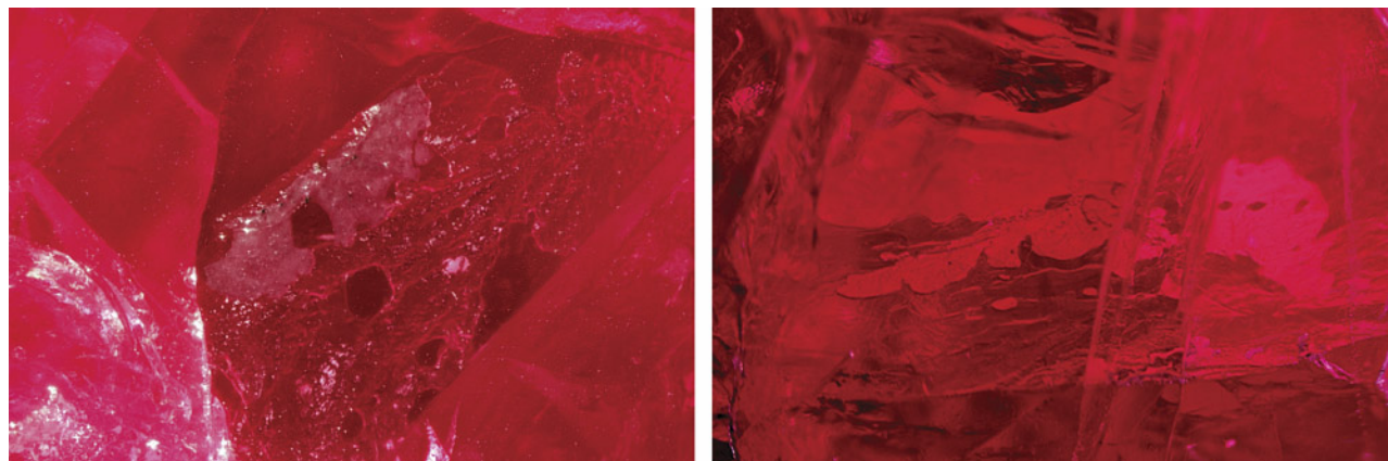
Figure 29. A fracture with whitish filler (left) and trapped air pockets (right). Fields of view 1.58 mm (left) and 2.90 mm (right).
