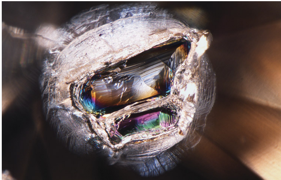
Figure 4. This iridescent ferropericlasite crystal with a stress halo measuring approximately 0.7 mm was trapped inside a light brown diamond. Photomicrograph by Kyaw Soe Moe; field of view 1.58 mm.
