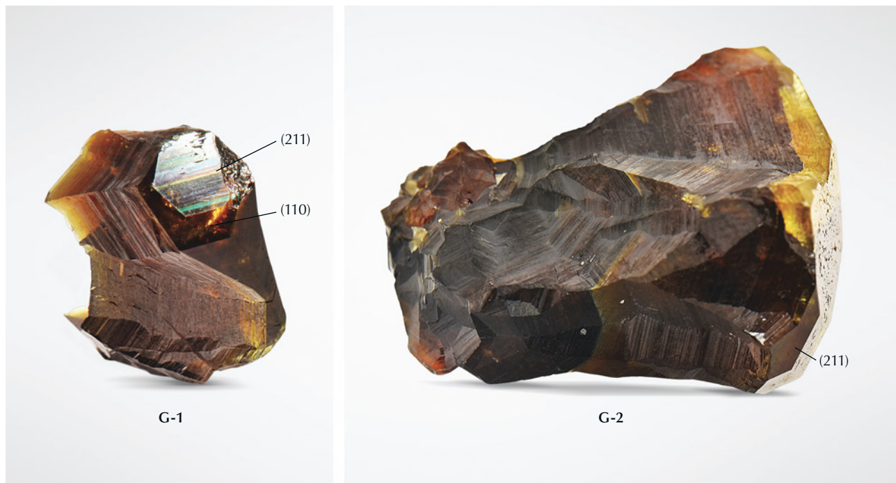
Figure 5. Iridescent andradite samples (25 ct and 125 ct) from the Lindong area of Inner Mongolia, China. As shown in the left photo, sample G-1 displays iridescence on the (211) plane but not on the (110) plane. Photos by Jiuchang Yang.
