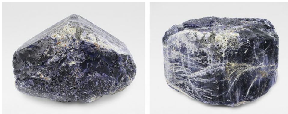
Figure 7. Large, euhedral cordierite crystal containing facetable and cabochon-quality sections. Note the deformation-induced fractures visible on prism faces in the photo on the right. The crystal measures 11.3 cm wide. Photos by Philippe Belley.
