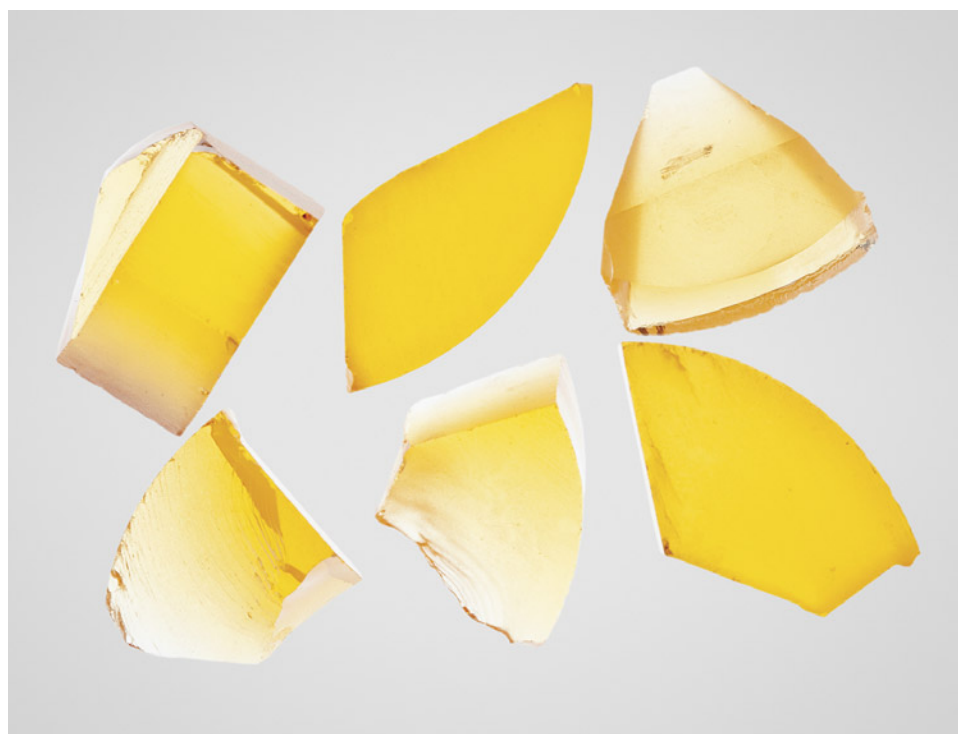
Figure 28. Synthetic sapphire colored only by the h^{\bullet}\text{-Fe}^{3+} chromophore. The three thickest sections are 12 mm thick. Photo by John L. Emmett.
