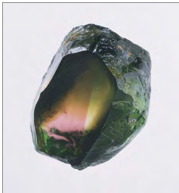
Figure 7. Microprobe analyses across the primary color zones—pink and green—in this Lundazi tourmaline nodule showed higher Bi contents in the pink core. Courtesy of Marc Sarosi; photo © GIA and Tino Hammid.
