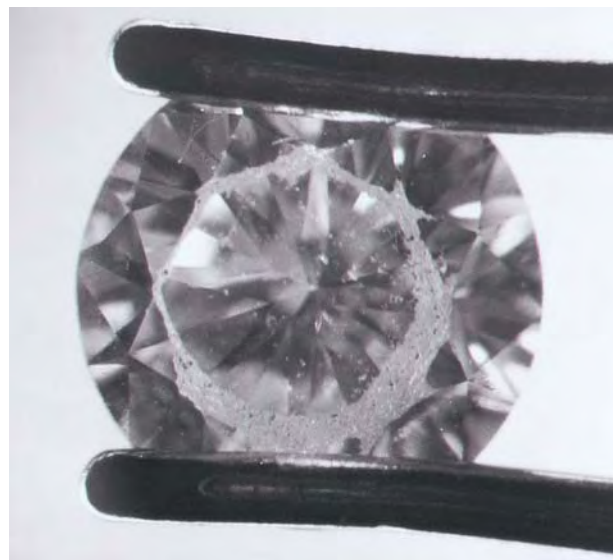
Figure 1. Note the extreme and uneven wear on this diamond (about 4.5 mm in diameter), which was the centerpiece of a brooch in which all the diamonds showed similar abrasion. Photo by Bernard Lasnier.
