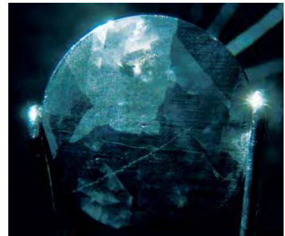
Figure 2. Fiber-optic illumination revealed the aggregate nature of the cabochons shown in figure 1, as seen here through the base of one of them. Magnified 15 \times .
