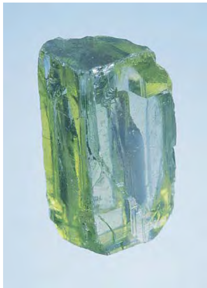
Figure 10. The shape of this 115.32 ct piece of rough synthetic periclase was dictated by well-developed cubic cleavage.
