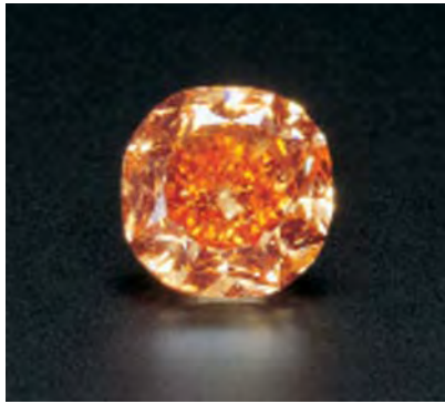
Figure 3. This 5.54 ct Fancy Vivid orange diamond is rare for its intensity of color. Diamonds in the orange hue range are typically darker, less saturated, and often modified by brown.
