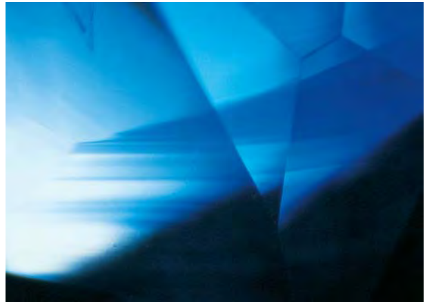
Figure 27. Planar color zoning is commonly visible at some angles within benitoite. The color zones appear curved in this 0.81 ct stone, because of refraction through adjacent facets. Shadow-like internal graining bounds and truncates the color zones, and is visible as the stone is tilted from side to side. Darkfield illumination, magnified 15 \times ; photomicrograph by John I. Koivula.
