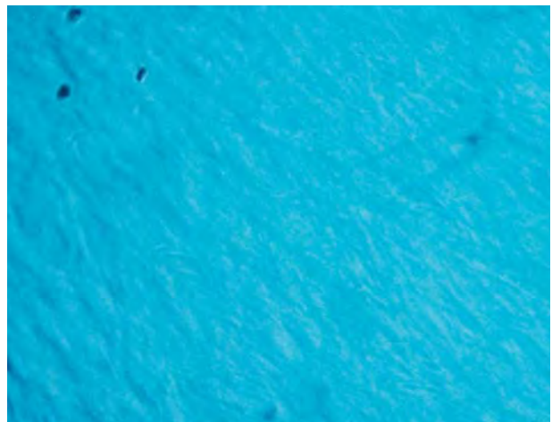
Figure 16. Swirl-like and chevron patterns were commonly seen in the Tairus synthetic green-to-greenish blue sapphires. Immersed in methylene iodide, magnified 100 \times ; photomicrograph by S. Z. Smirnov.
