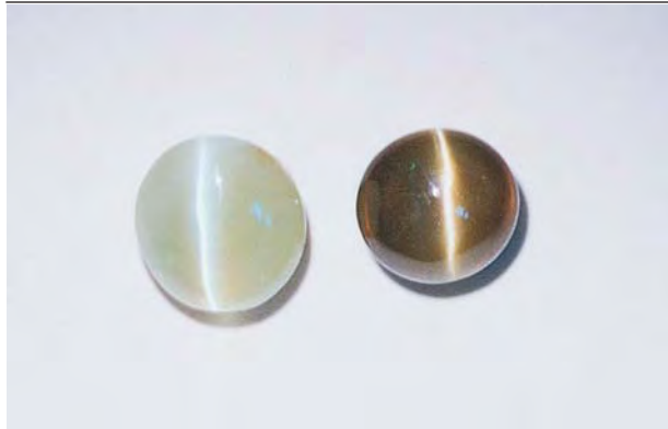
Figure 2. Material similar to the pale green cat's-eye chrysoberyl on the left was irradiated to produce the 3.5 ct radioactive dark brown cat's-eye chrysoberyl on the right. Photo courtesy of Kenneth Scarratt.
