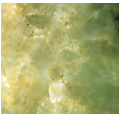
Figure 9. Jadeite “phantom” crystals, with translucent green cores and near-colorless rims, were seen with low magnification in this carved lid. The center crystal measures about 0.5 mm across.
