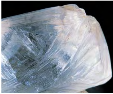
Figure 15. The shape, orientation, and raised relief of the "trigons" on this fashioned topaz do not reproduce the appearance of actual trigons on diamond crystals. Magnified 5x.
