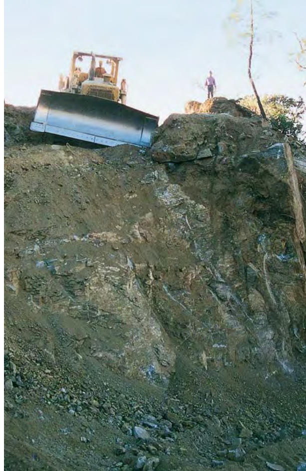
Figure 12. The Junnila claim was excavated with heavy equipment in 1995. Benitoite was recovered from the narrow, vertical zone of resistant blueschist that is visible here beneath the slender pine tree. Photo by William Larson.
