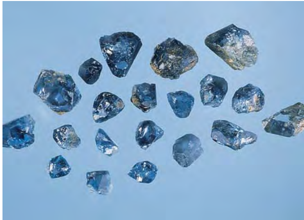
Figure 18. Rough benitoite gem nodules and crystal fragments, such as these, are removed from the gravitational separation jig by hand. The largest stone on the upper right is 1.0 cm wide. Photo by Maha DeMaggio.
