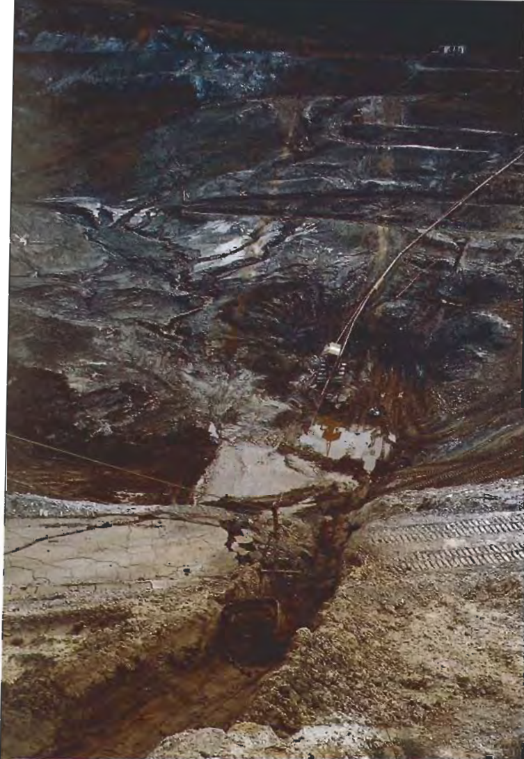
Figure 13. Draglines stretch across the large open pit at the Capão do Lana Imperial topaz mine. Large buckets suspended from the two lines scoop up the gem-bearing slurry from the bottom of the pit and drag it to the top for processing. Photo by Daniel A. Sauer, Amsterdam Sauer, Rio de Janeiro.
