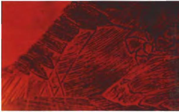
Figure 16. Interconnecting tubes of residual flux form characteristic "feathers" in this Russian flux-grown synthetic alexandrite. Immersion, magnified 40 \times .
