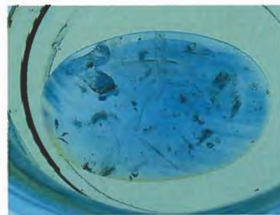
Figure 18. Immersion in methylene iodide revealed both natural color zoning and evidence of a "dye" in the sapphire in figure 17.
