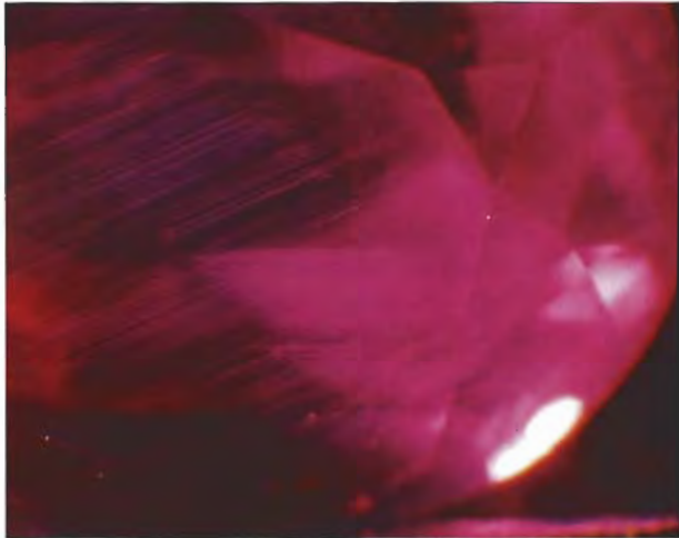
Figure 11. Unaltered rutile needles, concentrated more densely in bands parallel to subordinate negative d planes, provided proof of natural origin in the 1.34 ct ruby obtained in Vietnam. Oblique fiber-optic illumination, magnified 20 \times .
