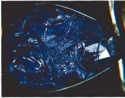
Figure 19. This quench-crackled natural sapphire owes its color to diffusion treatment. Magnified 10 \times .
