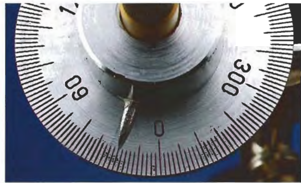
Figure 8. By rotating the stone holder until the growth features are sharply defined, the pointer will show the number of degrees, on the indicator dial, that the growth features are located from the optic-axis direction of the gemstone. The measurement of 20 shown here identifies a series of dipyramidal w ( 11\bar{2}1 ) planes, which are located characteristically at 20.1° from the optic-axis direction. Photo by Shane F. McClure.
