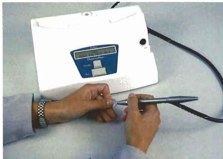
Figure 3. The DiamondSure probe can be removed from its mounting to test a diamond in a ring or other setting. Photo by M. J. Crowder.
