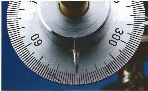
Figure 6. Once the optic axis has been successfully centered, before the stone is rotated to observe the growth features, the pointer must be positioned at the 0° mark on the indicator dial. Photo by Shane F. McClure.
