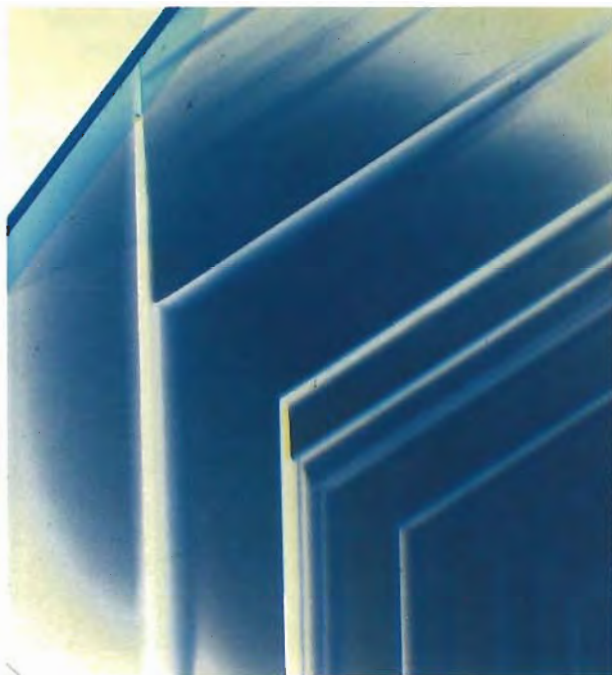
Figure 7. One of the most obvious ways to identify sharpened growth structures is through color zones, or bands, the thickness of which may fluctuate between consecutive periods of crystal growth. Shown here are broad blue color bands alternating with narrow colorless bands, parallel to dipyramidal v ( 44\bar{8}3 ) planes, in a sapphire from Kashmir. The vertical growth planes are at 15.4° from the optic axis direction, and the angle created at the junction of the v - v planes is 123°. Immersion, magnified 15×.
