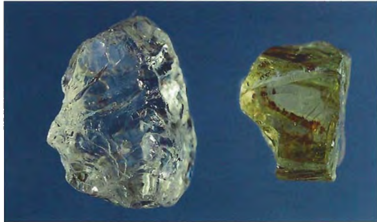
Figure 1. The most extreme change in color produced by this irradiation experiment was observed in these grossular specimens from Africa. Left: a 12-mm-long, 1.52-gram crystal (ROM specimen M40868) in its naturally yellowish gray state. Right: a similar specimen after exposure to 20 Mrads of ^{60}\text{Co} radiation.
