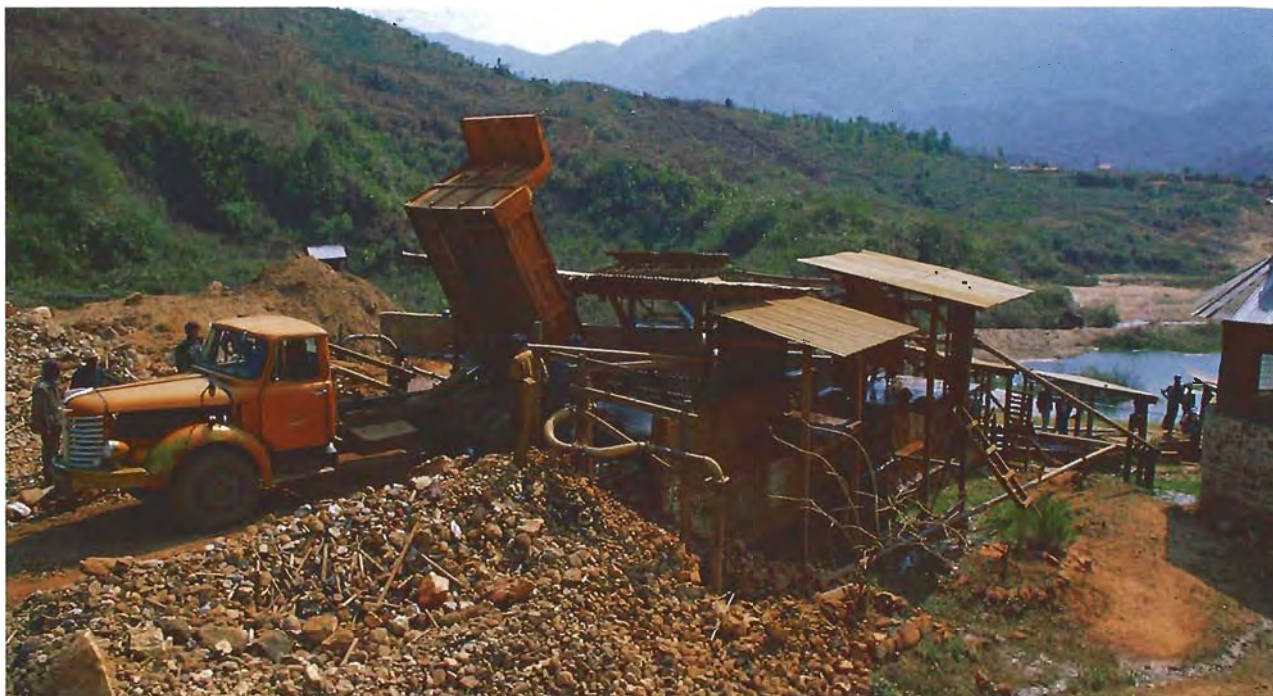
Figure 19. Processing at the Central Washing Plant begins with trucks unloading byon from MGE-operated mines onto a large metal grate. Photo by Robert E. Kane.
