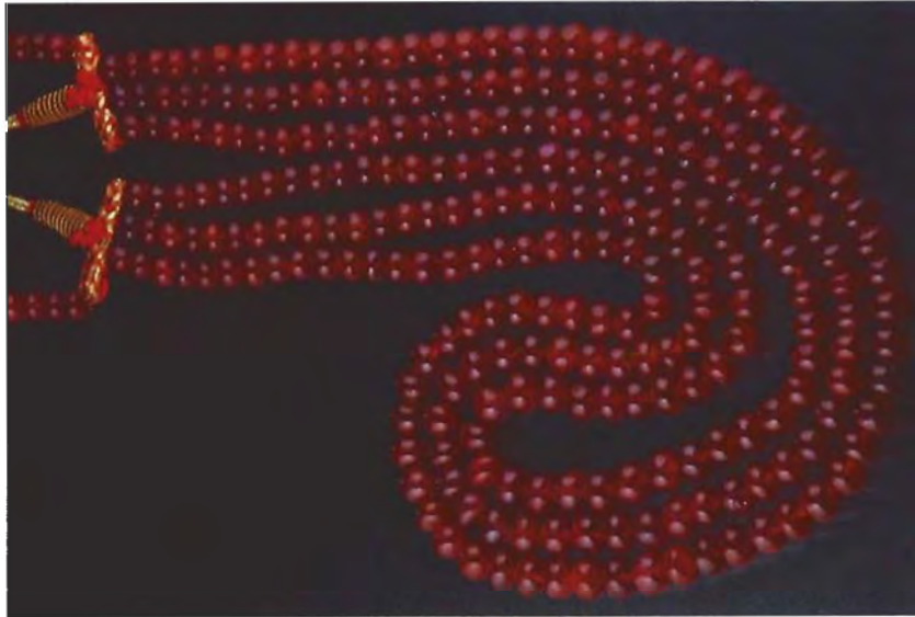
Figure 16. This multiple strand of 6- to 7-mm-diameter red beads was represented as natural ruby.
