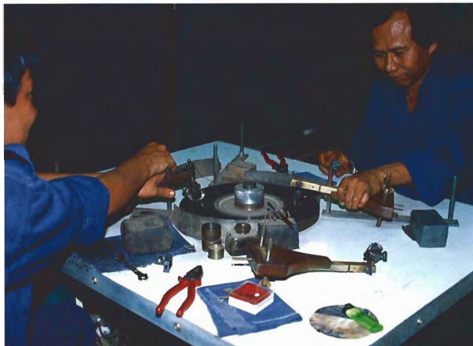
Figure 2. Diamonds from Myanmar deposits are faceted in Yangon at a cutting facility within the headquarters of the MGE. Here, two cutters work simultaneously on the same scaife. Photo by Robert C. Kammerling.
