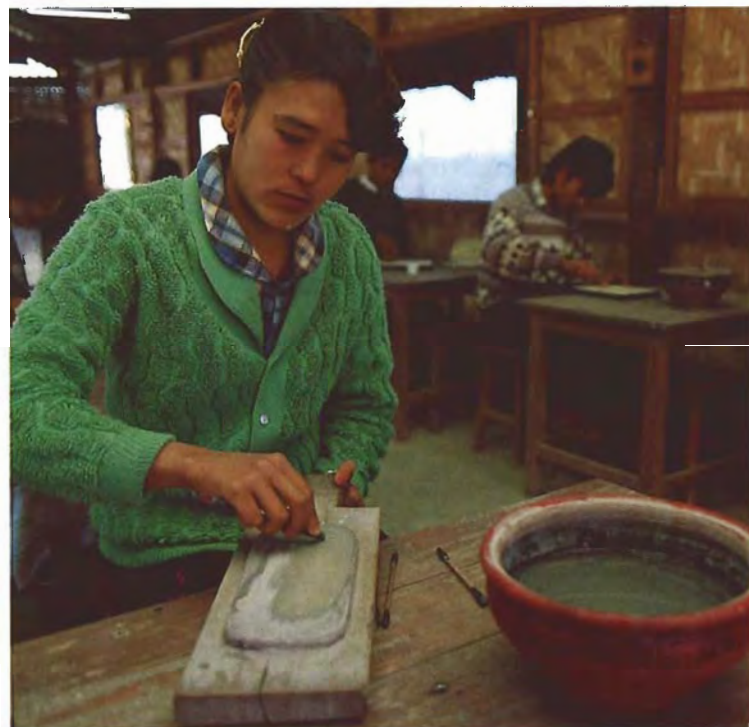
Figure 23. Some of the gem materials recovered from MGE-operated mines are fashioned at a small cutting factory/school within the MGE headquarters compound in Mogok. This young woman is using a traditional method—a wooden board coated with silicon carbide—to polish a sapphire cabochon. Photo by Robert E. Kane.
