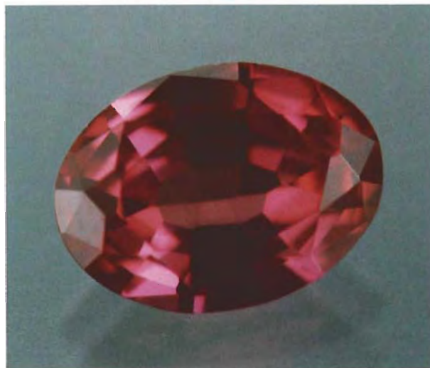
Figure 18. Czochralski-pulled synthetic alexandrite (here, 1.26 ct) is marketed under the trademark name Allexite. Photo by Maha Smith-DeMaggio.
