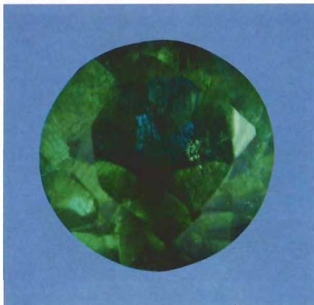
Figure 16. Faceup, this quench-cracked and green-dyed quartz (1.30 ct) makes an effective emerald imitation. I.R. spectroscopy determined that the dye was carried by an Opticon-like epoxy resin. Photo by Maha Smith-DeMaggio.
