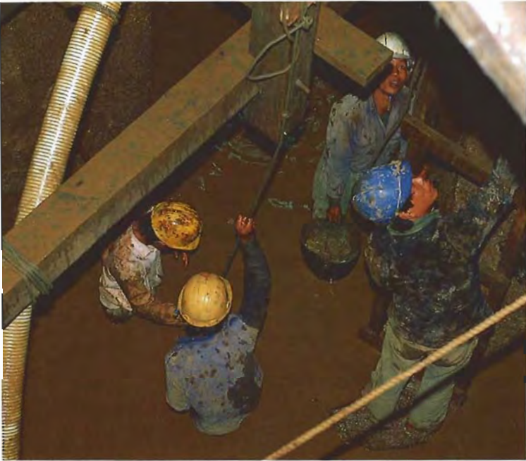
Figure 12. At the bottom of a 100-m-deep shaft at Than Ta Yar, workers use a hand winch to haul out buckets of waste material. The wide plastic tube to their left carries water and gem-bearing gravels to the surface for processing. Photo by Robert E. Kane.
