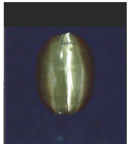
Figure 9. Strangely enough, two refractive indices were seen in this 2.76-ct cat’s-eye opal.
