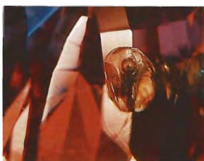
Figure 1. Note the gas bubble in the filled cavity (as seen through the table) on the pavilion of this natural alexandrite. Magnified 19\times .
