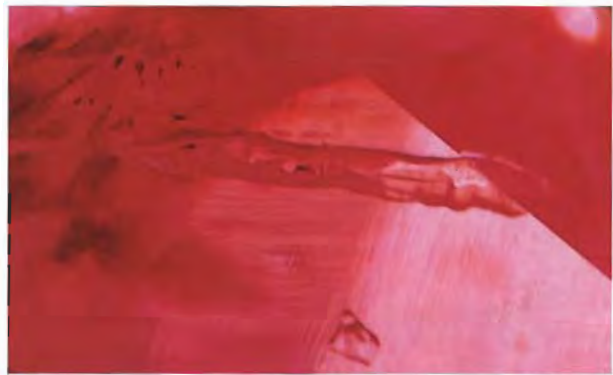
Figure 24. Several stones in this study contained unusual rod-like transparent crystals that proved to be an uncommon form of calcite. Darkfield and oblique fiber-optic illumination, magnified 40 \times ; photomicrograph by Robert E. Kane.
