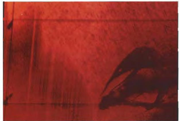
Figure 14. Extremely fine inclusions of rutile and/or other particles were concentrated in varying densities and were often, as here, confined to growth zones in the ruby. Immersion, magnified 65×; photomicrograph by K. Schmetzer.
