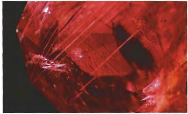
Figure 21. Needle-like inclusions of what are probably boehmite were observed in some stones along the junctions of laminated twinning planes. Oblique fiber-optic illumination, magnified 30 \times ; photomicrograph by Robert E. Kane.
