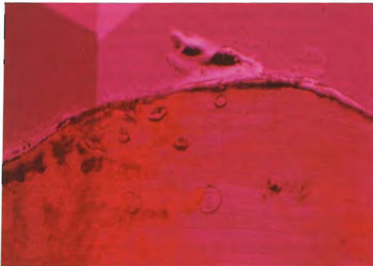
Figure 30. One sample was found to have been repaired. Note the glue layer and the misalignment of the reattached portion. Magnified 30 \times ; photomicrograph by John I. Koivula.
