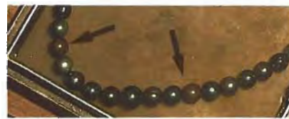
Figure 6. Immersed in film cleaner in preparation for X-radiography, the two dyed cultured pearls appear brown when compared to the others in this necklace.
