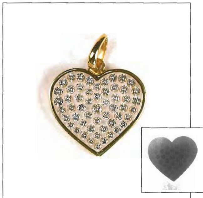
Figure 15. The diamonds in this pendant are mounted in a transparent colorless carbon-based polymer. The X-radiograph clearly shows the distinctive X-ray transparency of the diamonds. Pendant courtesy of Claar Brothers; photo by Nick DelRe. X-radiograph by Robert Crowningshield.
