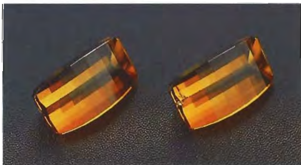
Figure 7. These two dravite tourmalines appear slightly brownish yellow when seen under incandescent (or fluorescent) lighting (left), but they become distinctly greenish yellow when illuminated simultaneously with incandescent and fluorescent lighting (right). Courtesy of Don Clary; photos by Robert Weldon.
