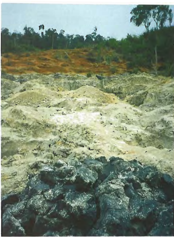
Figure 8. In many parts of the Quy Chau ruby-bearing district, the gem-bearing gravels can be reached only by removing layers of clay and kaolin. Here a pile of wet gray kaolin (foreground) that has just been removed lies next to mounds of dry white kaolin. In the back can be seen the clay-like soil that covers the surface of the region. Photo by C. Mora.
