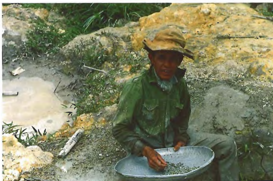
Figure 10. For the most part at Quy Chau, the miners wash the gravels by hand using rudimentary "pans" in their search for rubies and other gem materials. Photo by C. Mora.
