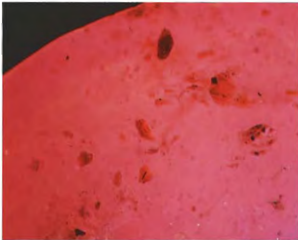
Figure 29. Brownish orange crystals of phlogopite mica were among the many solid inclusions found in these Vietnamese stones. Dark-field and oblique fiber-optic illumination, magnified 35 \times ; photomicrograph by Robert E. Kane.
