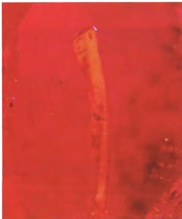
Figure 28. This unusual yellowish orange inclusion, consisting of the rare mineral nordstrandite, may be confused with flux found in Ramaura synthetic rubies. Darkfield and oblique fiber-optic illumination, magnified 30×; photomicrograph by Robert E. Kane.
