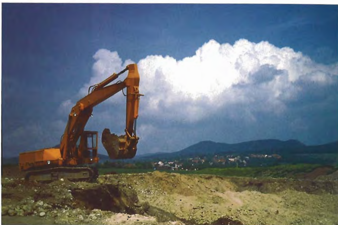
Figure 3. A power shovel is used to remove the overburden and garnetiferous gravels at Podsedice. In the background can be seen remnant pipes of Tertiary volcanism in the Bohemian Hills. Photo by J. Schlüter.
