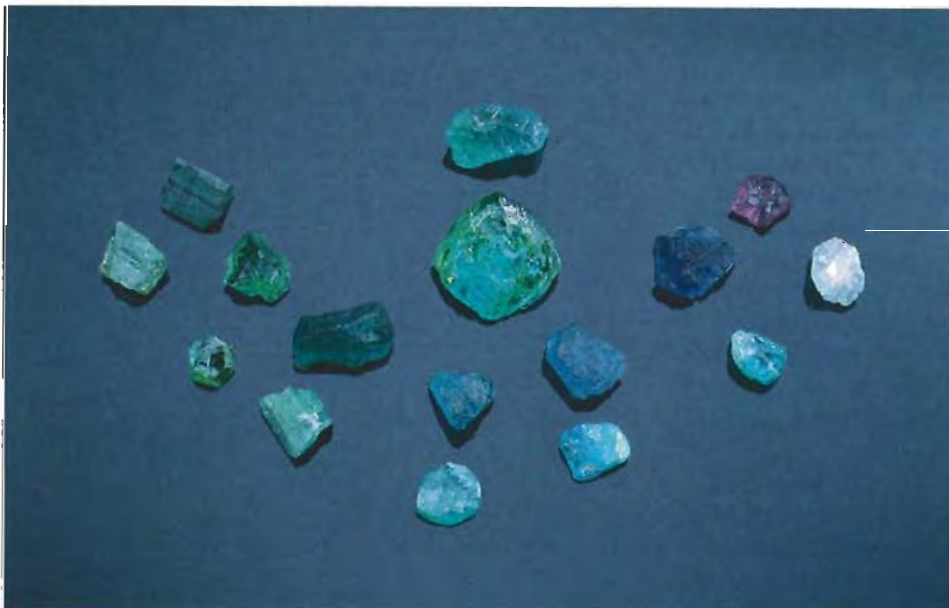
Figure 17. These pairs of Paraiba tourmaline fragments show the effect of heat treatment on this material. Originally, both specimens in each pair were the same color (with the range of colors chosen to represent those typical of this locality); the lower specimens were subsequently heat treated to illustrate the color change produced. As described in the text, heat treatment results in blue to green for virtually all colors of starting material. Photo by Robert Weldon.
