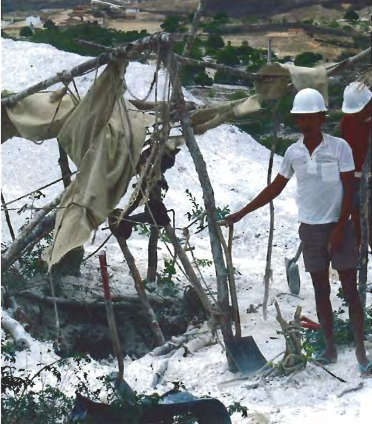
Figure 4. White clay (altered feldspar) can be seen surrounding the main shaft of the tourmaline mine on Serra da Frade. The village of São José da Batalha appears in the background. Vertical shafts and horizontal tunnels have been dug into the weathered pegmatite in search of gem tourmaline. Photo, taken August 1990, by Brian Cook.
