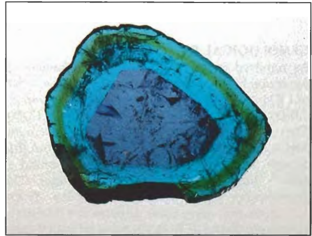
Figure 7. This 5.96-ct slice ( 15.20 \times 12.20 \times 3.28 mm) of Paraíba tourmaline is representative of the somewhat complex color zoning that appears in some crystals. This color zoning reflects changes in chemical composition as the tourmaline crystallized. Courtesy of The Gold Rush, Northridge, CA; photo by Shane McClure.
