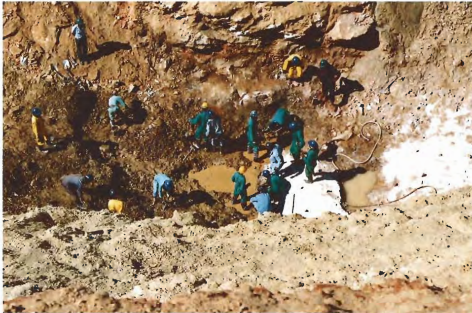
Figure 3. This view from the edge of the main pit at the Machingwe mine, southeastern Zimbabwe, shows miners at work recovering emeralds. The pegmatite structure (white area) has been followed downward 60 m. Photo © Tom Lee and Michael Smith.
