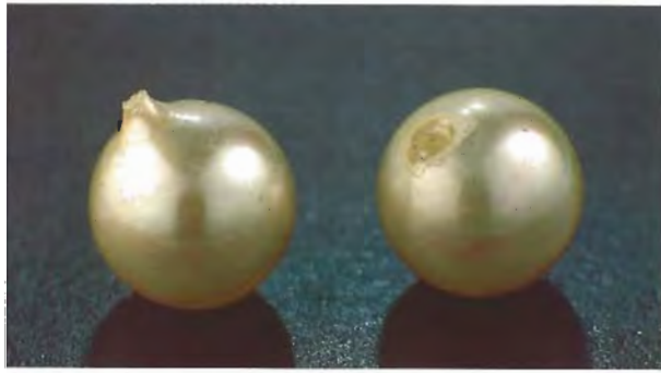
Figure 9. Once the final coating is dry, the tail-like accumulation of pearl essence (left) is trimmed by hand. This ensures a more perfect sphere (right). Photo by Robert Weldon.
