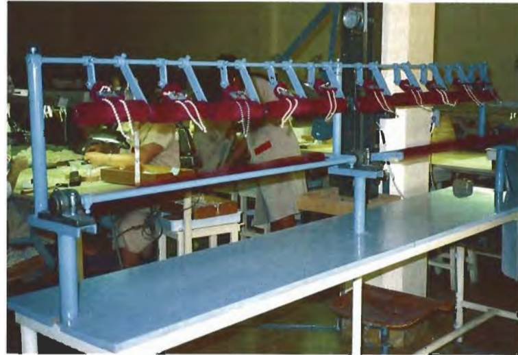
Figure 10. As a final step, selected strands of the finished Majorica beads are subjected to strenuous durability testing. Here, the strands are mounted on a special machine that literally "beats" them against a rotating bar to simulate years of wear. Photo by June Hanano.
