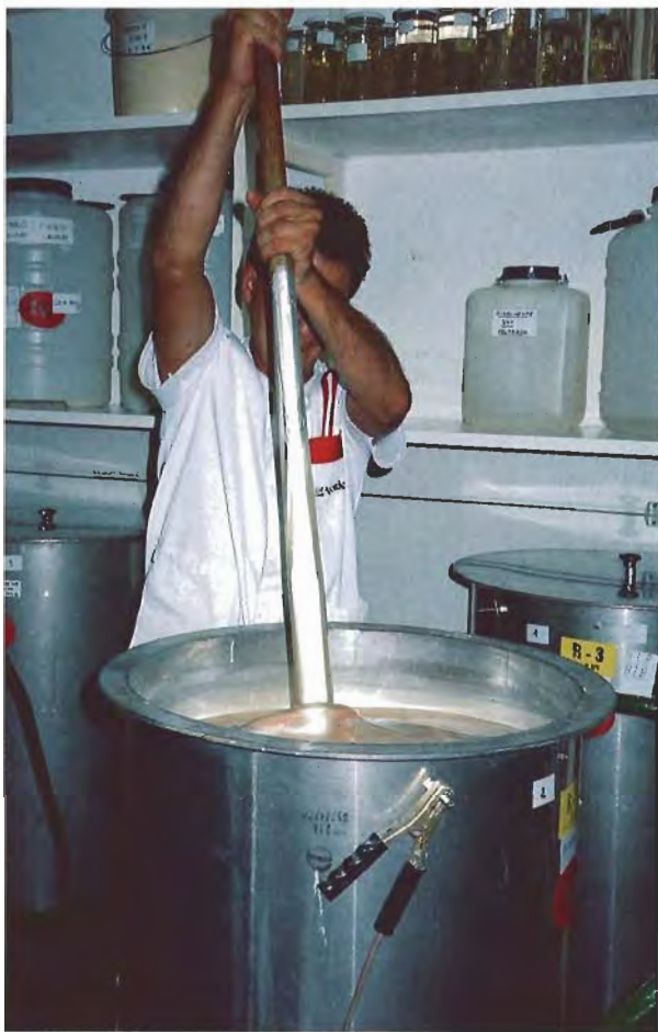
Figure 7. The iridescent material (“pearl essence”) used on the Majorica imitation pearl to simulate nacre is formed by mixing the guanine extracted from fish scales with binding and coloring agents. Photo by June Hanano.
