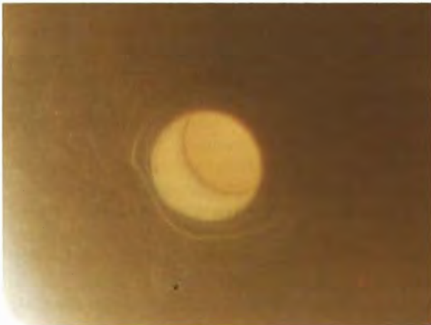
Figure 14. When examined with 10× magnification, the drill hole of a cultured pearl shows the outer nacreous layer separated from the mother-of-pearl nucleus by the slightly darker layer of conchiolin. Note also that the edges of the hole are sharp and well defined. Photomicrograph by John I. Koivula.
