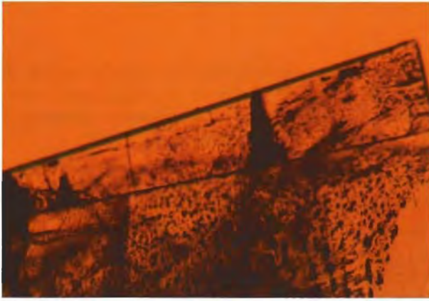
Figure 5. In the faceted sample of Russian hydrothermally grown synthetic aquamarine, "feathers" consisting of either liquid or two-phase inclusions are found in both the seed (above) as well as in the light blue portion (below). Immersion, magnified 40 \times .
