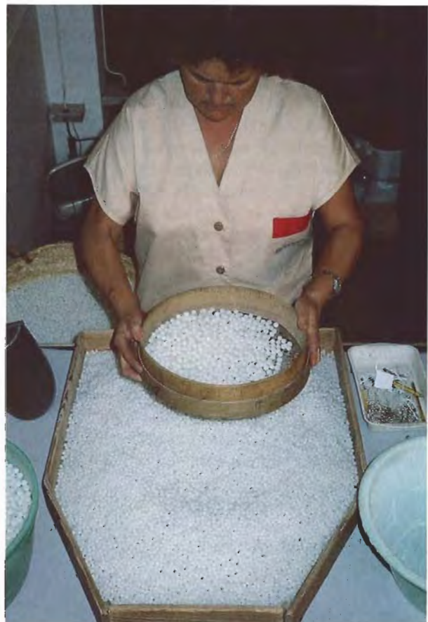
Figure 6. After the nuclei pass inspection, each "strand" is placed in an acid bath to remove the wire on which they were originally formed. Then, as shown here, the loose beads are sorted through sieves that place them into size categories with a tolerance of 0.2 mm. Photo by June Hanano.
