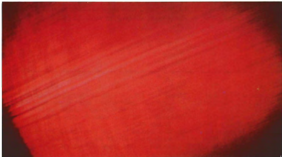
Figure 4. With the built-in iris diaphragm on the Gemolite microscope stage partially closed (over darkfield illumination) to create a shadowing effect in this cabochon-cut Inamori synthetic cat's-eye alexandrite, the unevenly spaced parallel growth features become more evident and reveal themselves as undulating rather than straight. Magnified 25x.
