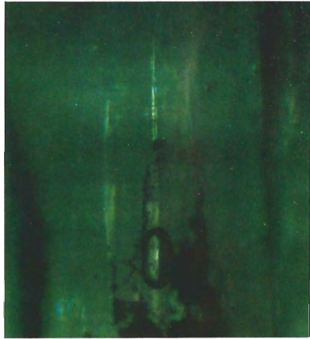
Figure 10. In this greatly enlarged two-phase inclusion, the large oval bubble that corroborates the second phase is probably in a glassy flux relic. The inclusion runs parallel to the c -axis of the host. Transmitted light, magnified 100 \times .
