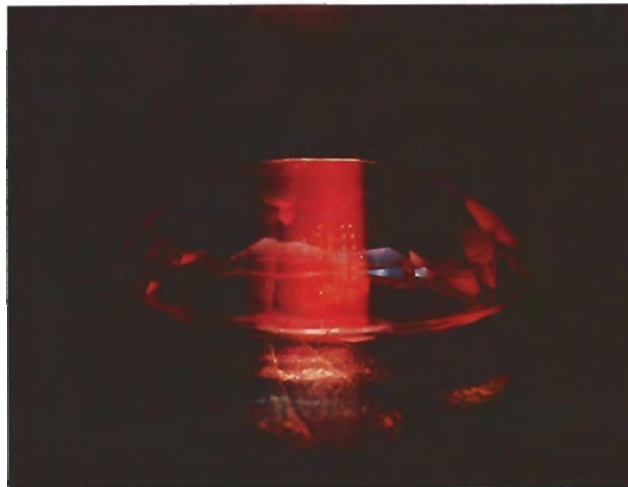
Figure 3. Transmission luminescence as seen over the strong light source from the opening of the iris diaphragm on the spectroscope unit. Left, Inamori synthetic cat's-eye alexandrite; right, natural alexandrite from Brazil. Photos by Shane McClure.
