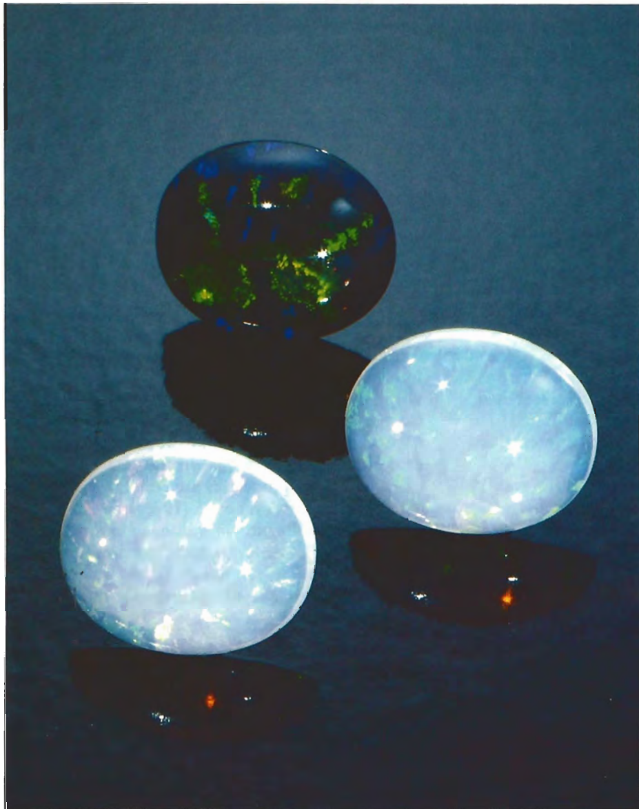
Figure 1. These three examples of Inamori Created Opal are produced by the Kyocera Corp. of Kyoto, Japan. The sample with the black body color weighs 3.96 ct and measures 10 × 12 mm. Photo © Tino Hammid.
