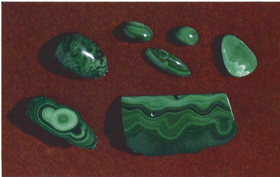
Figure 9. All of these polished samples of synthetic malachite show potential for use in jewelry, carving, or inlay. The cabochons range from 15 to 32 mm.
