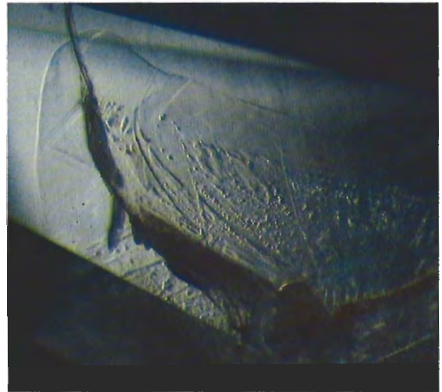
Figure 3. The inner surface of a filled cleavage plane in one of the diamonds examined at GIA shows the flowing rounded structures that appear to be typical of filling. Shadowed transmitted light, magnified 50×; photomicrograph by John I. Koivula.
