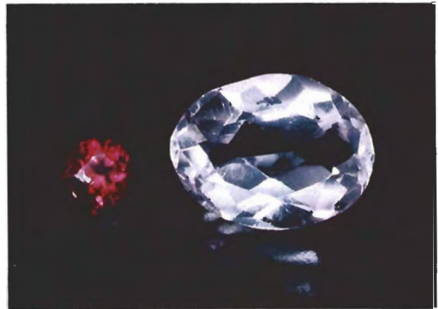
Figure 6. The difference in color intensity between a pink beryl (morganite) from Brazil, colored by \text{Mn}^{2+} , and a red beryl from Utah, colored by \text{Mn}^{3+} , illustrates the importance of the valence state of the coloring ion. Photo by Shane McClure.
