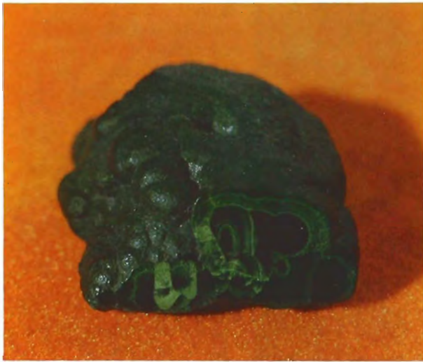
Figure 4. A bud-like texture is evident in this sample of synthetic malachite, which is cut parallel to the growth direction. Maximum length and width, 30 × 12 mm.
