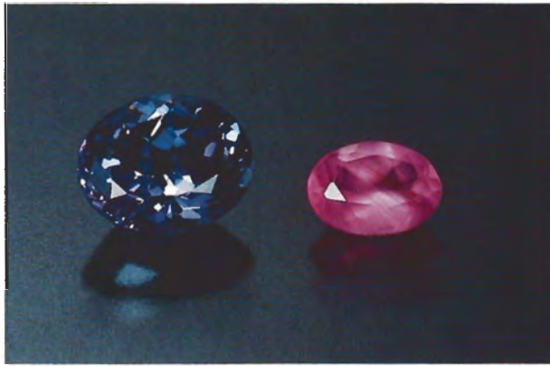
Figure 9. These two stones show the difference in color caused by a difference in coordination: \text{Co}^{2+} is in tetrahedral coordination in this blue spinel, and in octahedral coordination in the pink cobaltocalcite. Photo by Shane McClure.
