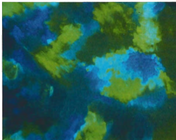
Figure 3. This Kyocera opal imitation with black body color shows the mosaic-like patterns with distinct boundaries between different "grains," as well as the pattern referred to as "lizard-skin," "chicken-wire," or "honeycomb" that is caused by the subdivision of each color "grain." This pattern is considered characteristic of man-made opal. Magnified 40×.
