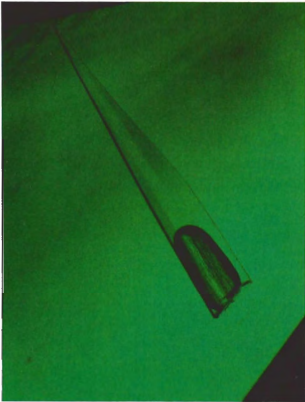
Figure 10. This large nail-head spicule in a Biron synthetic emerald consists of a cone-shaped void that is filled with a fluid and a gas bubble. Although not visible at this viewing angle, the spicule is capped by a poorly developed, ghost-like phenakite crystal. Dark-field illumination, magnified 50 \times .
