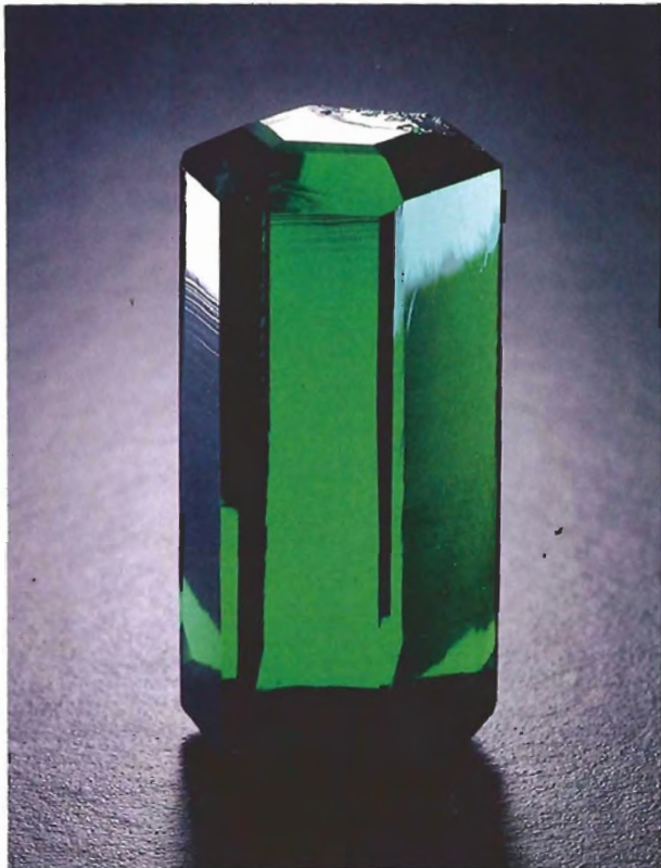
Figure 2. An exceptional example of the Biron hydrothermal synthetic emerald crystals grown in Western Australia. This crystal measures 3.50 cm long by 1.6 cm wide, and weighs 96.08 ct. Photo by Tino Hammid; © W. L. Cotton.
