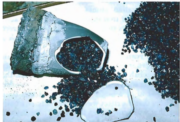
Figure 17. The inner crucible has been broken open after treatment of these Australian blue sapphires was completed.
