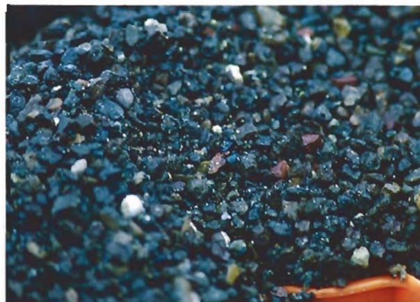
Figure 8. Fine concentrate after removal from the pulsator. Note the abundant black pleonaste.
