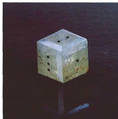
Figure 4. This 11.73-ct gambling die was fashioned from industrial-quality diamond and the "dots" subsequently inscribed by laser. It measures 9.29 x 9.28 x 9.12 mm.
