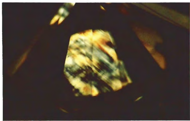
Figure 8. A 10× view inside the same stone as in figure 7, using polarized light, shows the typical banded or linear birefringence pattern that signifies internal strain in the diamond, coincidental with the grain lines.
