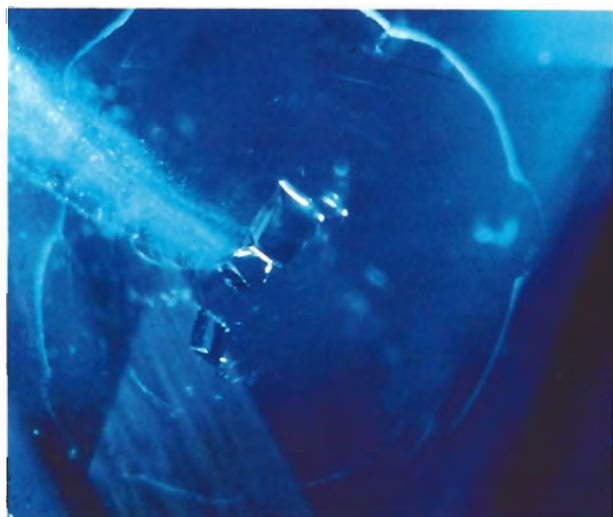
Figure 18. This colorless euhedral crystal surrounded by a tension halo and accompanied by a "comet tail" is a common inclusion in Australian blue sapphire. Photo by B. Scheos, Diamond Laboratory Services; magnified 40x.
