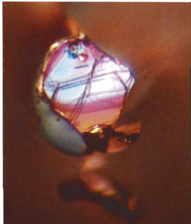
Figure 4. Phlogopite in taaffeite from Sri Lanka as observed with crossed polarizers. Magnified 25x.
