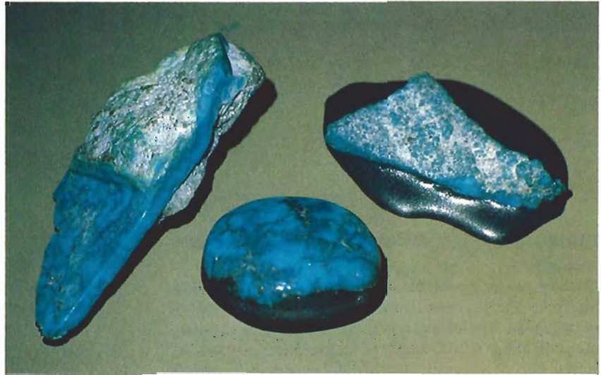
Figure 18. Top left: a thin layer of turquoise in matrix. Top right: turquoise backed by a metal-loaded epoxy cement. Center: finished backed cabochon.
