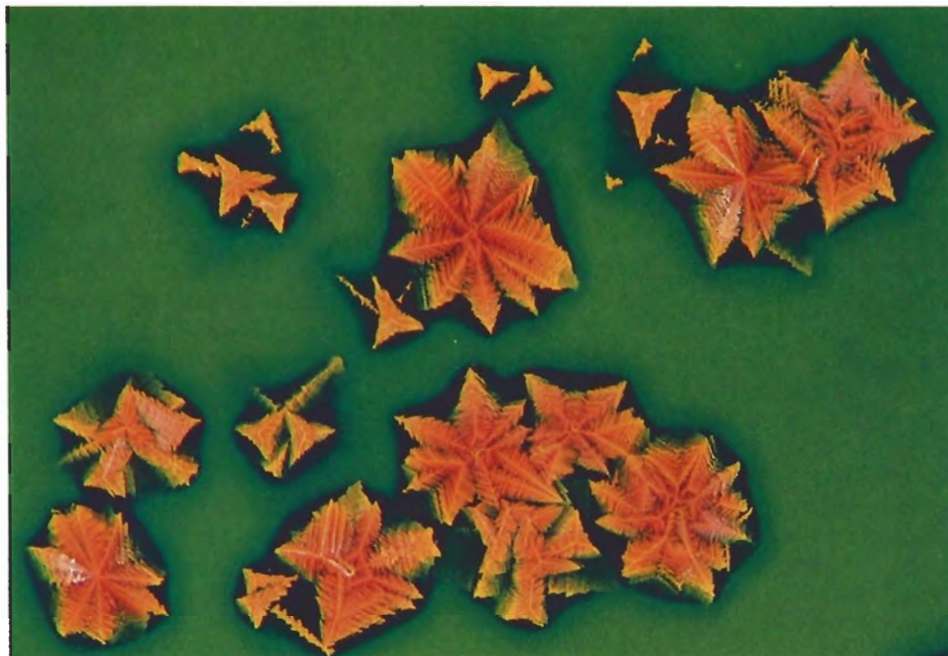
Figure 1. Dendritic areas of synthetic cuprite devitrification in Iimori's "Maple Stone" glass. Magnified 20x.
