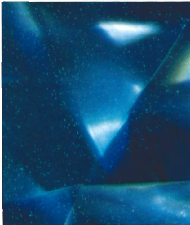
Figure 11. A cloud of tiny, whitish pinpoint inclusions in the faceted blue synthetic diamond. Dark-field and oblique illumination, magnified 50 \times .
