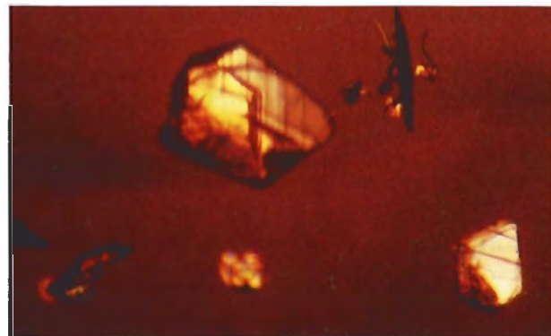
Figure 6. Muscovite mica observed in a taaffeite found in the Amerawewa gem area of Sri Lanka. Immersion microscope, magnified 40x.
