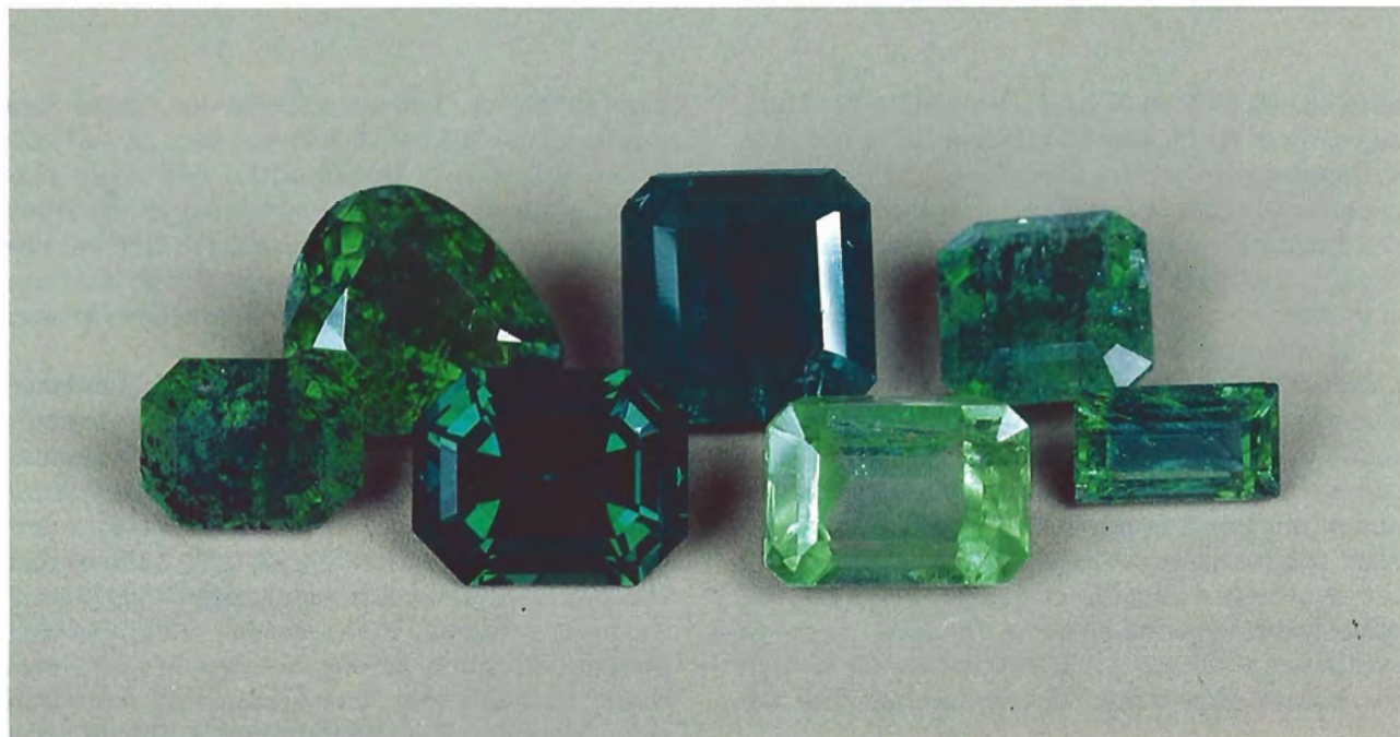
Figure 1. A representative sample of natural and synthetic emeralds from the study collection. The stones pictured range from 0.50 to 1.91 ct and originate from the following sources (left to right): Santa Terezinha de Goiás (Brazil), Lake Manyara (Tanzania), Biron (hydrothermally grown synthetic), Chatham (flux-grown synthetic), natural (country unknown), and two stones from Colombia (specific localities unknown). Photo by Michael Havstad.
