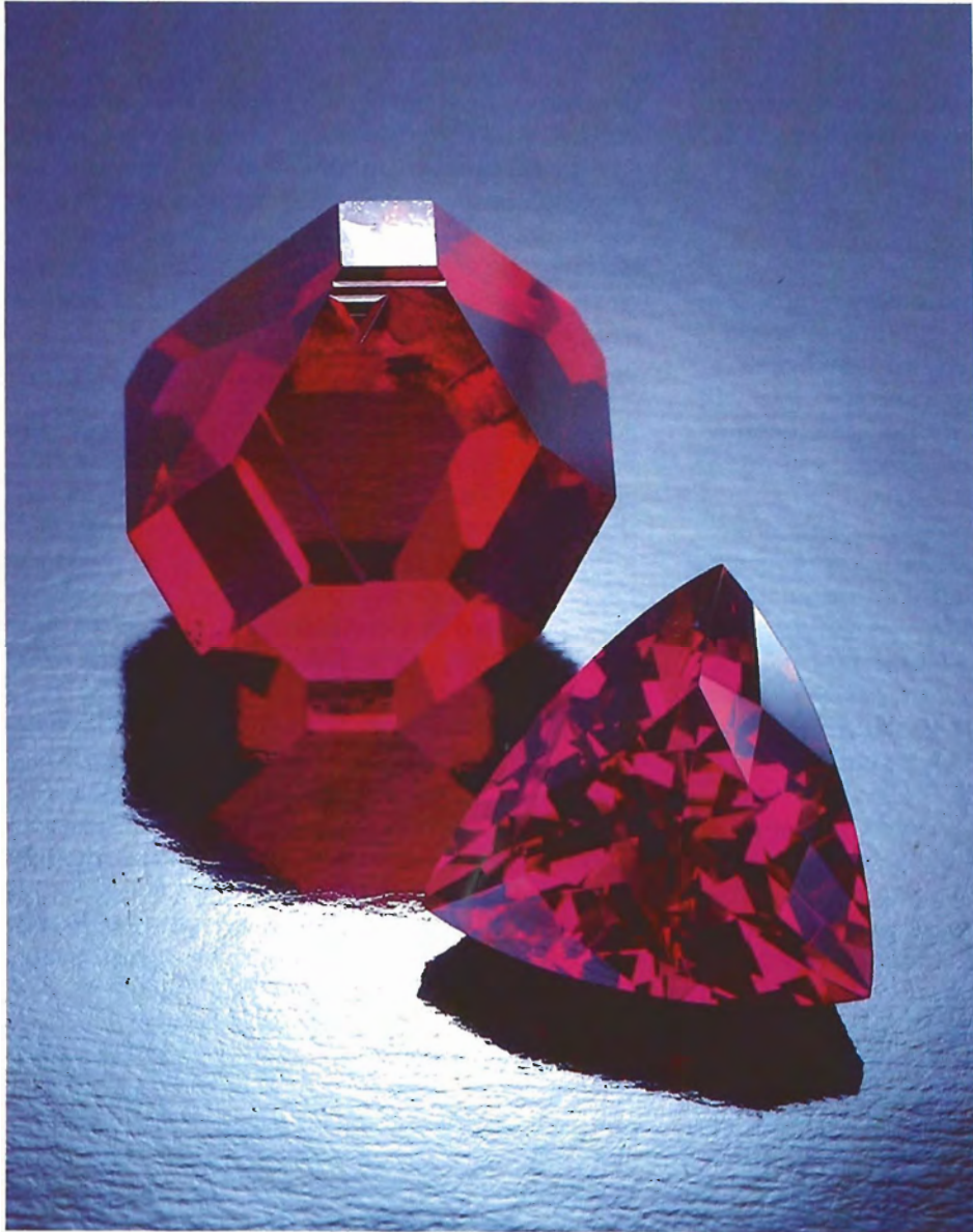
Figure 1. Ramaura synthetic rubies: the 8.77-ct uncut specimen is a rare example of a large, nearly equidimensional rhombohedral crystal; the faceted stone weighs 3.67 ct. Photo ©1983 Tino Hammid.
