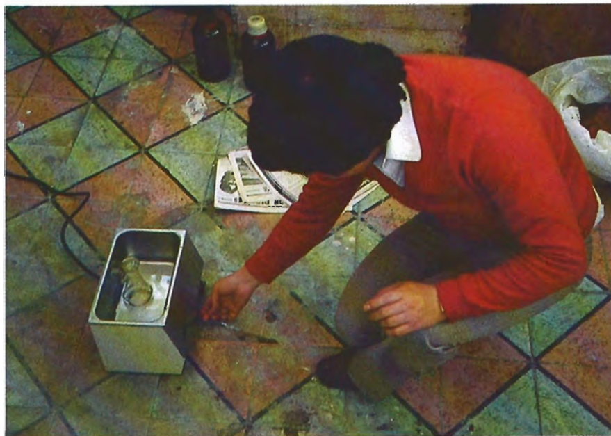
Figure 4. An ultrasonic cleaning tub is sometimes used to help the acid mixture penetrate and clean the emeralds. The cutting and polishing oxides left in the fracture openings would otherwise block the penetration of the oil.
