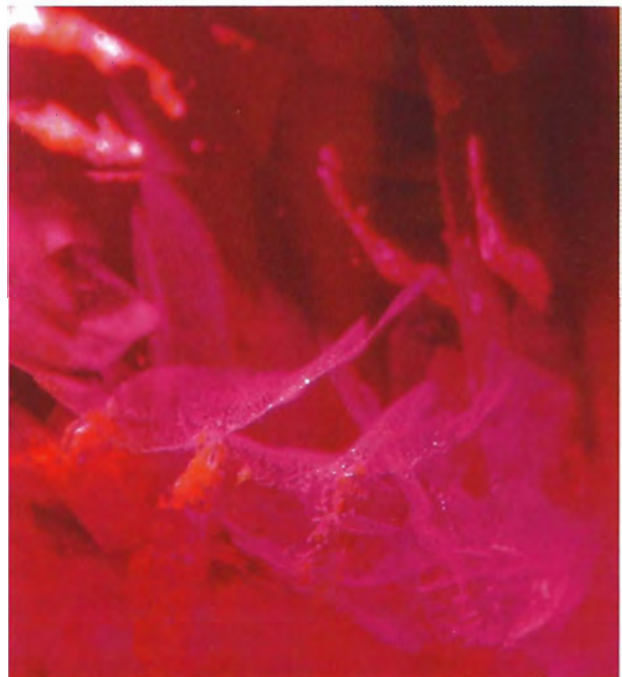
Figure 15. Orange-yellow flux globules interspersed among white, wispy flux "fingerprints" in a Ramaura synthetic ruby. Dark-field and oblique illumination, magnified 20 \times .
