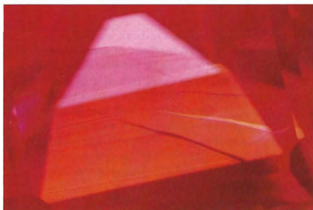
Figure 22. This Ramaura synthetic ruby is host to several different forms of growth features and color zoning. Dark-field illumination and shadowing, magnified 20 \times .
