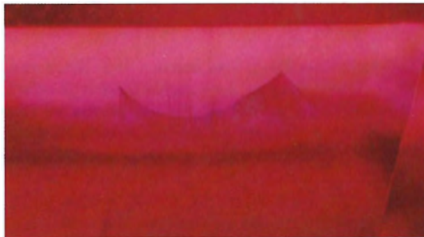
Figure 25. Curved and straight growth features associated with color zoning in a Ramaura synthetic ruby. Diffused and fiber-optic illumination, magnified 30x.
