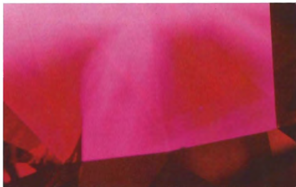
Figure 23. Prominent color zoning is revealed in this Ramaura synthetic ruby by placing a diffuser over dark-field illumination. Magnified 15 \times .
