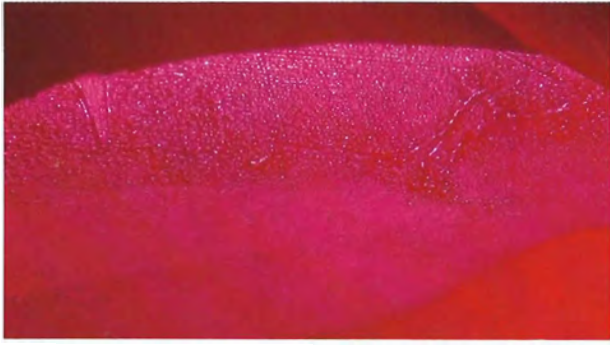
Figure 12. Healing fracture filled with white flux forming a flux "fingerprint" composed of a combination of tiny, closely arranged droplets and more loosely arranged mesh-like patterns. Dark-field and oblique illumination, magnified 32 \times .
