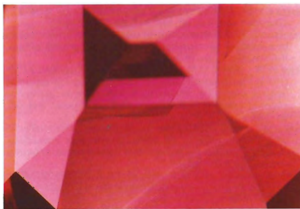
Figure 26. Diffused illumination accentuates different forms of color zoning and growth features in this Ramaura synthetic ruby. Magnified 15x.
