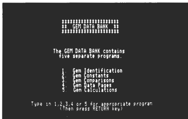
Figure 2. After the master program is loaded into the computer from the disk, a choice of five separate program sections is displayed on the monitor screen.
