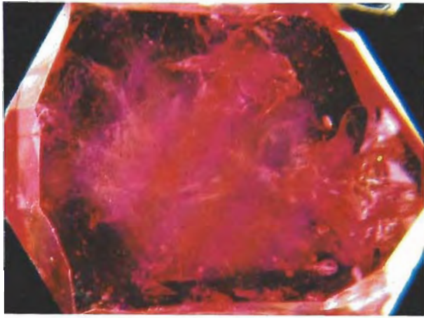
Figure 4. Integral picture of the interior of a cut synthetic \text{Al}_2\text{O}_3 ruby with cloudy veils. Magnified 10 \times .
