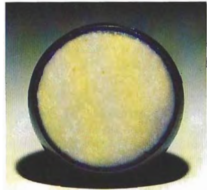
Figure 12. Cross-section of bead in figure 11 shows depth of dye penetration.
