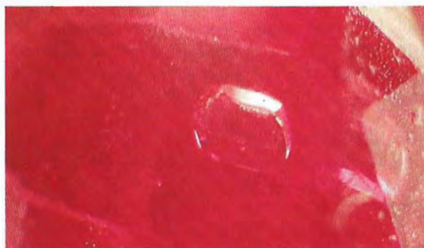
Figure 22. Distinctly shaped, hexagonal crystal of apatite in a Hunza Valley ruby. Magnified 20 \times .
