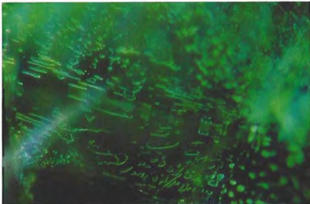
Figure 13. Partially healed fracture with tell-tale pattern of pseudosecondary liquid inclusions. Magnified 40×.
