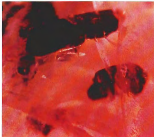
Figure 21. Flakes of phlogopite and an angular crystal of pyrite are indicative of rubies from the Hunza Valley. Magnified 20 \times .
